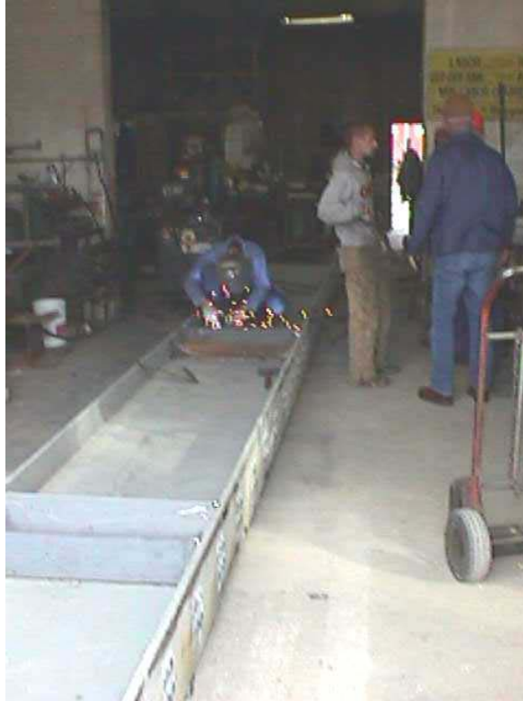
Figure 4.7. Manufacturing the steel girders.
