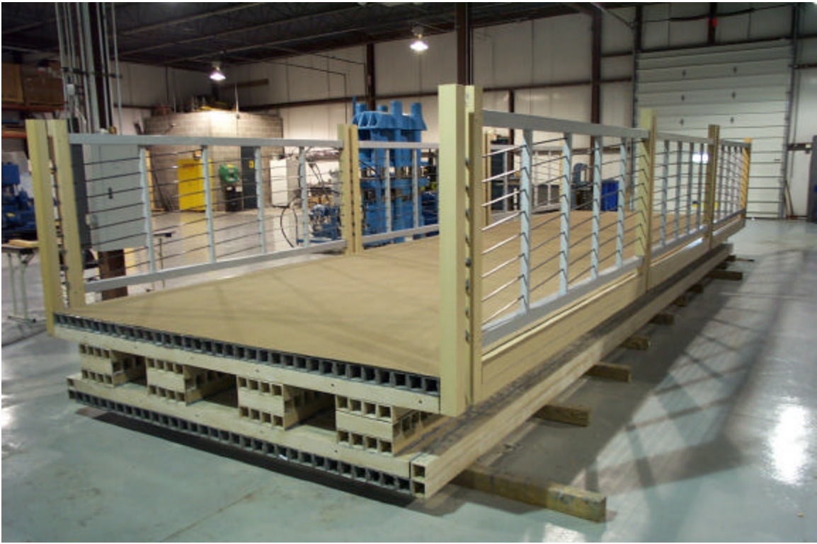
Assembled Smart Composite Bridge
