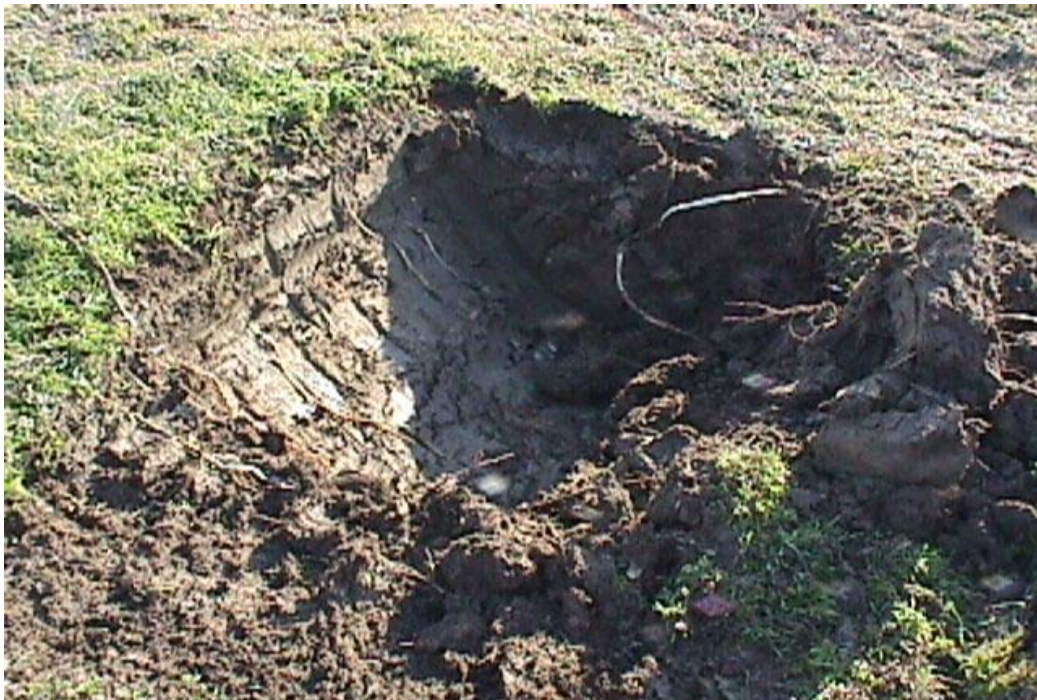
Figure 6. Sampling Trench for Clayey Soil at MM 17
