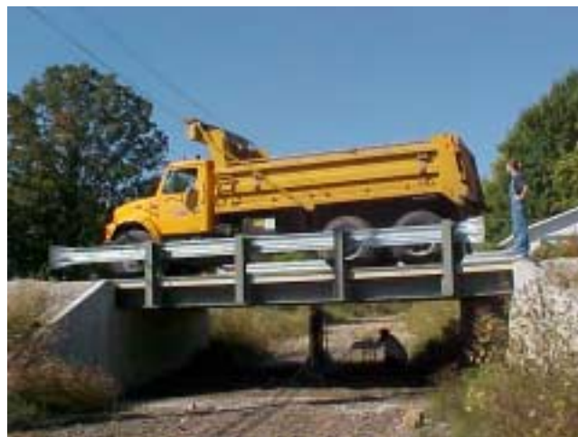
Figure 7.15 In-situ Bridge Load Test – Jay Street
