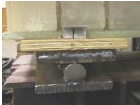
Figure 5.2 Specimen Support Detail
