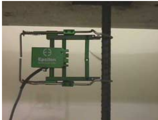
Figure 6.1 Extensometer Utilized During Tensile Testing
