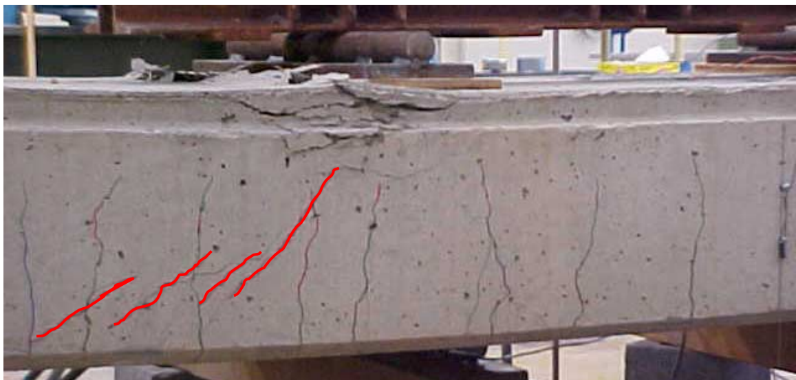
Figure 6.10 Failure of the FRP-RC Panel During Flexural Testing
