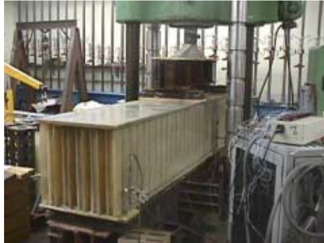
Figure 5.3 Flexural Test Setup – SF-2-1 and SF-2-2
