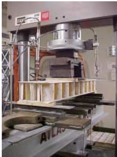
Figure 5.9 Test Setup for the Small-Scale Beam GFRP Sandwich Panel Specimens
