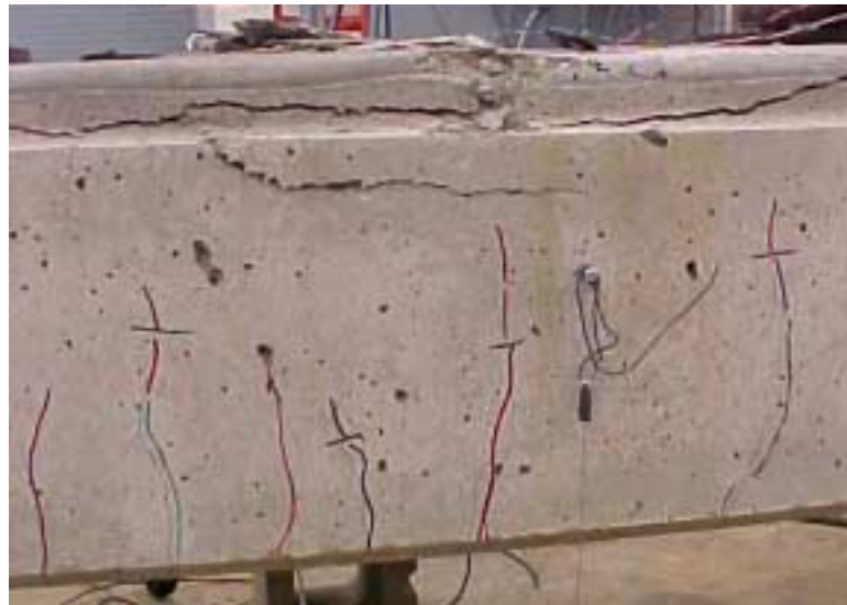
Figure 6.9 Failure of the Steel-RC Panel During the Flexural Testing
