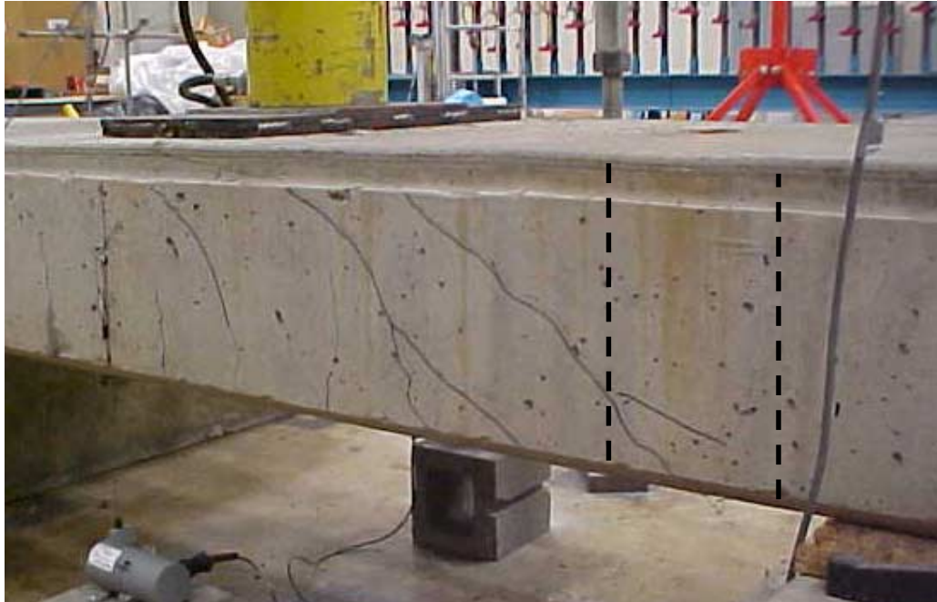
Figure 6.17 Shear Failure of the FRP-RC Panel
