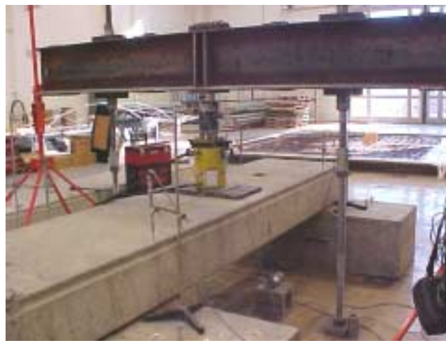
Figure 6.14 Test Setup for Shear Testing
