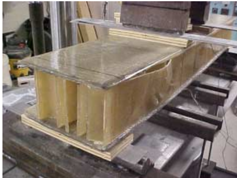
Figure 5.11 Failure Mode of the Small-Scale GFRP Sandwich Panel Specimens
