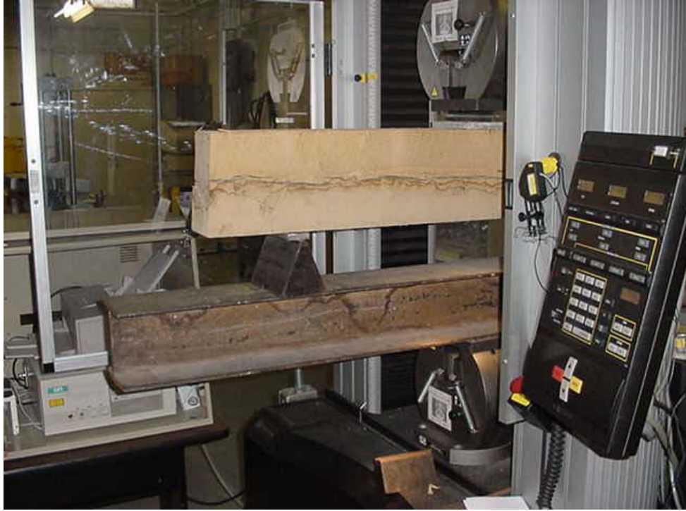
Figure 10: Three point bend test of 4" x 8" x 40" wooden beam.
