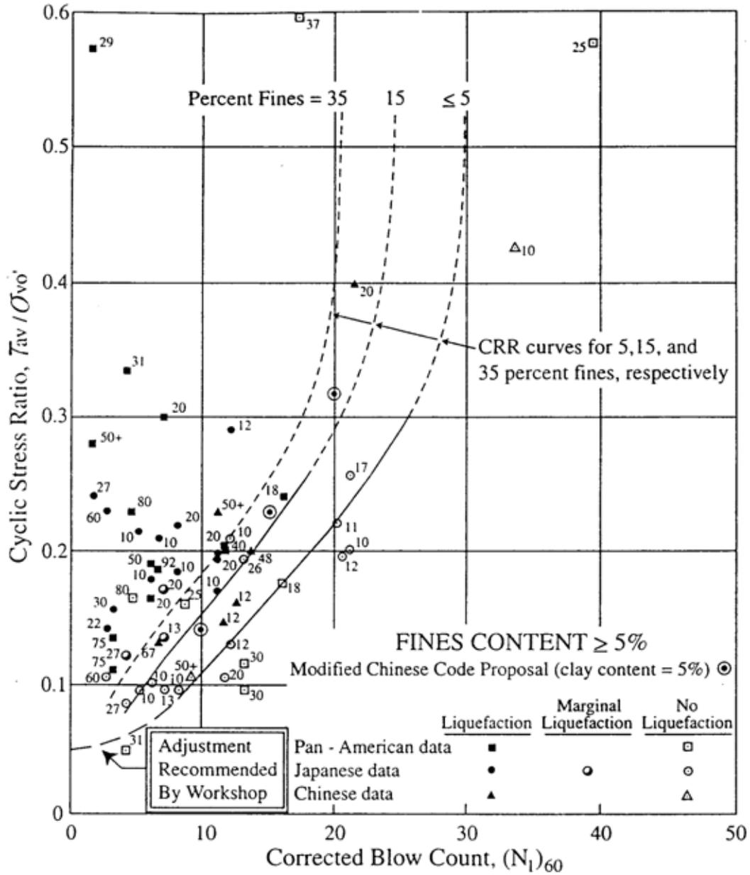
**Figure 5.4** Simplified Base Curve Recommended for Calculation of CRR From SPT  $(N_1)_{60}$  Data Along With Empirical Liquefaction Data for  $M=7.5$  (Seed et. al., 1971, modified by Youd and Idriss, 1997)
