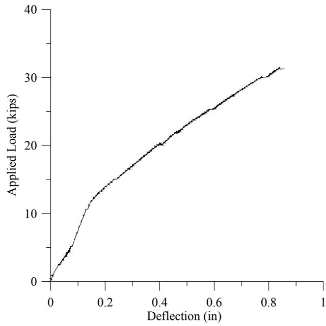
**Figure 6-20: Load Deflection Graph for 2 NSM**
