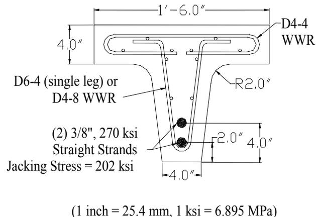
**Figure 3-1: Girder Cross-Section**
