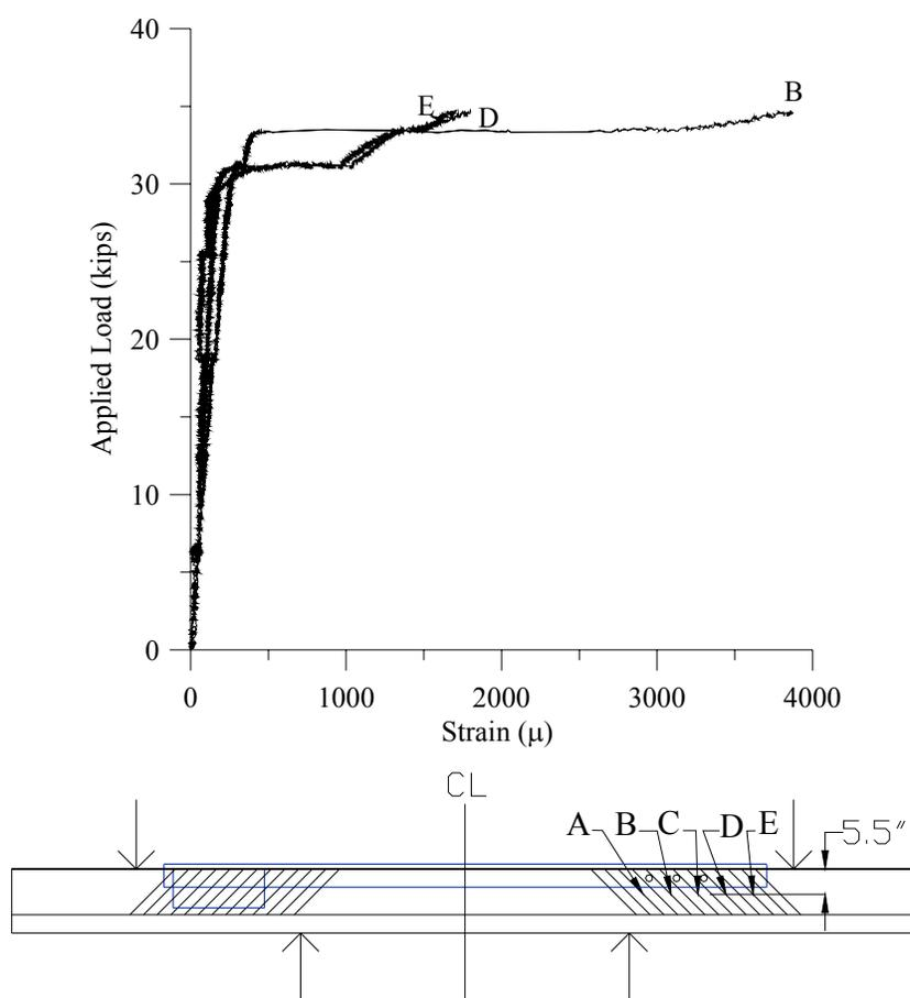
**Figure 6-12: Shear NSM Strain Graph for 1-NSM**
