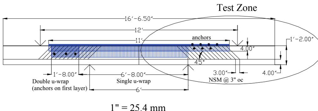
Figure 4-8: 2-NSM Strengthening
