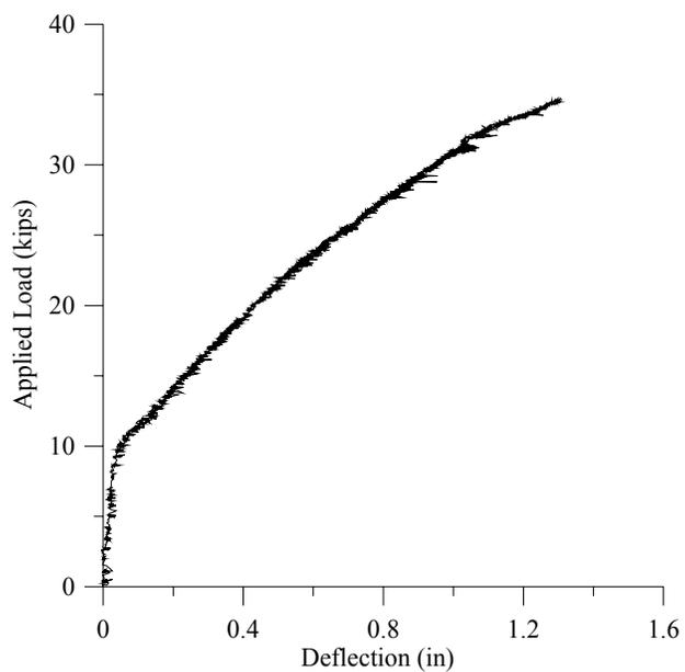
**Figure 6-13: Load Deflection Graph for 1-NSM**
