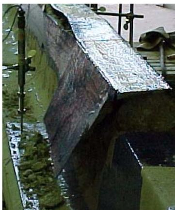
**Figure 6-15: 2-Sufficient FRP Debonding Failure**
