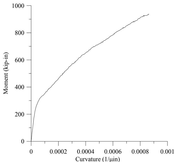
**Figure 6-6: Experimental Moment-Curvature Relationship for 1-Sufficient**
