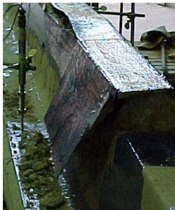
**Figure 6-15: 2-Sufficient FRP Debonding Failure**
