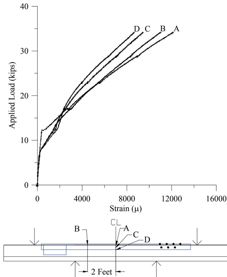
**Figure 6-16: Flexural FRP Strain Readings for 2-Sufficient**
