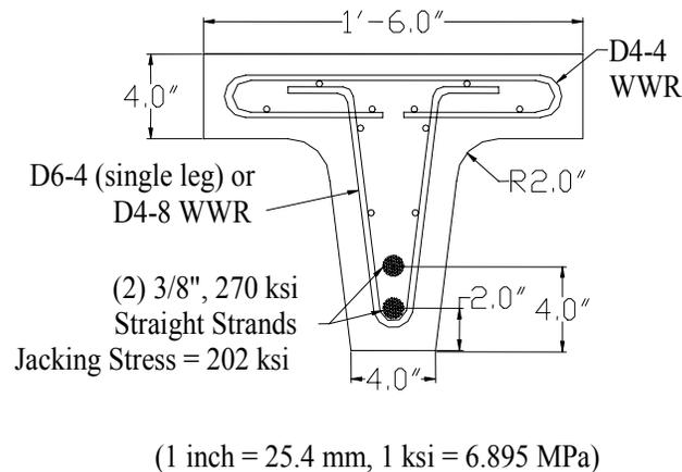
**Figure 3-1: Girder Cross-Section**
