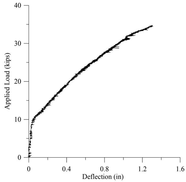
**Figure 6-13: Load Deflection Graph for 1-NSM**
