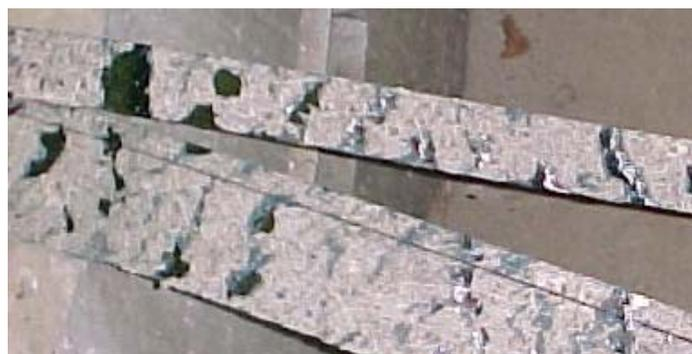
**Figure 6-3: Existing Defects on Flexural FRP of 1-Sufficient**
