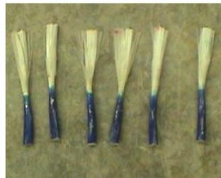
**Figure 3-2: GFRP Anchors**
