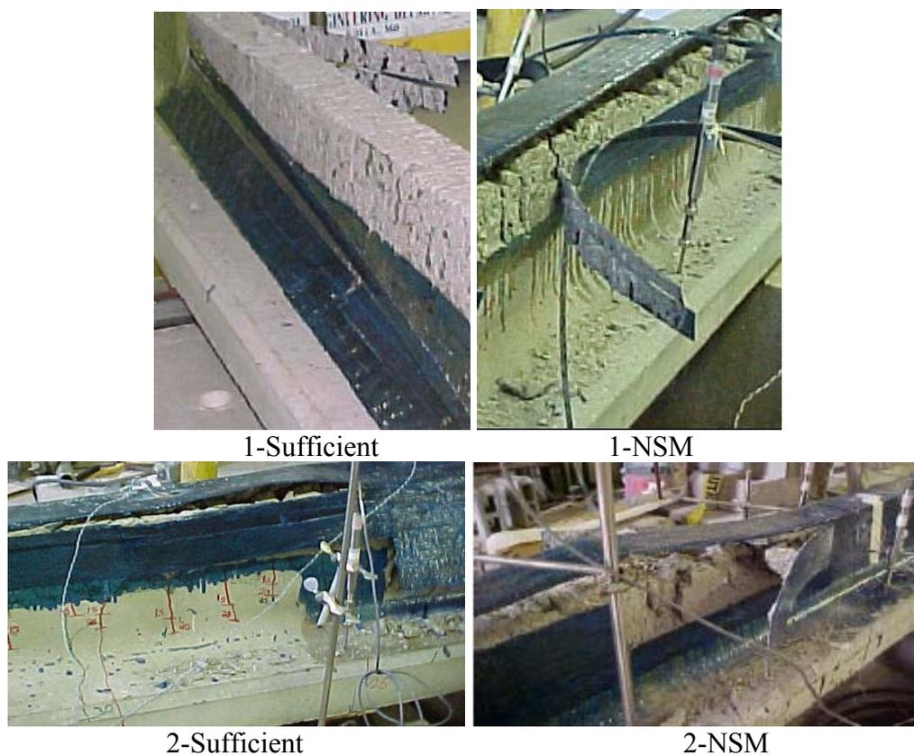
**Figure 6-2: FRP Debonding Failure in Four Girders**
