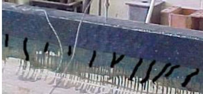
**Figure 6-4: 1-Sufficient Shear Cracks**
