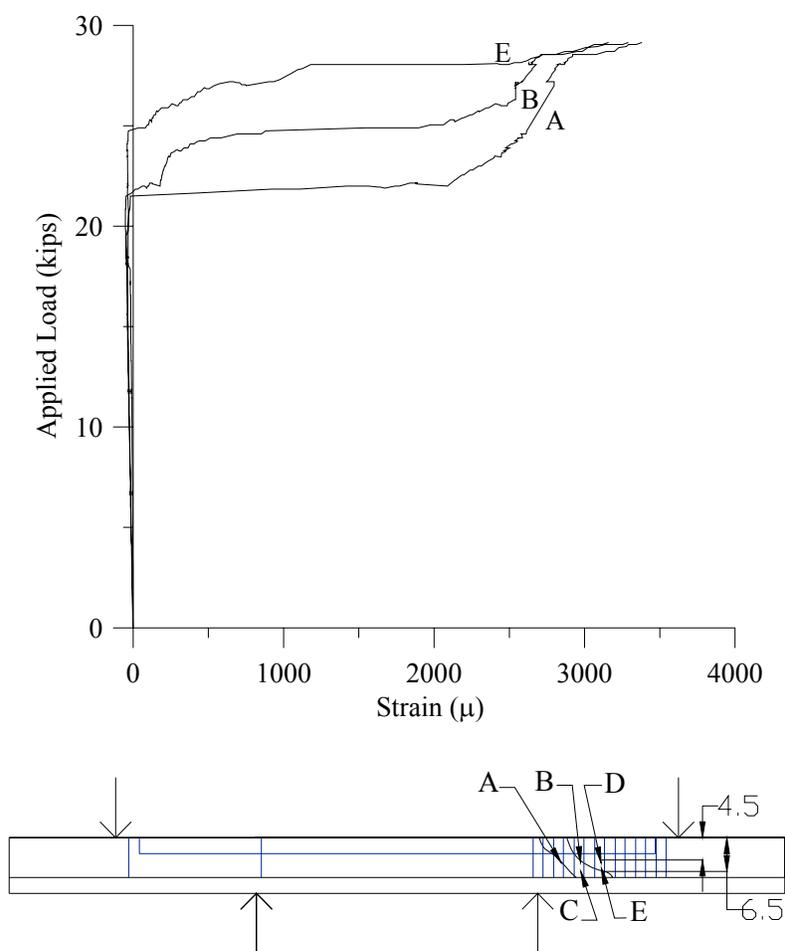
**Figure 6-8: Shear U-Wrap Strain Graph for 1-UW**
