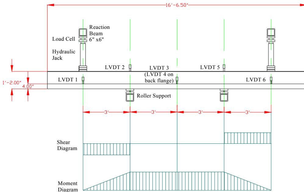
Figure 4-12: Schematic Test Set-Up and Shear and Moment Diagrams
