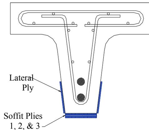
**Figure 4-1: Flexural Strengthening**
