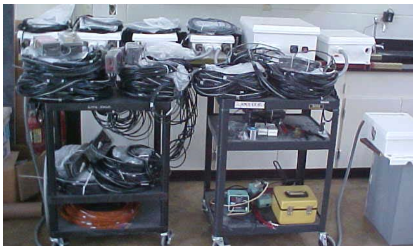
Figure 3.28. DAS and Gauges Ready for the Instrumentation
