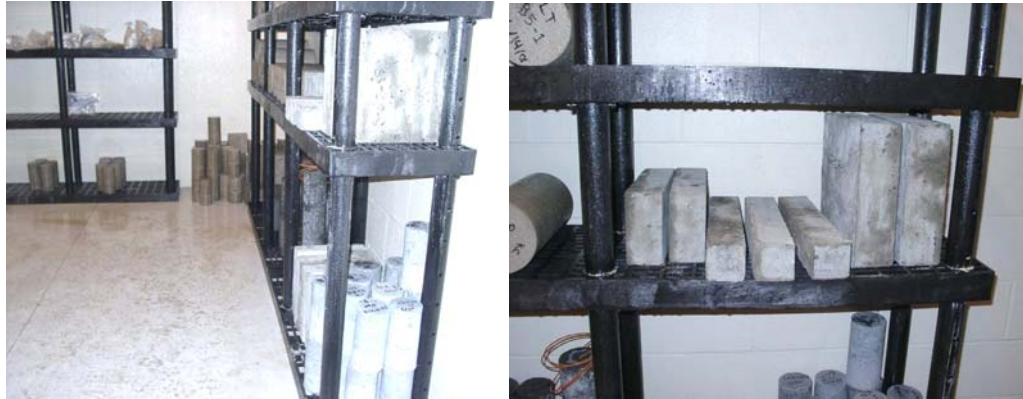
Figure 2.3. ASTM Moist Curing Room
