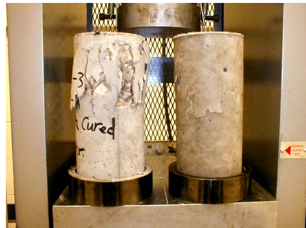
Figure 2.8. Compressive Strength and Elastic Modulus Test at UMR
