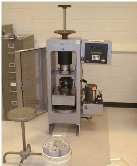
Figure 2.8. Compressive Strength and Elastic Modulus Test at UMR
