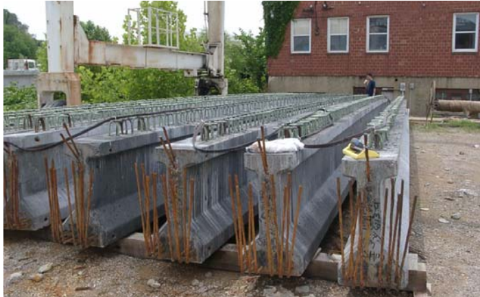
Figure 9.6. Girders Storage at Precast Plant
