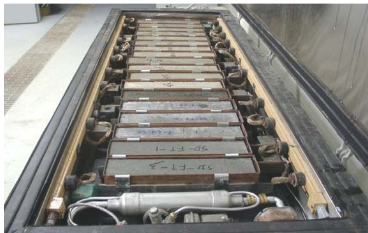
Figure 2.15. F-T Test Machine
