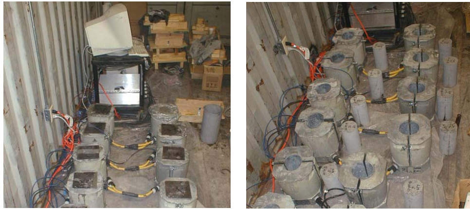
Figure 2.5. Match Curing System and Specimens
