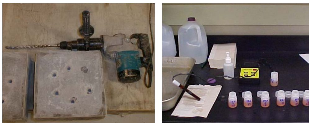
Figure 2.17. Ponding Chloride Test
