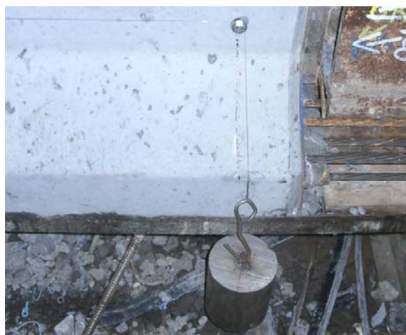
Figure 3.11. Dead Weight for Tension-Wire System
