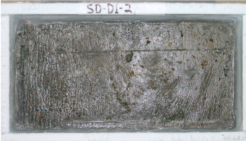
Figure 2.18. Scaling Resistance Test Specimen
