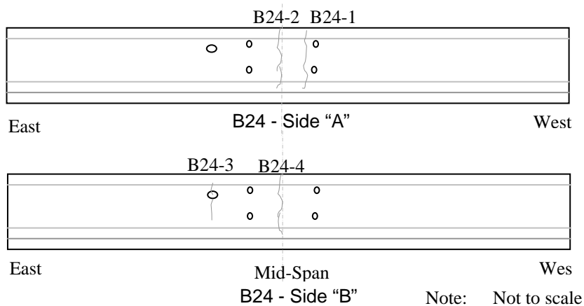
Figure 6.11. Cracking Observed in Girder B24 Prior to Release
