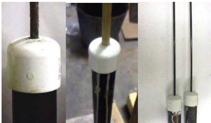
Figure 17: PVC drilled caps used for alignment
