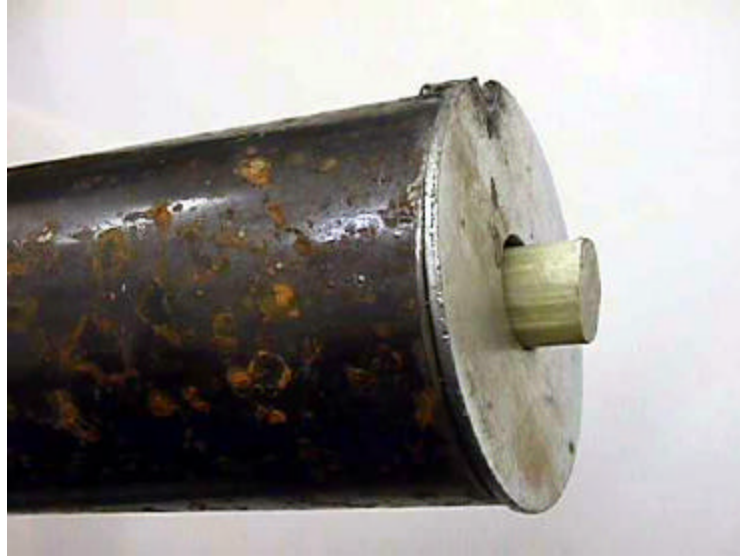
Figure 15: Washer welded for alignment of the rod
