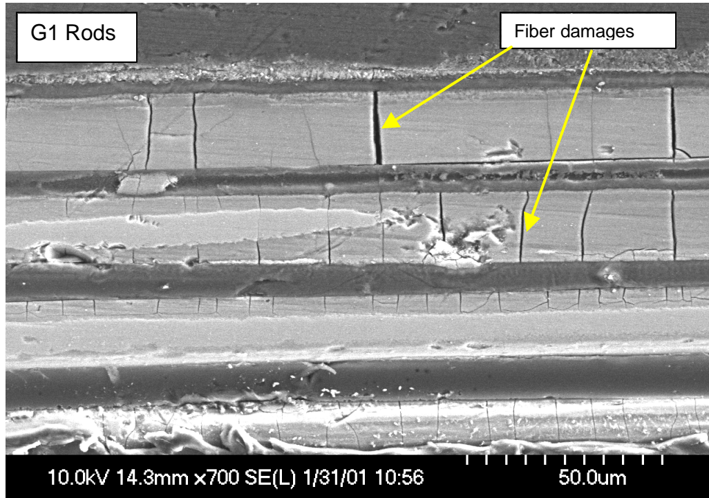
Figure 46: SEM longitudinal section of G1 specimens
