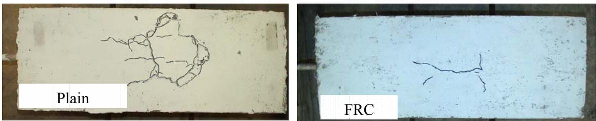
(c) Crack patterns of #4 GFRP with 1  $d_b$  cover in plain concrete and FRC
