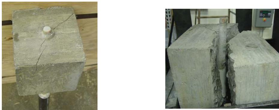
**Figure 4.10. Failure for FRC and Plain Concrete Specimens**
