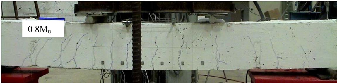
(a) VF4C (FRC Beams)
