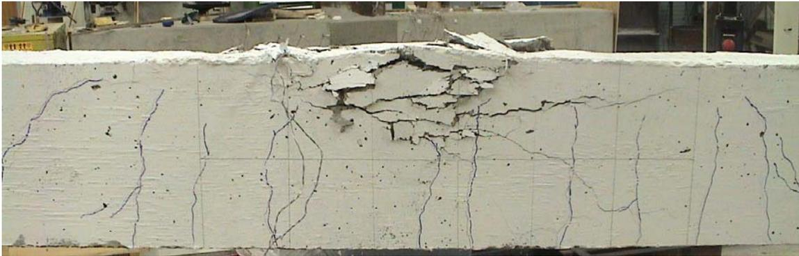
**Figure 5.18. Typical Failure Mode**
