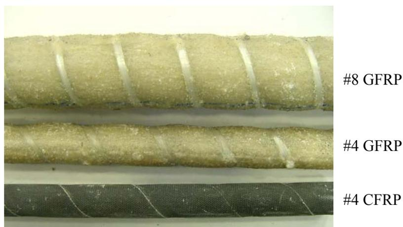
**Figure 3.12. FRP Rods Used in this Study**
