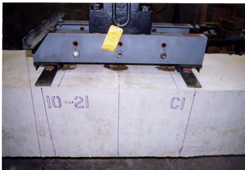
Figure 5.12. Close-up of spreader beam used for loading
