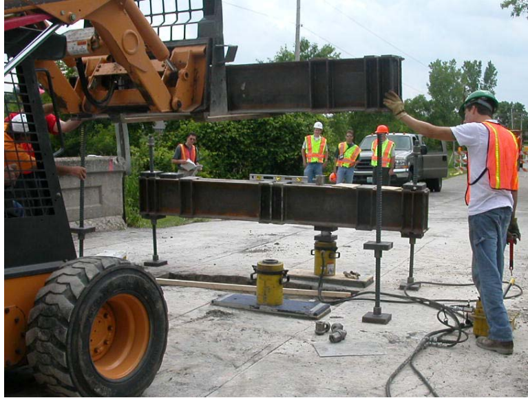
Figure 6.9. Placing the north reaction beam
