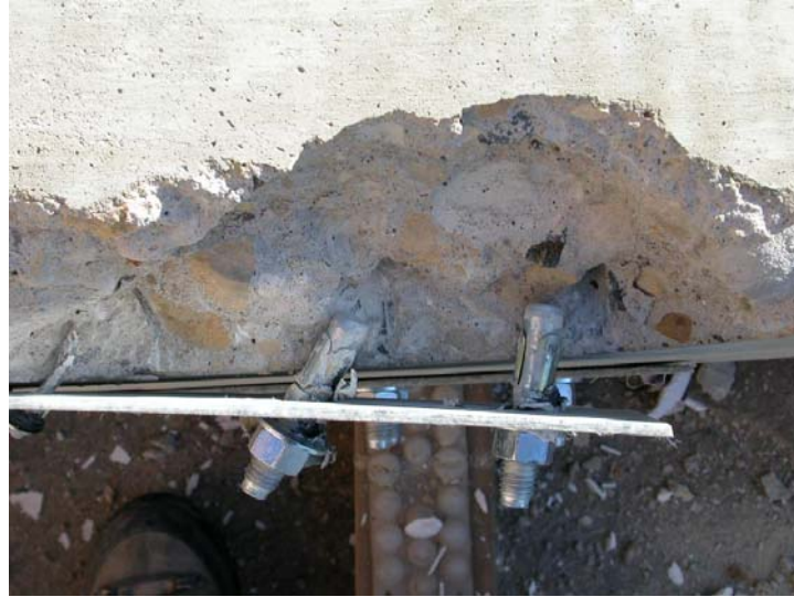
Figure 5.49. Final end-anchor pullout failure in beam FRP 3
