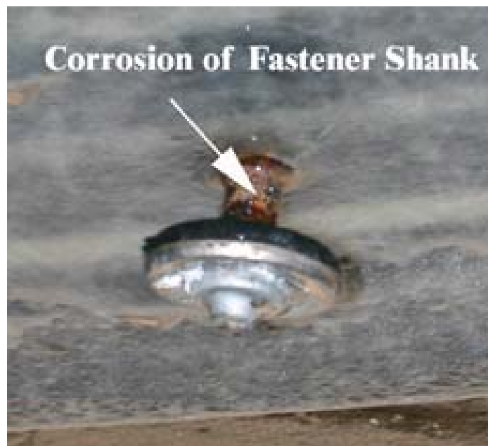
Figure 6.42. Corrosion of ALH fastener shank with incomplete embedment
