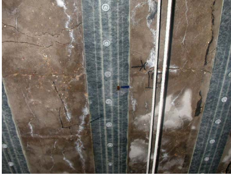
Figure 6.20. Flexural cracks at midspan of west section (during test)
