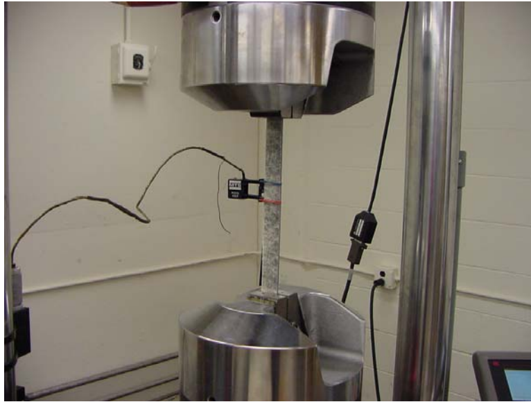
Figure 6.46. Testing a coupon of recovered material (no hole)
