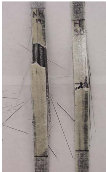
Figure 6.47. Failed coupons of virgin material (left – no hole; right – central hole)
