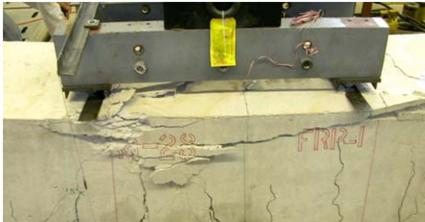
Figure 5.22. Concrete compression failure of FRP1
