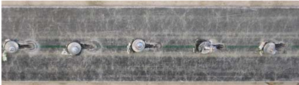
Figure 5.51. Bearing failure mode in FRP strip in beam FRP 3
