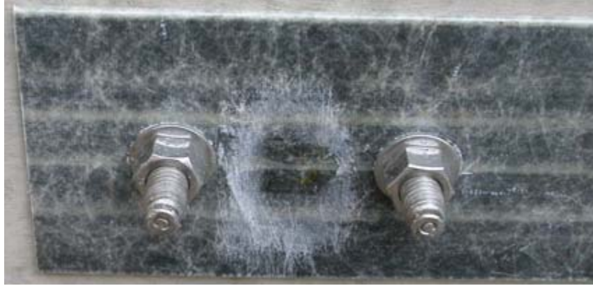
Figure 5.33. FRP strip at the end for beam FRP 2SS (post failure)
