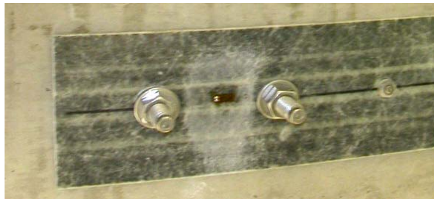
Figure 5.7. End anchor bolts and end fastener for FRP2 SS
