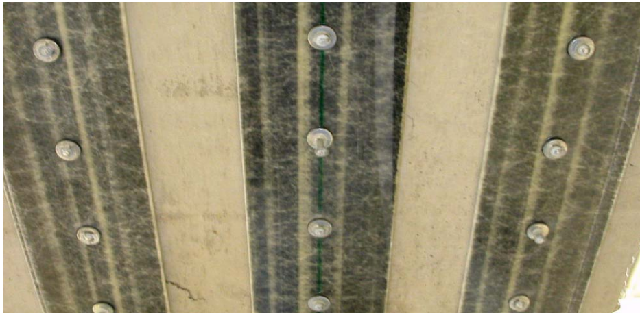
Figure 5.8. FRP 3 beam strengthened with three FRP strips
