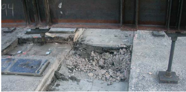
Figure 6.18. Concrete crushing failure along top of west section
