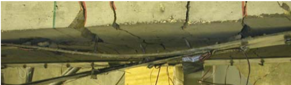
Figure 5.35. Horizontal splitting of the FRP strip in FRP 2SS
