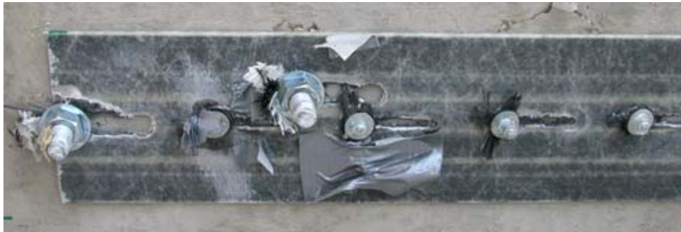
Figure 5.25. Bearing failure at the end of an FRP strip in beam FRP 1
