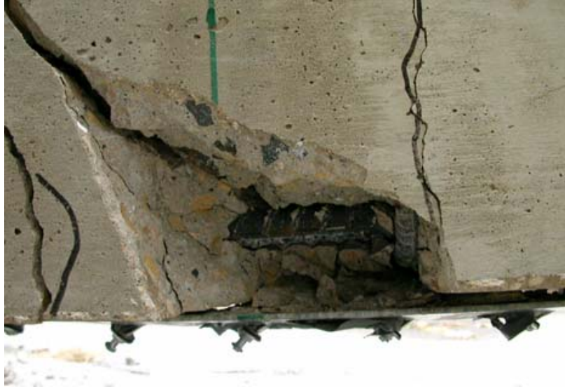
Figure 5.26. Secondary failure mode of beam FRP 1 due to fastener pullout
