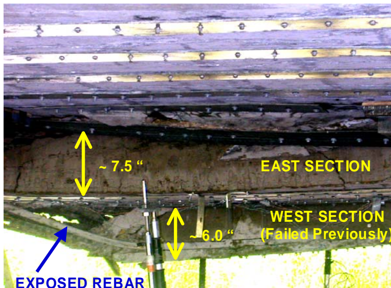
Figure 6.22. Concrete crushing along top of east section
