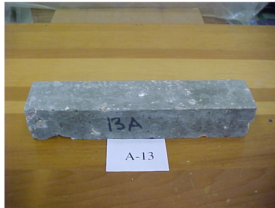
Figure B.7. Control sample of HSC with 0.30 w/c, after 300 freezing & thawing cycles (0 air entrainment)
