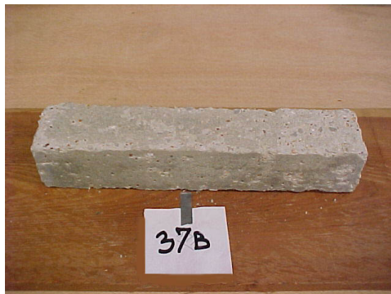
Figure B.25. Control sample of Limestone utilized HPC with 0.45 w/c ratio, after 300 freezing & thawing cycles
