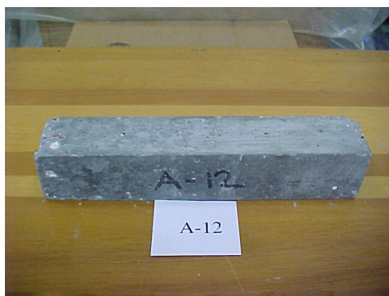
Figure B.6. 25% FA+5% GGBS substituted sample of HSC with 0.25 w/c, after 300 freezing & thawing cycles (3% entrained air)
