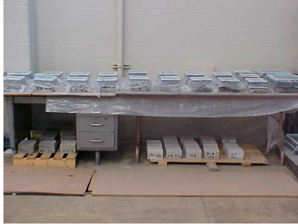
Figure 3.2. Concrete samples exposed to chloride solution
