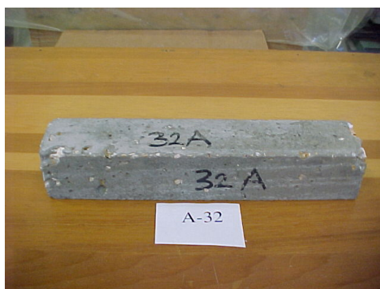
Figure B.17. 30% FA substituted sample of HSC with 0.35 w/c ratio, after 300 freezing & thawing cycles (3.5% air entrainment)
