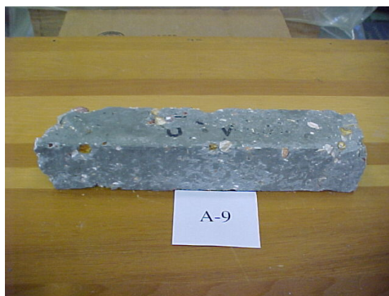
Figure B.5. 25% FA+5% GGBS substituted sample of HSC with 0.25 w/c, after 300 freezing & thawing cycles (0 entrained air)
