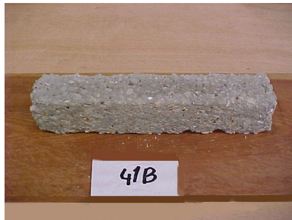
Figure B.29. 30% FA substituted sample of Limestone utilized HPC with 0.40 w/c ratio, after 300 freezing & thawing cycles
