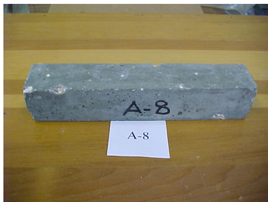
Figure B.4. 30% FA substituted sample of HSC with 0.25 w/c, after 300 freezing & thawing cycles (3% entrained air)
