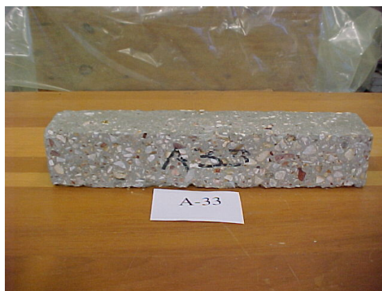
Figure B.18. 25% FA+5% GGBS sample of HSC with 0.35 w/c after 300 freezing & thawing cycles (0 air entrainment)
