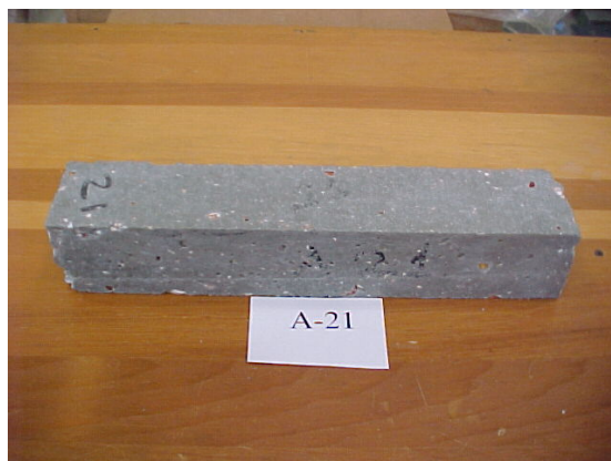
Figure B.11. 25% FA+5% GGBS substituted sample of HSC with 0.30 w/c ratio, after 300 freezing & thawing cycles (0 air entrainment)
