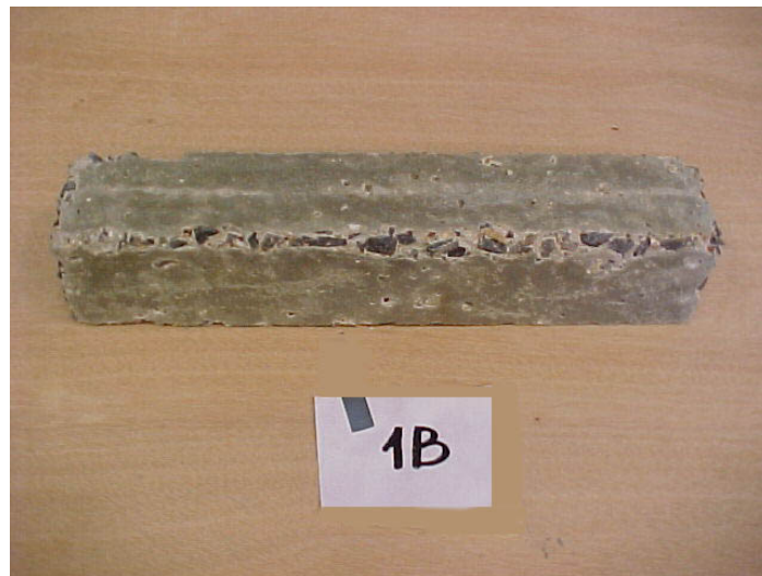
Figure 4.35. River Gravel used control mixture with 0.45 w/c ratio, after 300 freezing & thawing cycles
