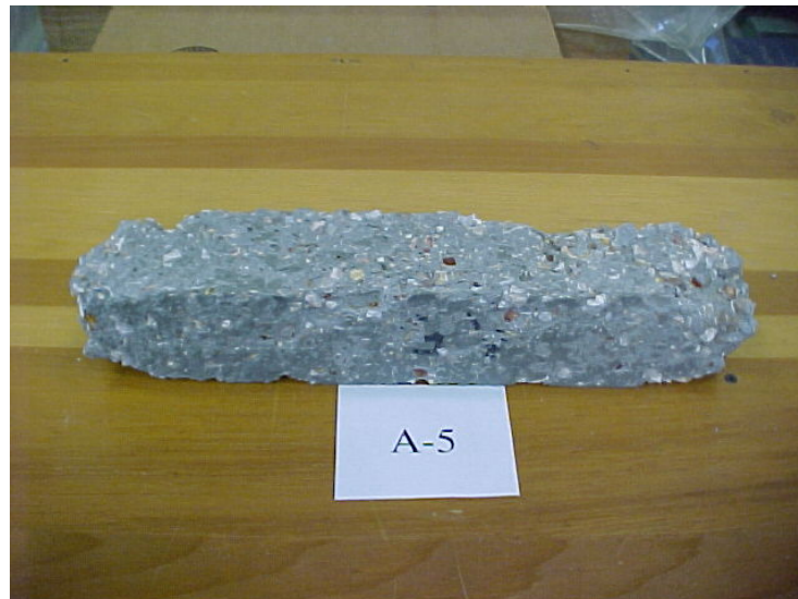
Figure 4.7. 30% fly ash substituted mixture with 0.25 w/c ratio, 0% air entrainment, after 300 freezing & thawing cycles
