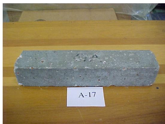
Figure B.9. 30% FA substituted sample of HSC with 0.30 w/c ratio, after 300 freezing & thawing cycles (0 air entrainment)
