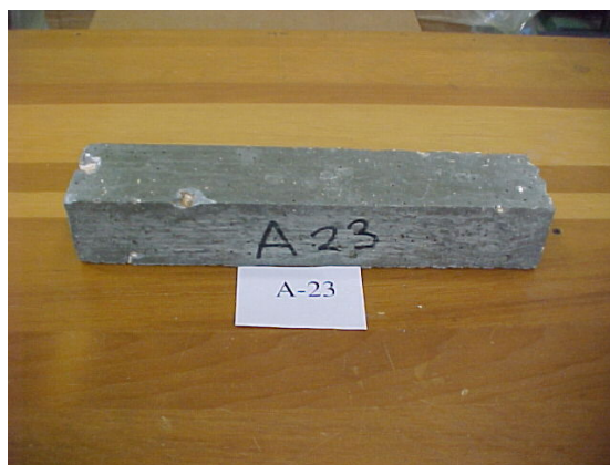
Figure B.12. 25% FA+5% GGBS substituted sample of HSC with 0.30 w/c ratio, after 300 freezing & thawing cycles (1% air entrainment)
