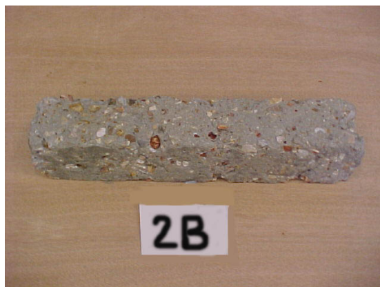
Figure B.20. Control sample of Trap Rock utilized HPC with 0.45 w/c ratio, after 300 freezing & thawing cycles
