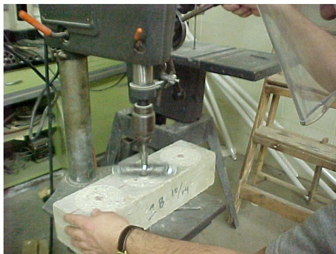
Figure 3.5. Abrasion test by rotating-cutter method
