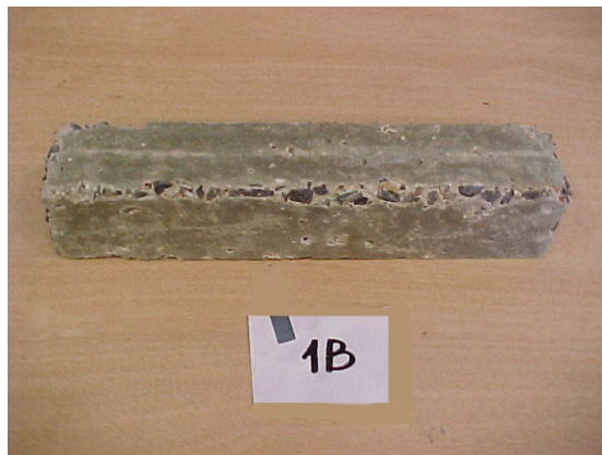
Figure B.19. Control sample of River Gravel utilized HPC with 0.45 w/c ratio, after 300 freezing & thawing cycles
