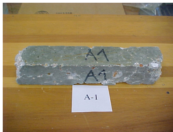
Figure B.1. Control sample of HSC with 0.25 w/c, after 300 freezing & thawing cycles (0 entrained air)
