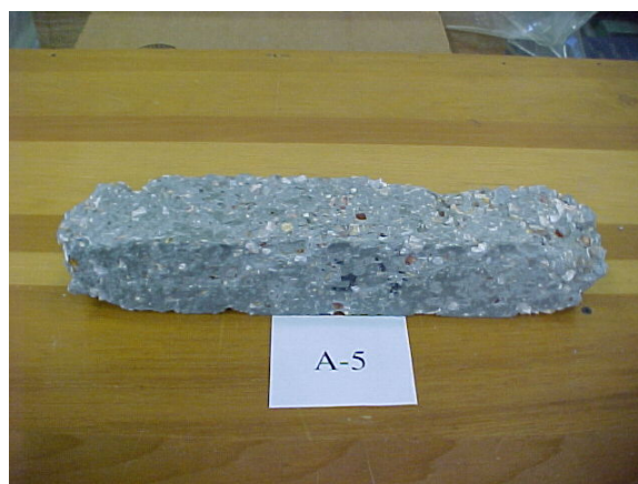
Figure B.3. 30% FA substituted sample of HSC with 0.25 w/c, after 300 freezing & thawing cycles (0 entrained air)
