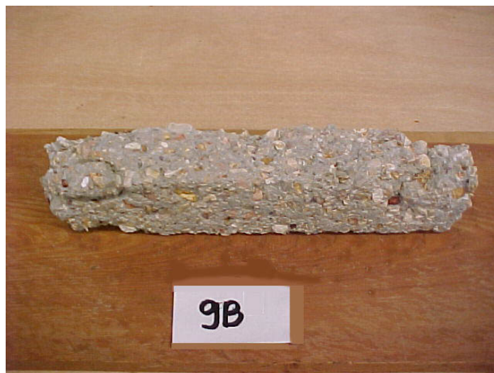
Figure 4.36. 30% fly ash substituted, River Gravel used mixture with 0.40 w/c ratio, after 300 freezing & thawing cycles
