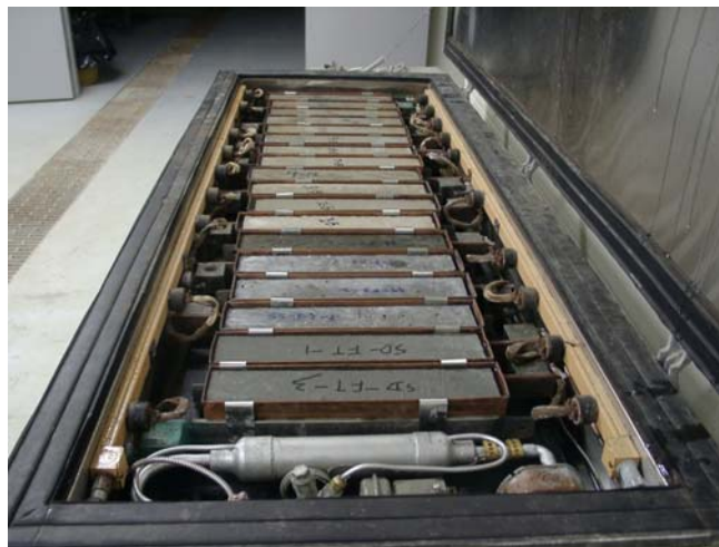
Figure 3.8 Freezing & thawing test set-up
