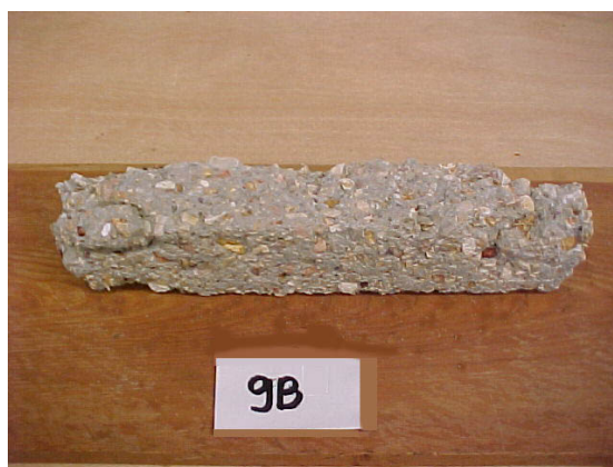
Figure B.24. 30% FA substituted sample of River Gravel utilized HPC with 0.40 w/c, after 300 freezing & thawing cycles
