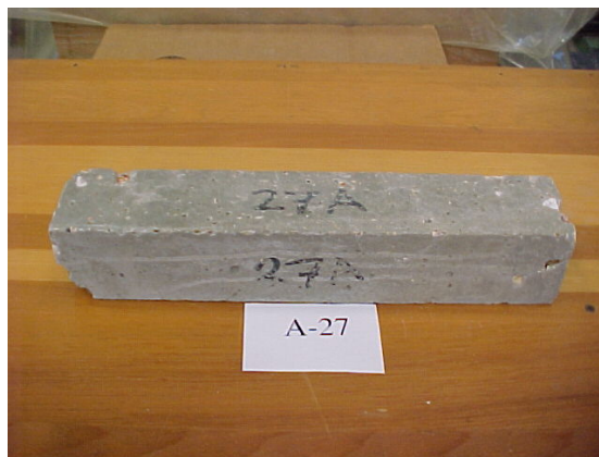
Figure B.15. Control sample of HSC with 0.35 w/c ratio, after 300 freezing & thawing cycles (3.5 air entrainment)
