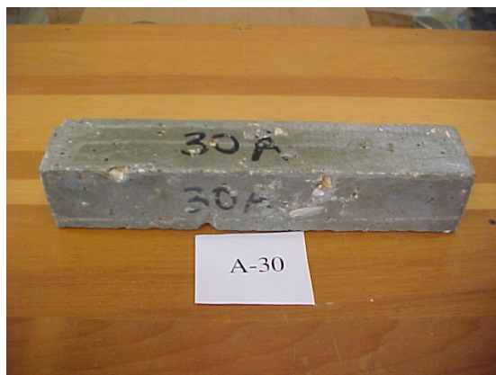
Figure B.16. 30% FA substituted sample of HSC with 0.35 w/c ratio, after 300 freezing & thawing cycles (1.5% air entrainment)
