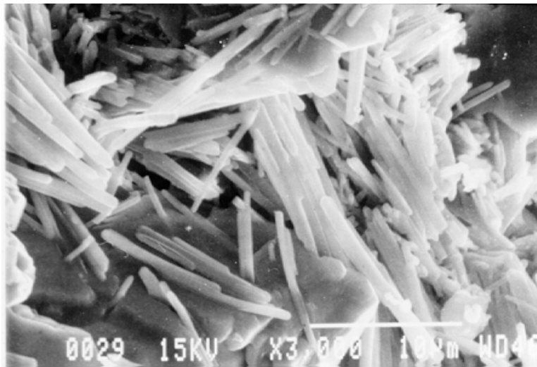
Figure 2.12: Ettringite growth under SEM examination at X3000 magnification [Myers, 1998]
