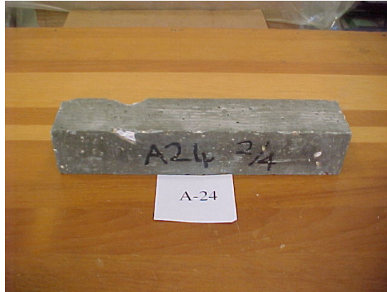
Figure B.13. 25% FA+5% GGBS substituted sample of HSC with 0.30 w/c ratio, after 300 freezing & thawing cycles (4.5% air entrainment)
