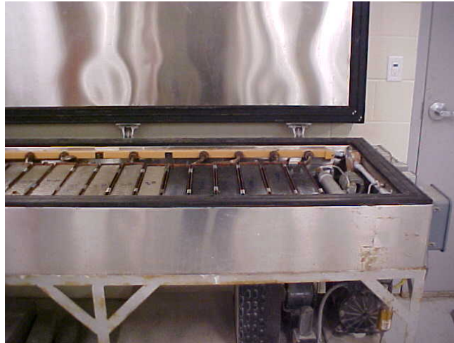
Figure 3.7 Freezing & thawing test set-up
