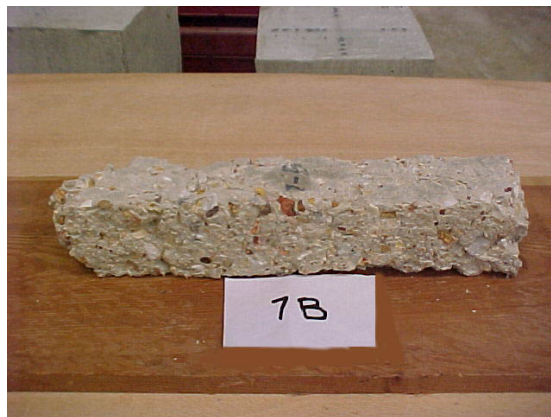
Figure B.22. Control sample of River Gravel utilized HPC with 0.40 w/c, after 300 freezing & thawing cycles
