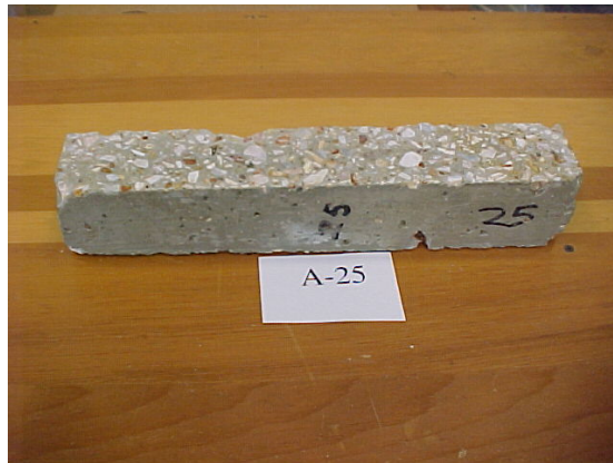
Figure B.14. Control sample of HSC with 0.35 w/c ratio, after 300 freezing & thawing cycles (0 air entrainment)
