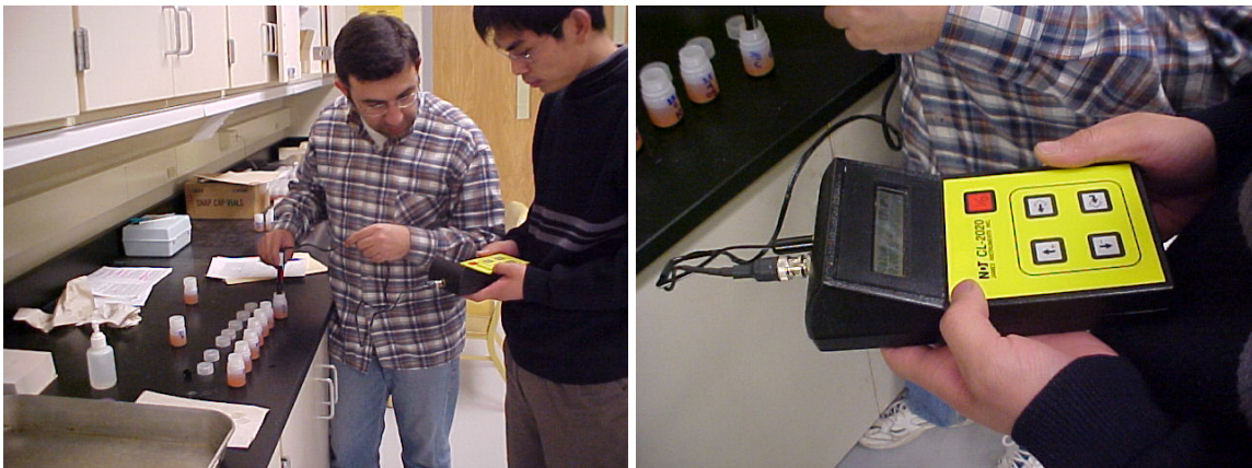
Figure 3.4. Chloride content (percent by weight) measurements
