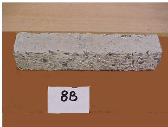
Figure B.23. Control sample of Trap Rock utilized HPC with 0.40 w/c ratio, after 300 freezing & thawing cycles
