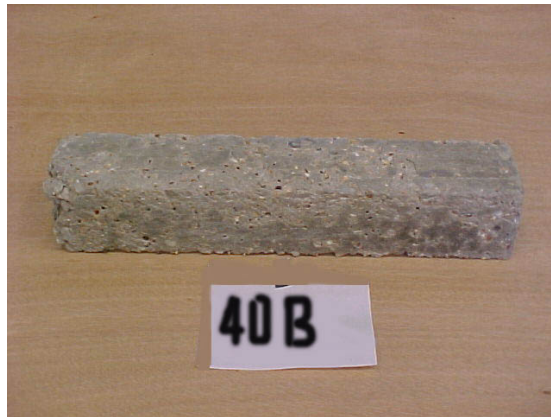
Figure B.28. Control sample of Limestone utilized HPC with 0.40 w/c ratio, after 300 freezing & thawing cycles
