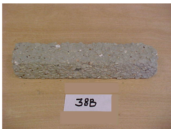
Figure B.26. 30% FA substituted sample of Limestone utilized HPC with 0.45 w/c ratio, after 300 freezing & thawing cycles
