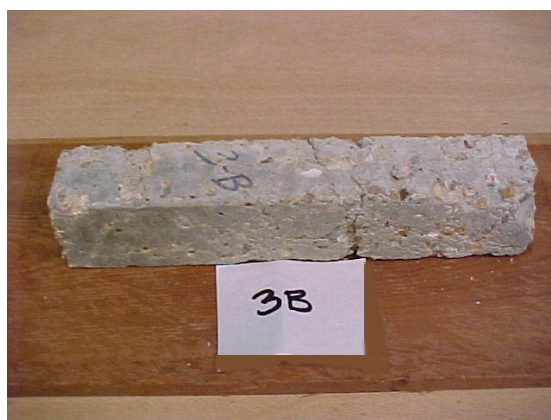
Figure B.21. 30% FA substituted sample of River Gravel utilized HPC with 0.45 w/c, after 300 freezing & thawing cycles
