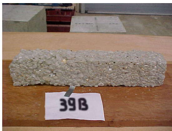
Figure B.27. 25% FA+5% GGBS substituted sample of Limestone utilized HPC with 0.45 w/c ratio, after 300 freezing & thawing cycles
