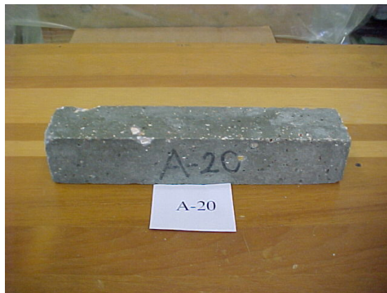
Figure B.10. 30% FA substituted sample of HSC with 0.30 w/c ratio, after 300 freezing & thawing cycles (1.5% air entrainment)
