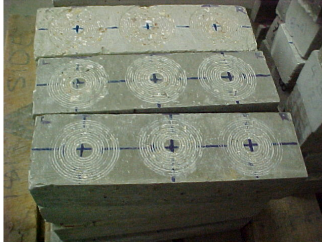
Figure 3.6. Concrete test samples after abrasion test
