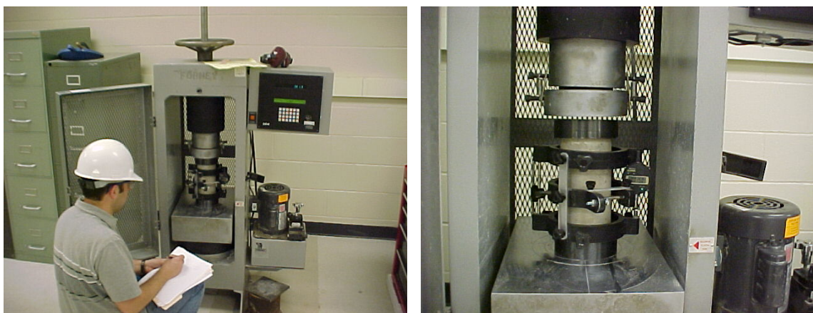
Figure 3.1. Uniaxial compression and MOE tests
