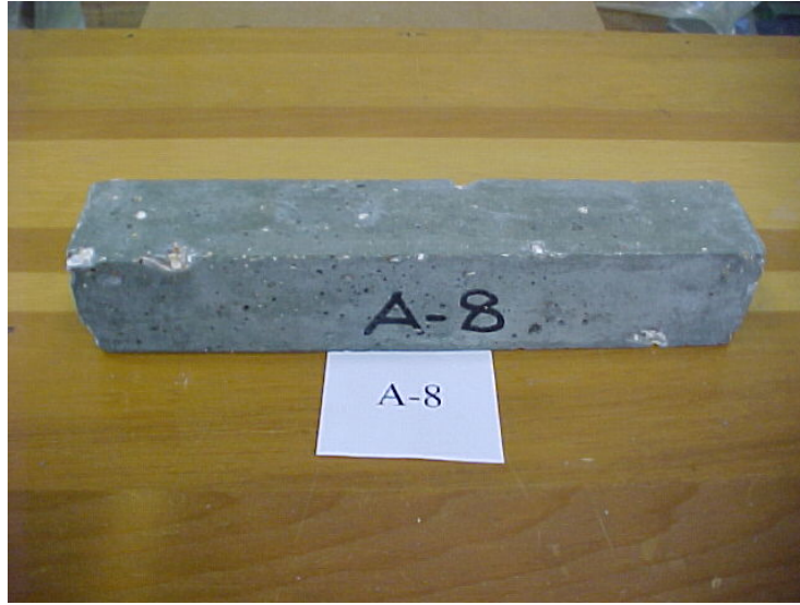
Figure 4.8. 30% fly ash substituted mixture with 0.25 w/c ratio, 4% air entrainment, after 300 freezing & thawing cycles
