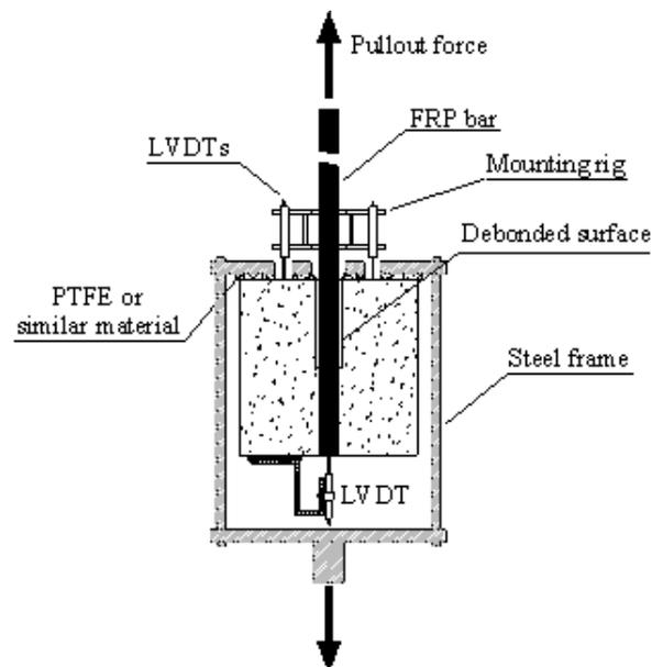
Figure 4: Pullout Test Assemble Sketch
