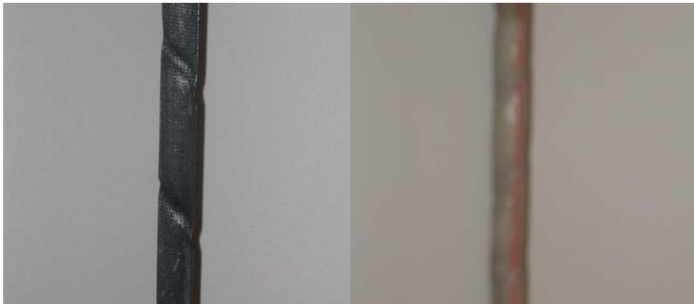
Figure 1: Surface of Carbon and Glass Rods
