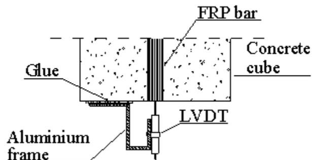
Figure 5: LVDT at the bottom face of the cube (vertical section)
