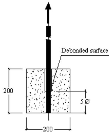
Figure 3: Pullout Test Sample
