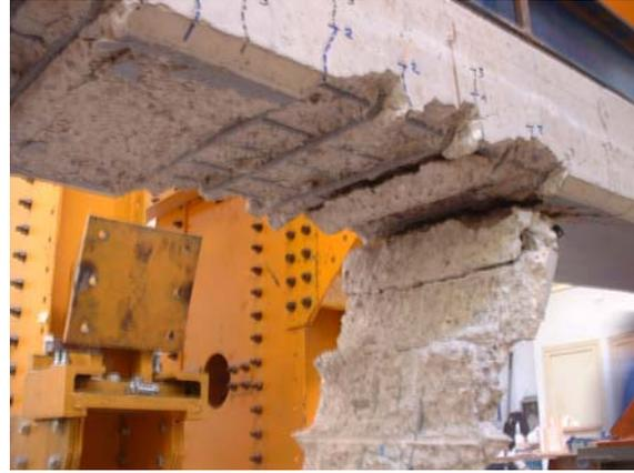
Figure 13 - Bottom View of Failure of A-2 Beam
