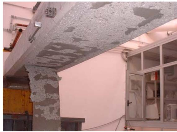
Figure 15 - Bottom View of Failure of B-2 Beam
