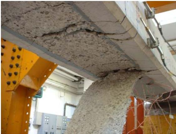
Figure 14 - Bottom View of Failure of B-1 Beam
