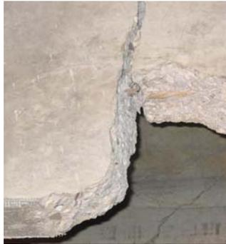
c) SRP Rupture    d) Rupture of the Lower Tendon
