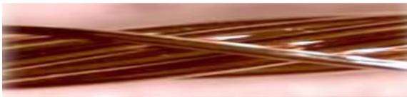
a) 12 Wires Wrapped by 1 Wire
