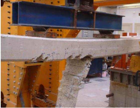
Figure 12 - Lateral View of Failure of A-2 Beam
