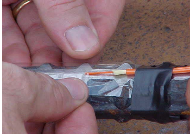
(a) Placing Mylar tape on sensor
