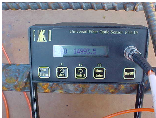
(c) Single channel data logger
