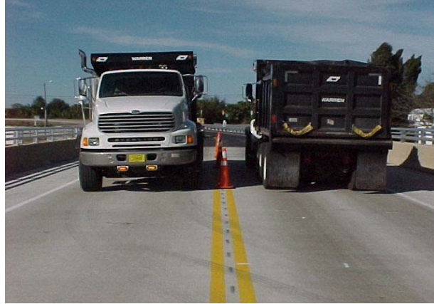
(a) Testing of bridge under SU4 trucks
