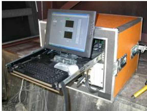
Figure 5 Data Acquisition System (“Orange Box”)
