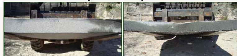
Reinforced concrete panel with plain polyurea B (left) and reinforced concrete panel with discrete fiber-reinforced polyurea B (right).
