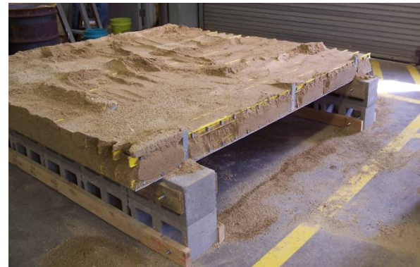
Figure 5 – Test set-up of gridform under uniform sand load
