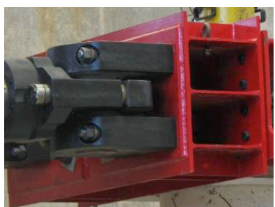
Photo of the Loading Beam Connected to Actuator and Specimen
