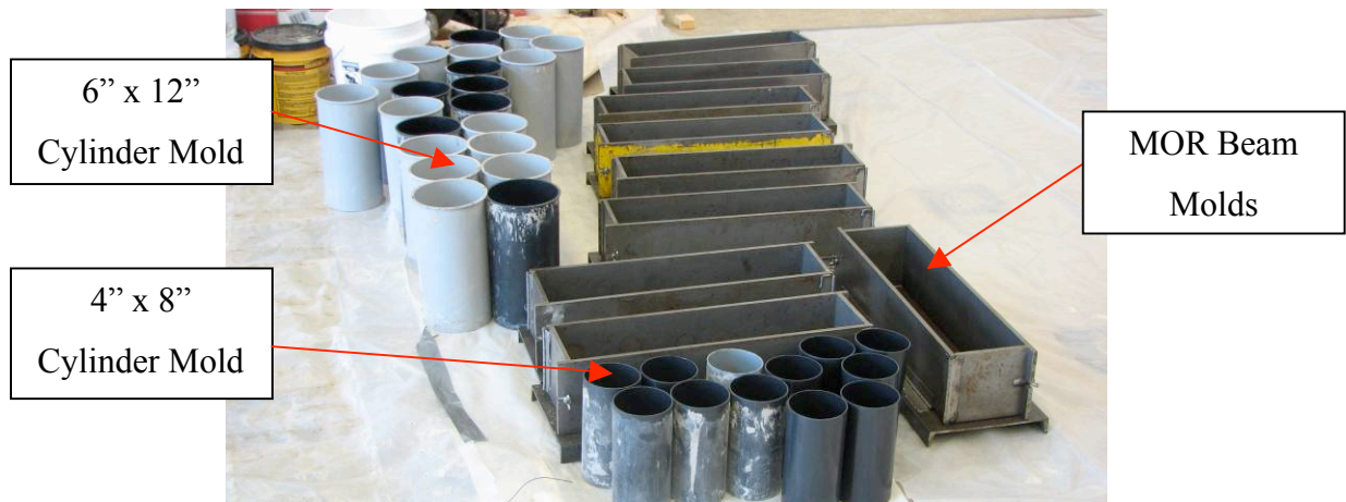
Figure 3.20 Auxiliary Specimens for Concrete Material Testing
