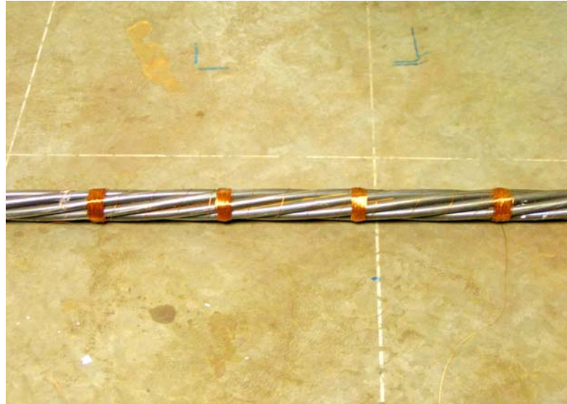
Figure 12: Prestressing strand with windings.
