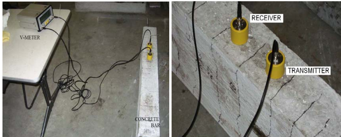
Figure 2: Photograph of a UPV system applied to a concrete beam in the laboratory.
