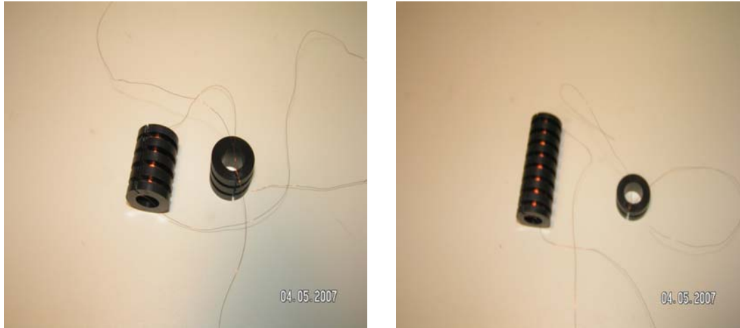
Figure 10: Pictures showing the 1-coil, 2-coil, 4-coil and 8-coil sensors with windings.
