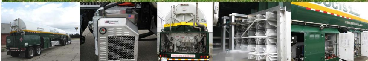
Liquid Hydrogen Tanker with onboard high pressure liquid pump and vaporizer
