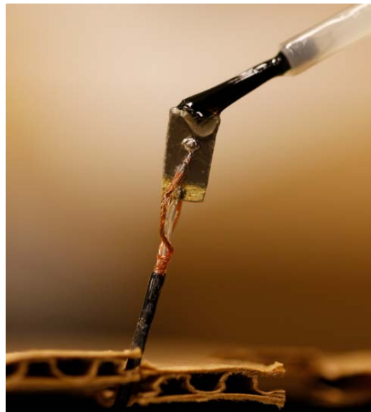
Fig. 7 Coating with polyurethane
