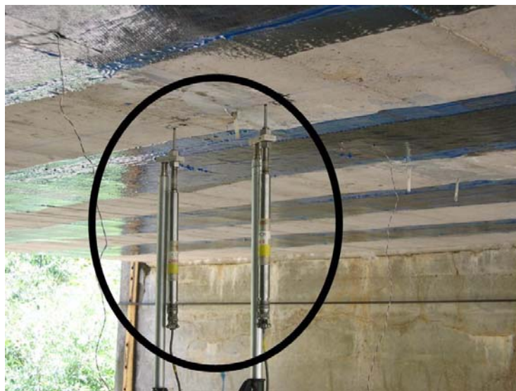
Figure 4.2. Two LVDT's Measuring Deflection
