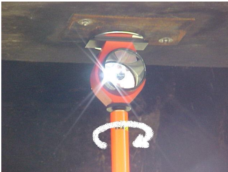
Figure C.5. Screw Range Pole onto Prism
