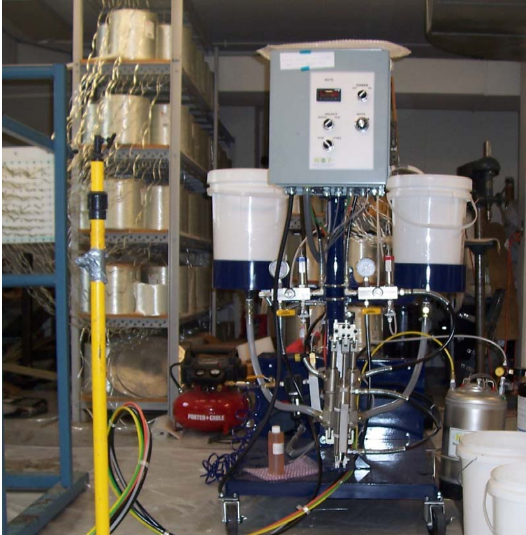
Figure 1. Metering unit setup for pultrusion process
