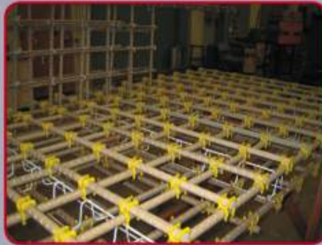
A steel free mock-up at the SERL High Bay Structures Lab.
