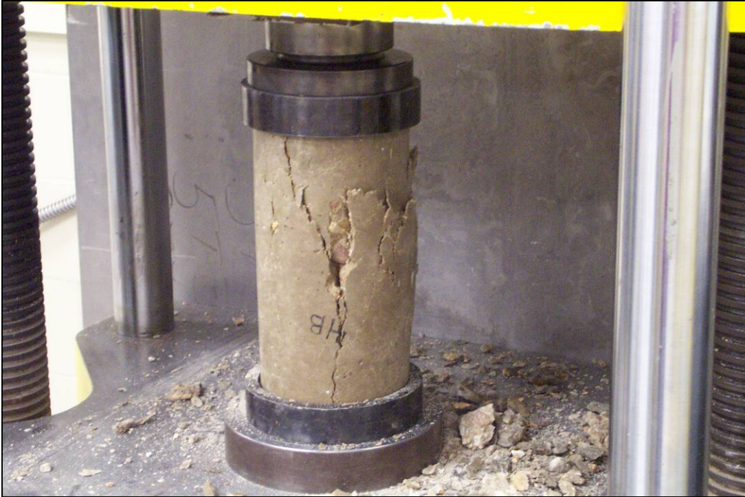
Figure 2: Compressive Strength Testing of Cylinders
