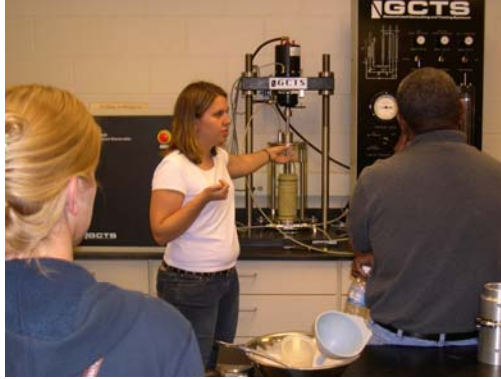
Graduate student Rachel Mudd demonstrating triaxial testing procedures.
