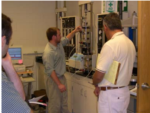
Graduate student Benjamin Gallagher demonstrating triaxial testing procedures.
