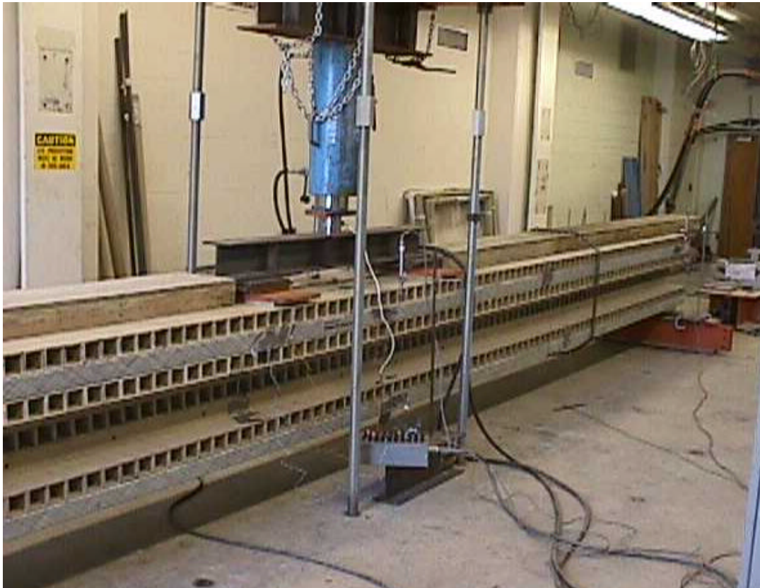
Figure 14: Experimental setup for the four-point static tests on the bridge deck test sample
