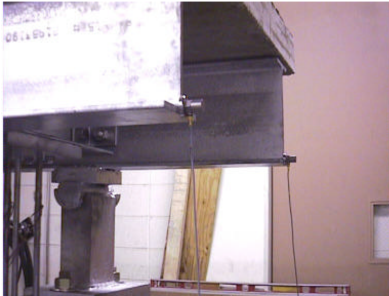
Figure 3.10. Accelerometers Attached to Girders
