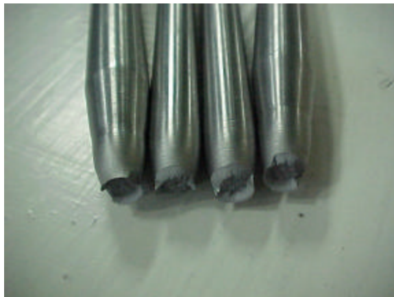
Figure C.5. Fracture Surface, Tests 2 and 3
