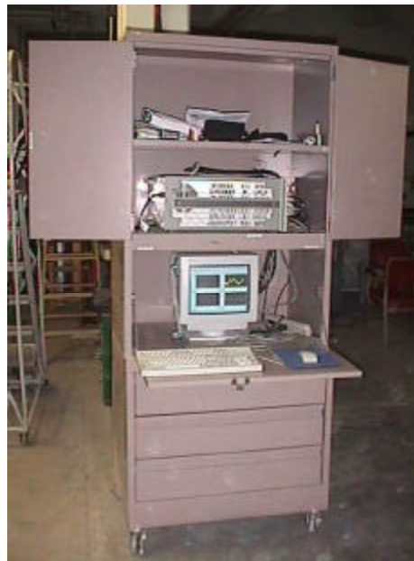
Figure 2.11. HP VXI Unit Used to Generate Input Data
