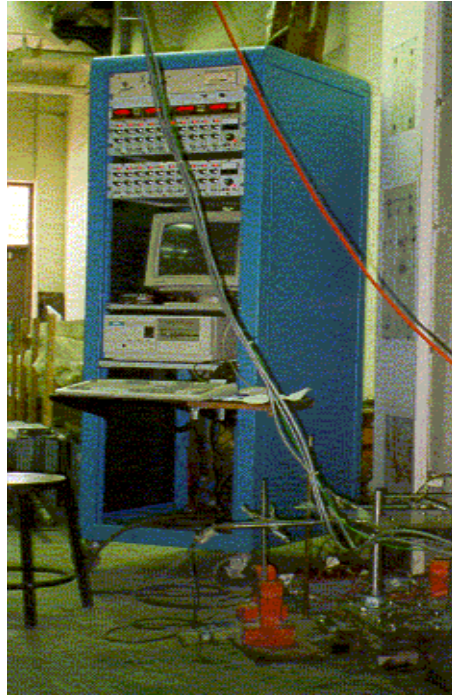
Figure 2.12. Data Acquisition System for Full-Scale Dampers
