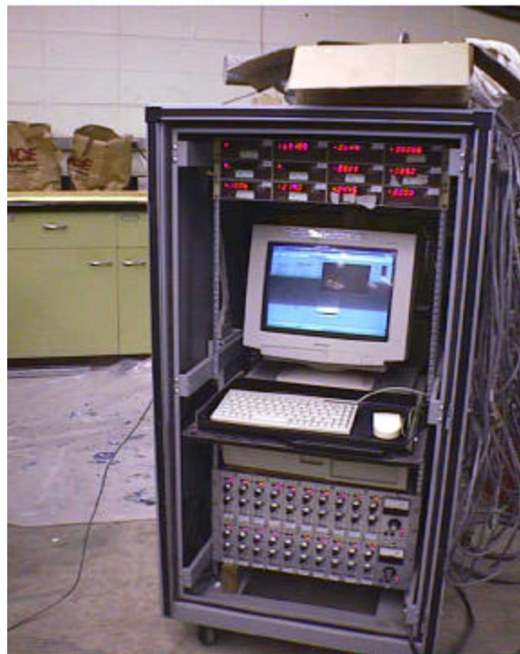
Figure 3.11. Data Acquisition Unit for Small-Scale Bridge
