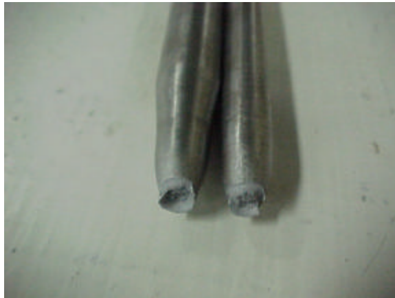
Figure C.4. Fracture Surface, Test 1
