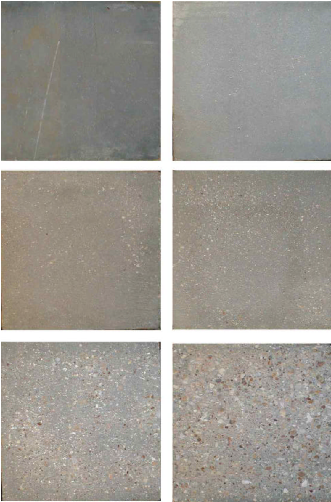
Figure 1. Initial test samples, 0,1,2,3,4,5, in order of roughness.
