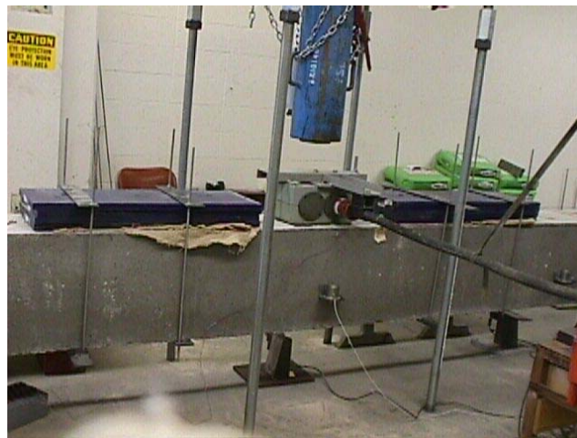
Figure 2.1 Steel plates as preload
