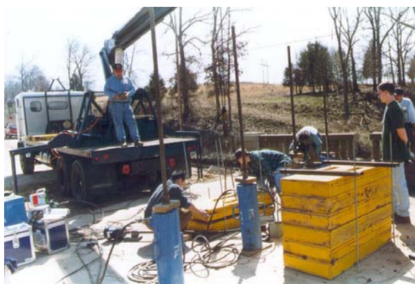
Figure 5.4 Preloading before dynamic tests
