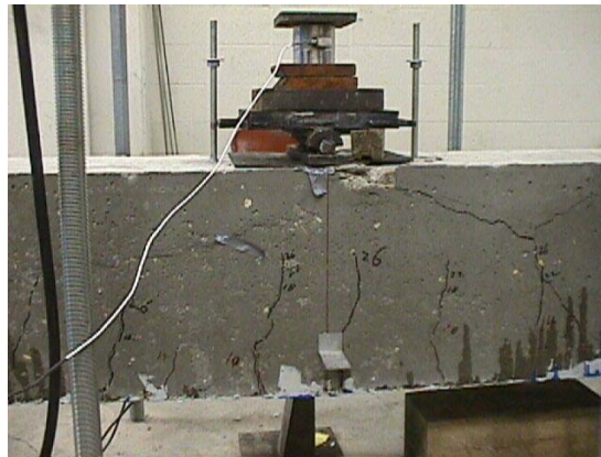
Figure 4.16 Failure of a CFRP strengthened beam
