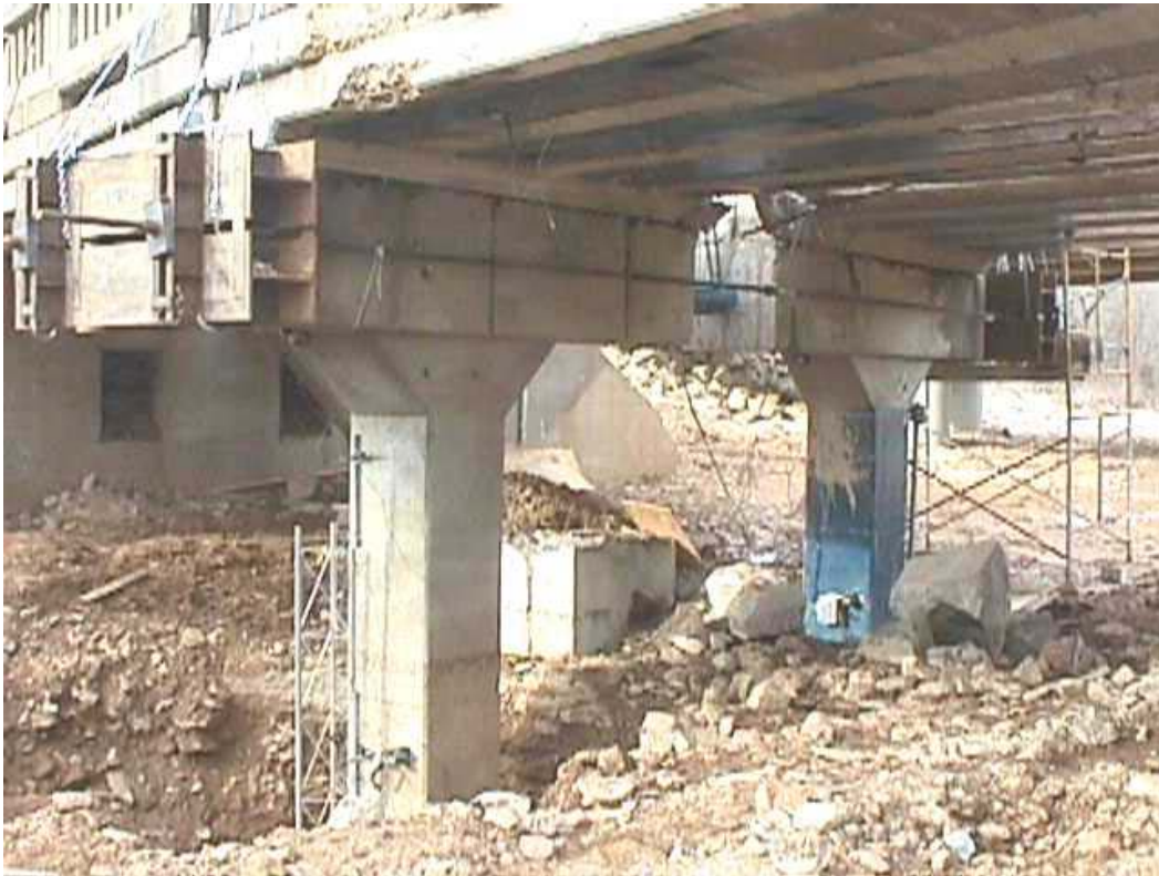
Figure 3.10. Photo showing piers test setup.
