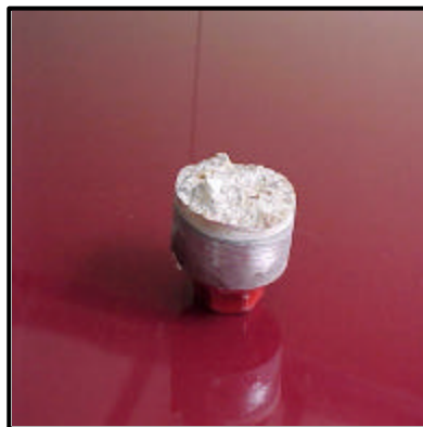
Figure 7.10. Adhesion Fixture Showing Concrete Failure Mode .
