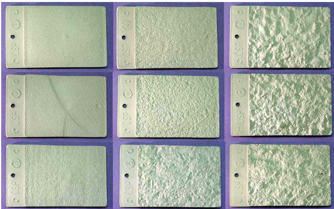
Figure 13: Plastic model concrete surface profiles. The profiles are ordered 1 to 9 in order of increasing roughness, and correspond to acid etching, grinding, light shotblast, light scarification, medium shotblast, medium scarification, heavy abrasive blast, scabbing, and heavy scarification.
