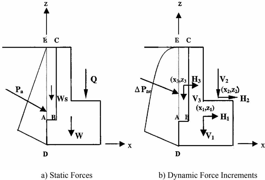
**Figure 6.3** Forces Acting on the Non-Integral Bridge Abutment
