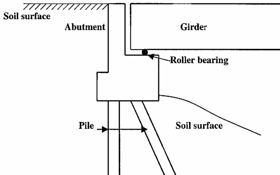
**Figure. 6.1** Typical Non-Integral Bridge Abutment Supported on Piles
