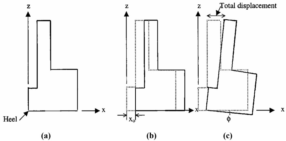
**Figure 6.2** Translation and Rotation Movement of Bridge Abutment Forces Acting on the Non-Integral Bridge Abutment
