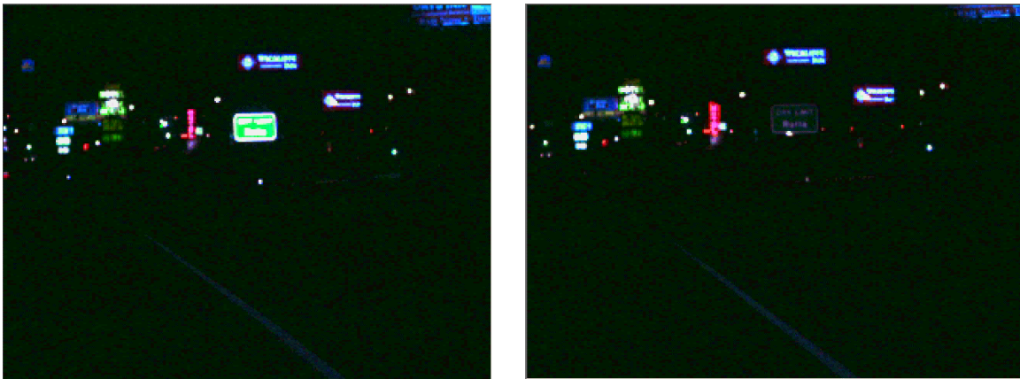
FIGURE 8. Left: High beam image. Right: Low beam image. Note that the green sign in the left image almost completely disappears in the cluttered background of “lit” signs
