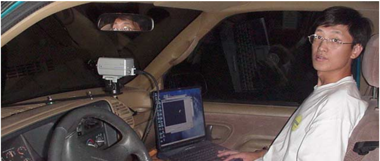
FIGURE 2. In-vehicle installation consists of a dash mounted digital camera, attached to a laptop computer.
