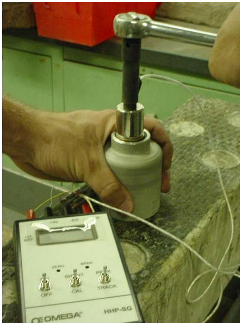
Figure 3. The pull-off tester used in a tensile mode.
