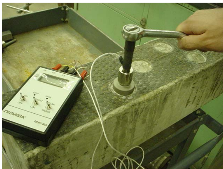
Figure 2. Pull-off tester used in a shear mode.
