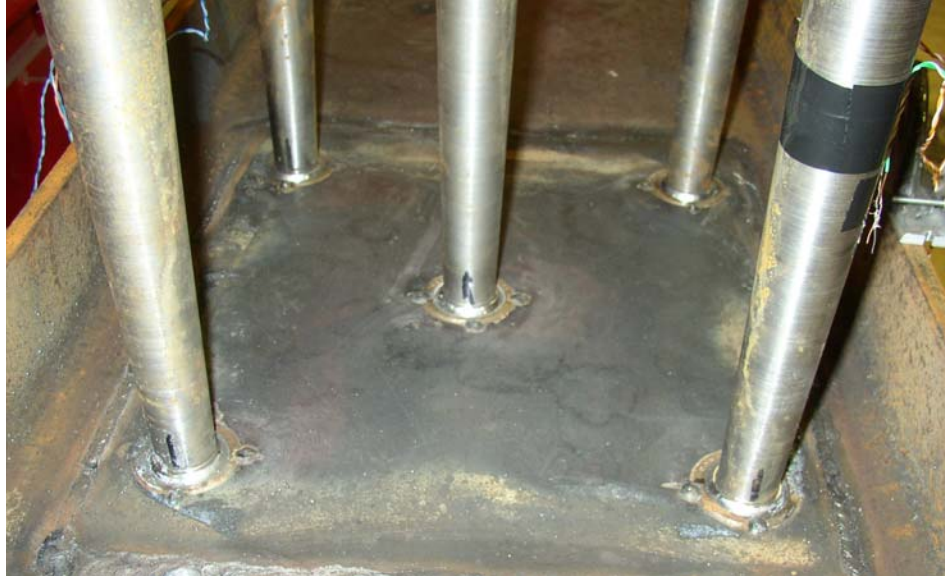
Figure 4.5 Ball Joint Connections
