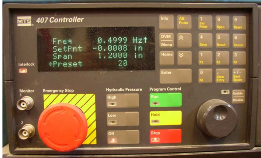
Figure 2.11 MTS 407 Input Control Screen
