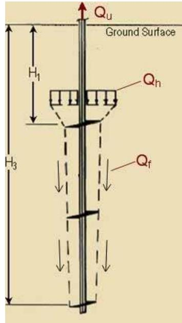
Figure 3.2. Cylindrical Shear Friction Capacity Method
