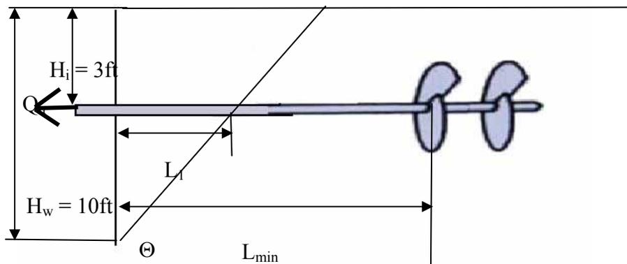
Soil Parameters:  $\gamma = 105 \text{ pcf}$ ,  $c = 0 \text{ psf}$ ,  $\phi = 30^\circ$
