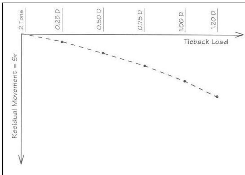
Figure 5.1. Typical Proof Test Results
