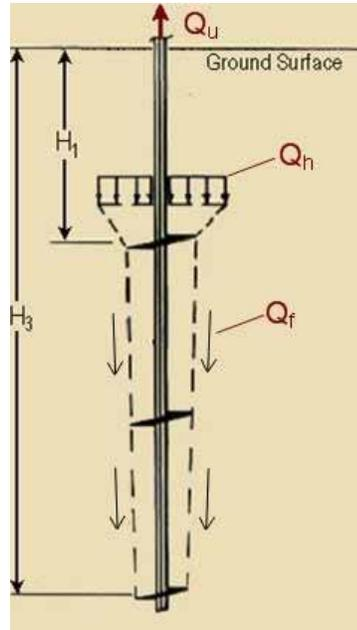
Figure 3.2. Cylindrical Shear Friction Capacity Method
