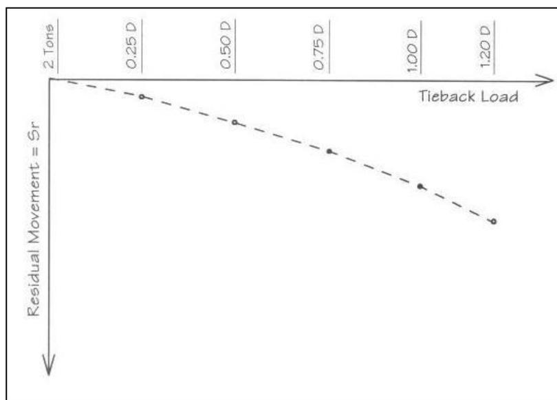
Figure 5.1. Typical Proof Test Results
