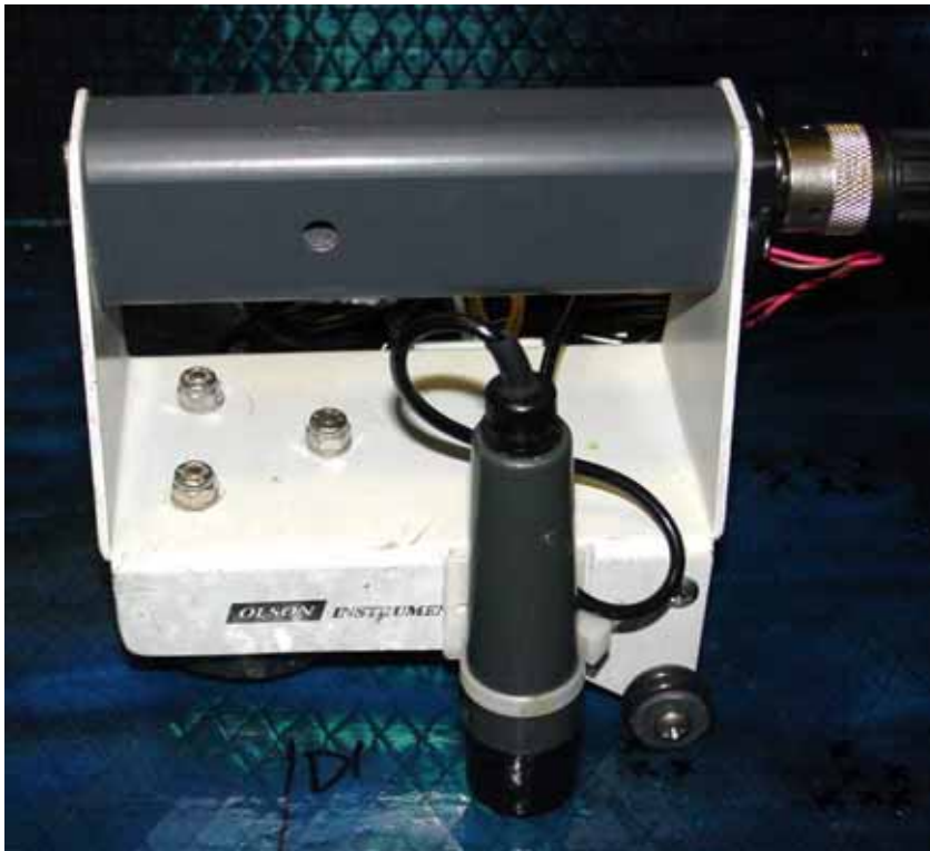
Figure 2. CFG-1TF modified impact echo testing device, with air coupled microphone.
