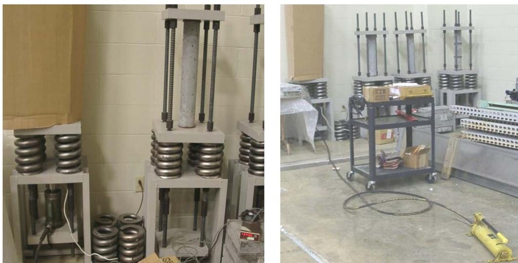
Figure 3.3 Creep Loading Frame and Specimens
