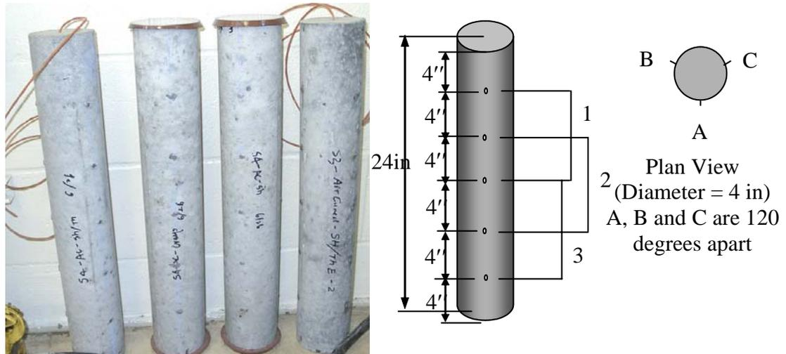
Figure 3.1 C/S/T Specimens and DEMEC Points Arrangement
