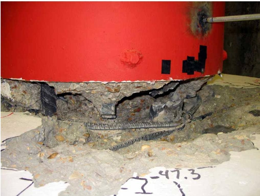
**Figure 0-20. Hoop Buckling Side “B”**
