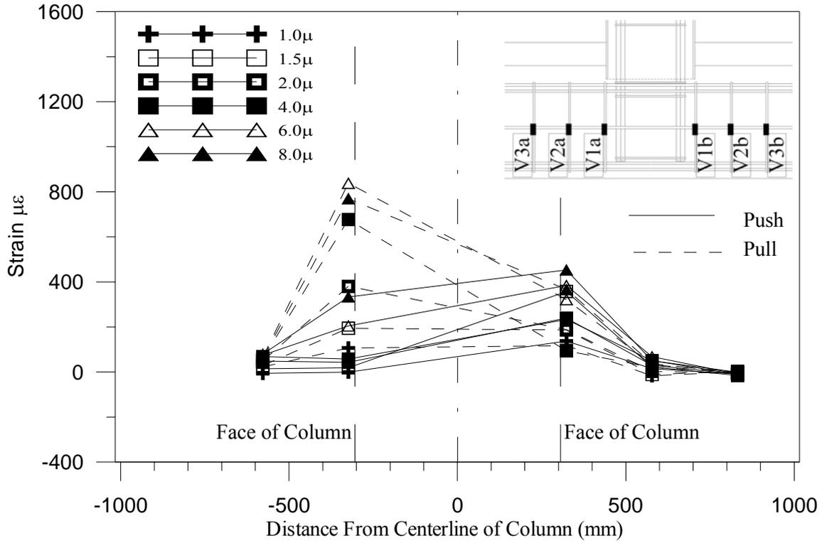
**Figure 0-29. As-Built Strain Gauge Profile**
