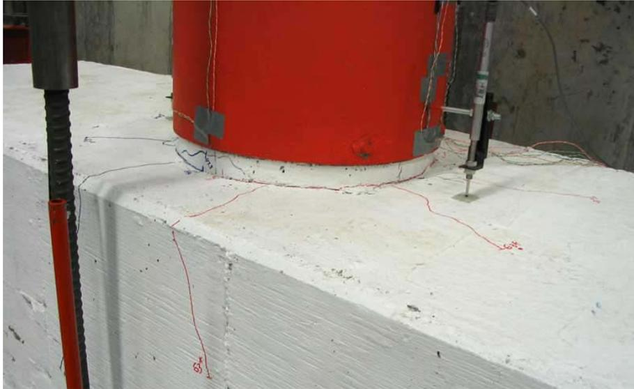
**Figure 0-2. Bent Cap Cracking at 1.00 V<sub>y</sub>**
