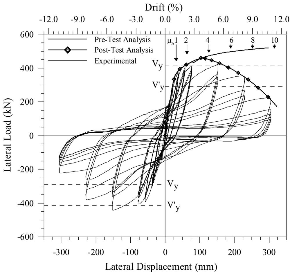
**Figure 0-22. Unit 1 - Load Displacement Response**
