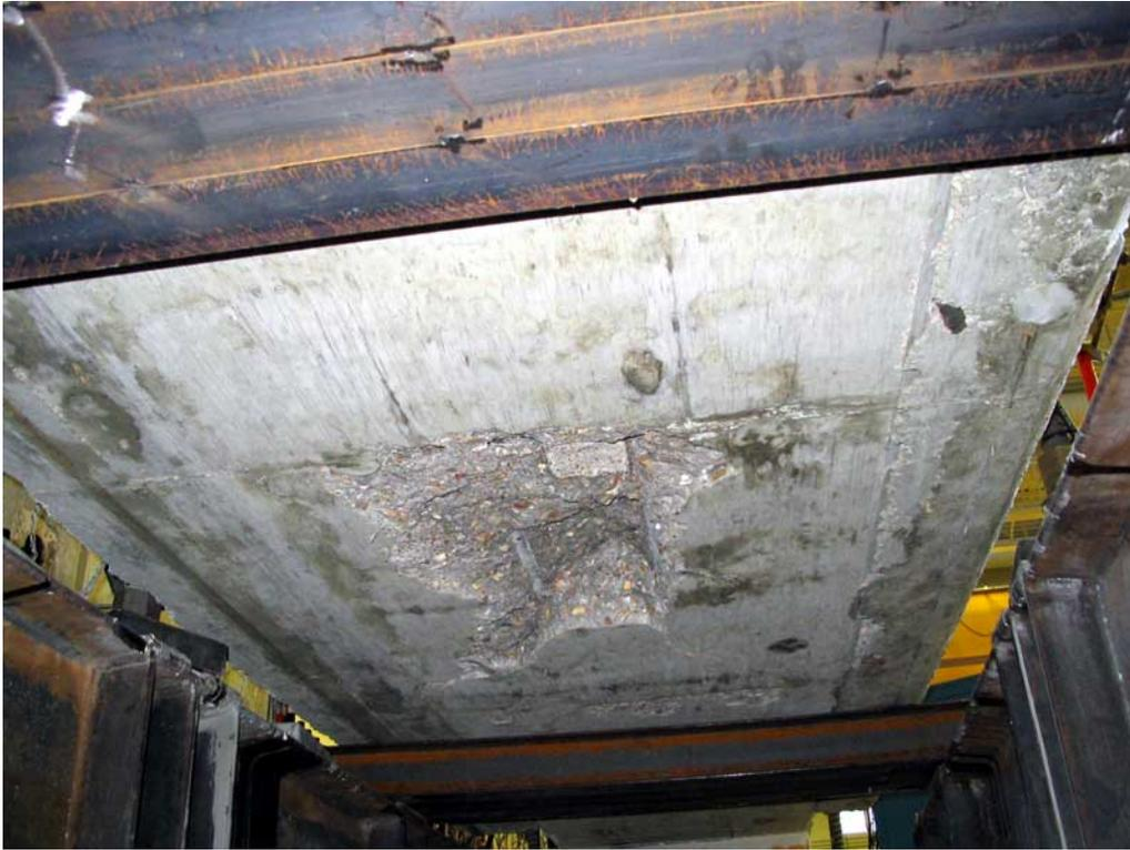
**Figure 0-19. Bent Cap Bottom Spalling at 8.0  $\mu\Delta$**
