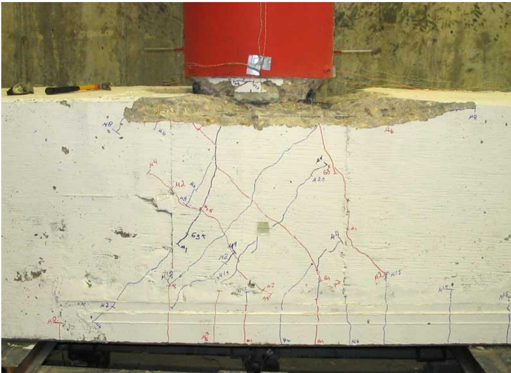
**Figure 0-20. Joint Cracking at 8.0  $\mu\Delta$**
