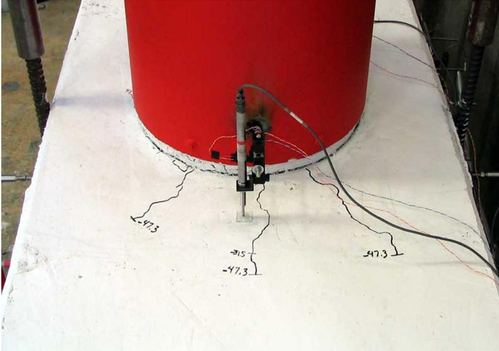
**Figure 0-2. Bent Cap Cracking at  $0.75V_y$**
