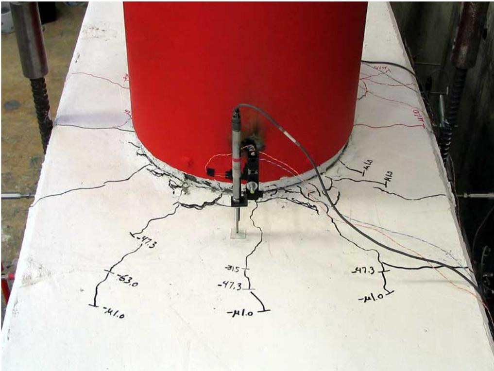
Figure 0-8. Bent Cap Cracking at  $1.5 \mu\Delta$
