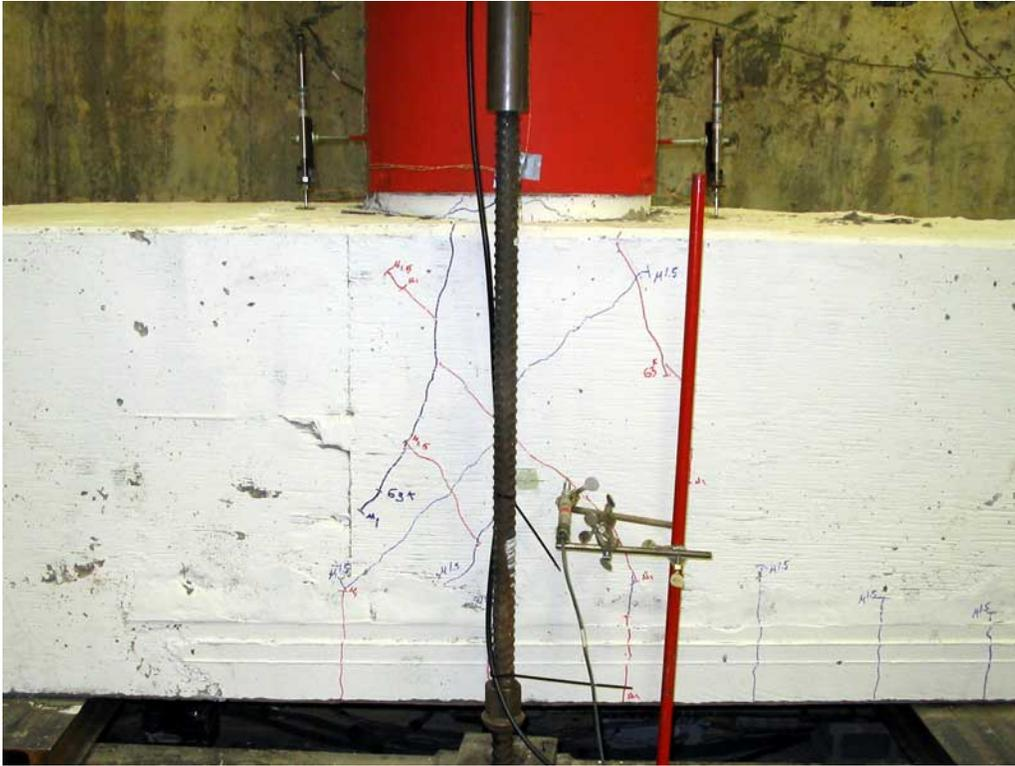
Figure 0-5. Joint Cracking at  $1.5 \mu\Delta$
