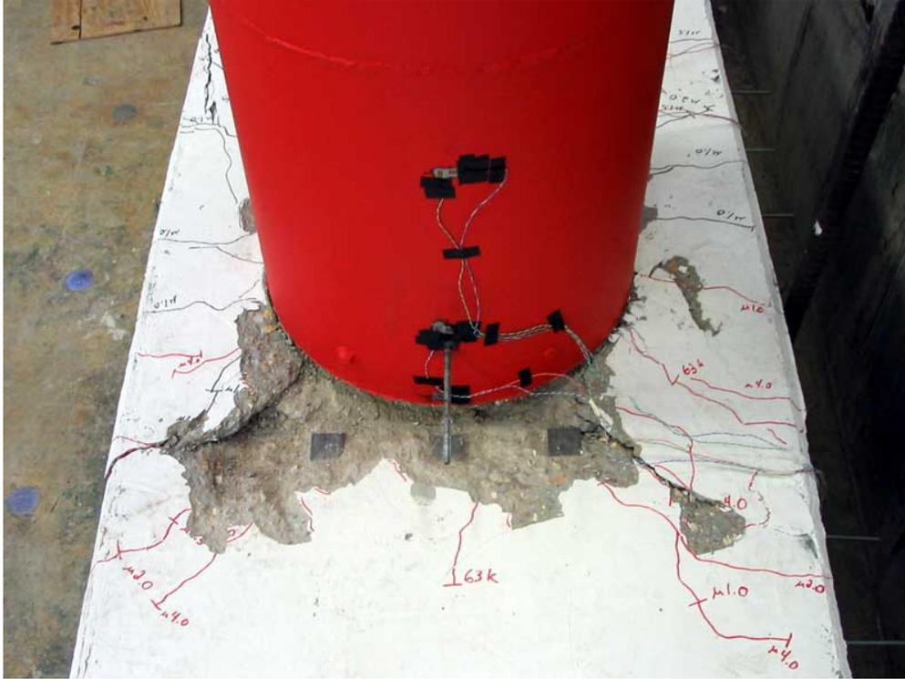
**Figure 0-16. Bent Cap Cracking Ultimate Damage**
