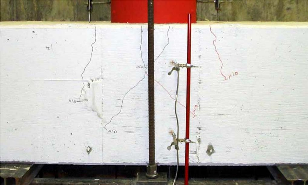
**Figure 0-2. Joint Cracking at 1.0  $\mu\Delta$**
