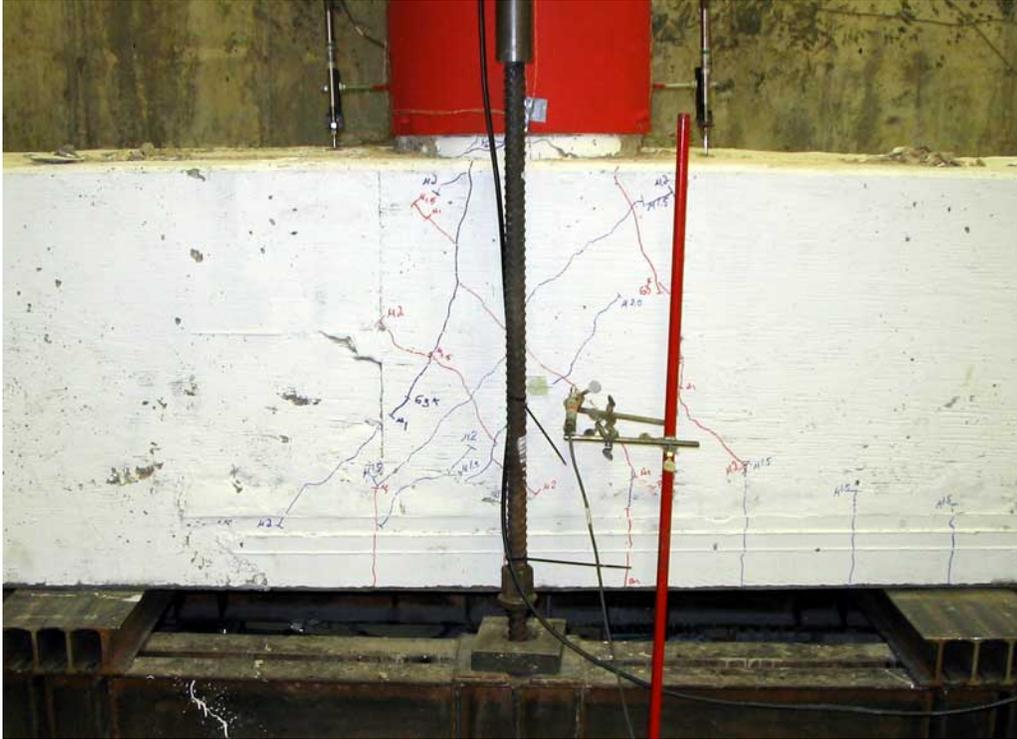
**Figure 0-7. Joint Cracking at 2.0  $\mu\Delta$**
