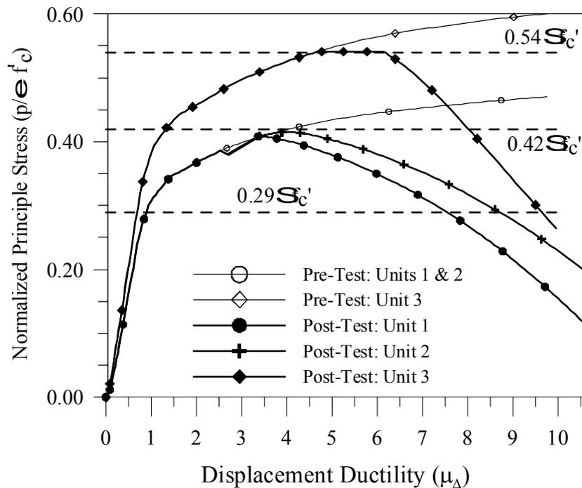
**Figure 0-5. Post-Test Analysis**
