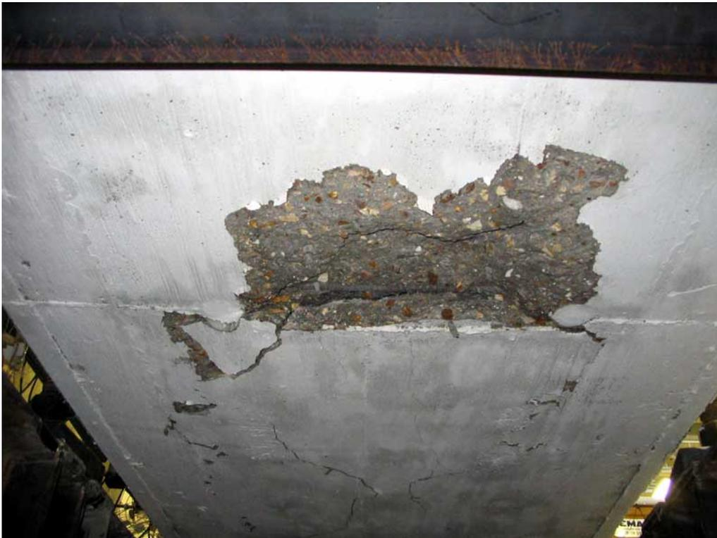
**Figure 0-15. Bent Cap Underside Cracking at 8.0  $\mu\Delta$**
