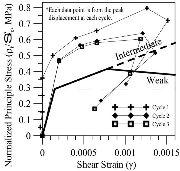
**Figure 0-31. Unit 3 Principle Tensile Stress vs. Joint Shear Strain**
