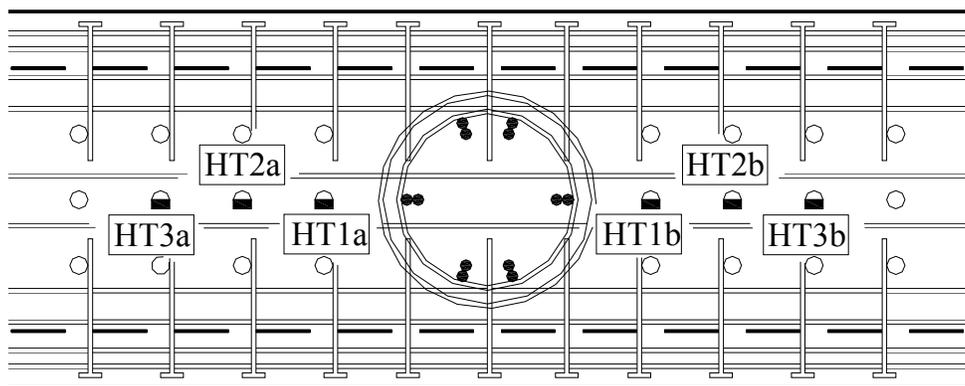
**Figure 0-7. Retrofit Vertical Headed Reinforcement Strain Gauges**
