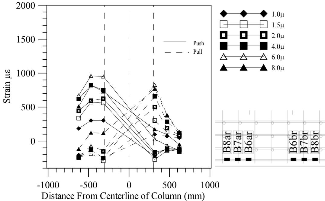
**Figure 0-32. Retrofit Strain Gauge Profile**
