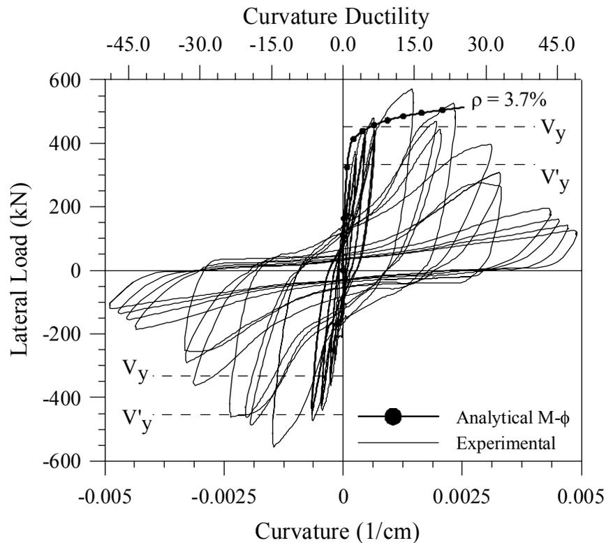
**Figure 0-21. Unit 3 – Load versus Curvature Response**
