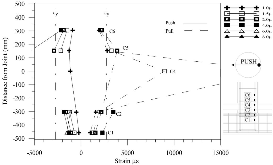
Figure 0-26. Strain Gauge Profile – Side "A"
