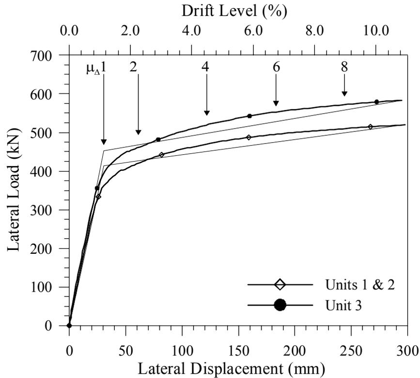
**Figure 0-1. Predicted Force-Displacement Response of Units 1, 2 and 3**
