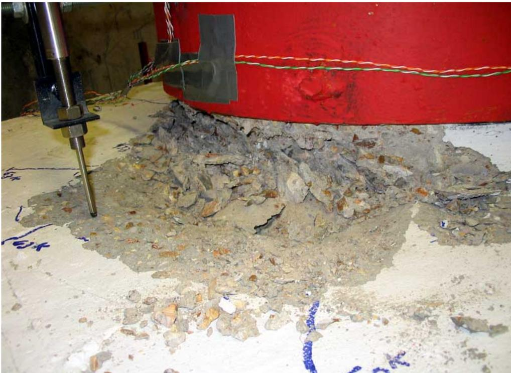
**Figure 0-12. Column Concrete Crushing at  $4.0 \mu\Delta$**
