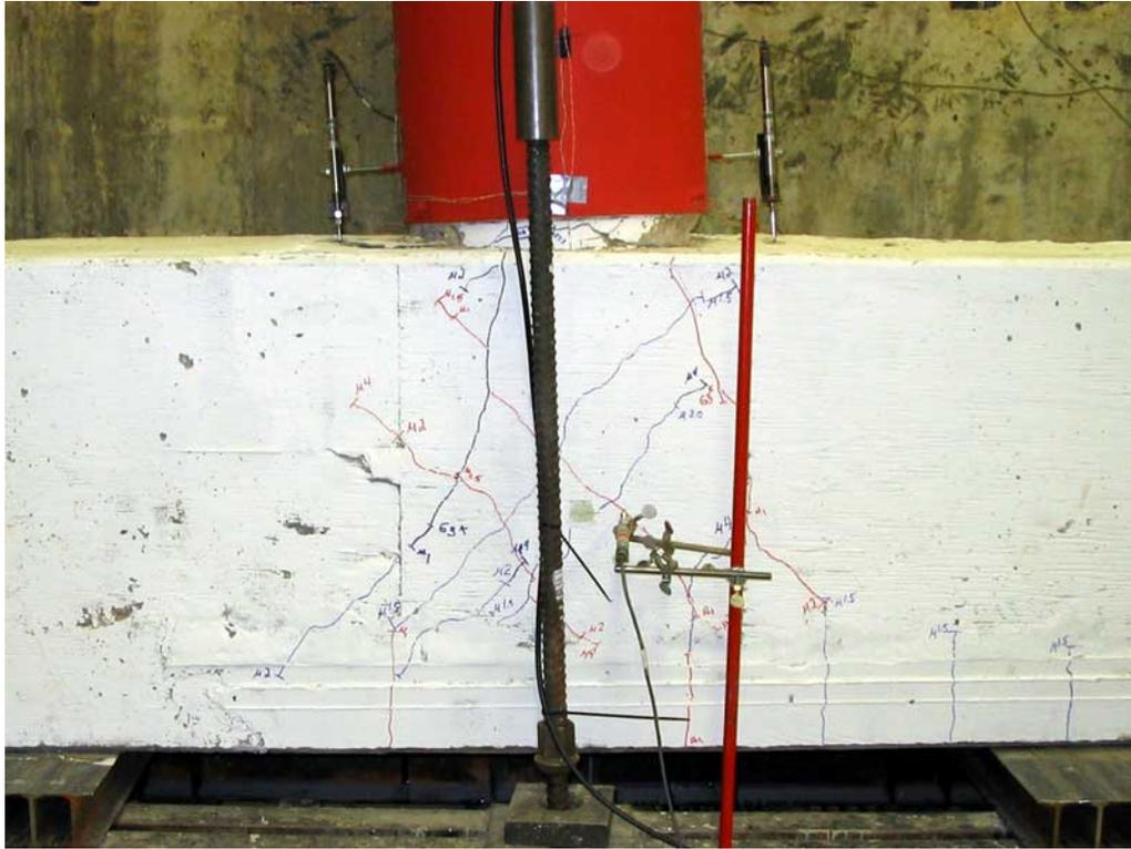
**Figure 0-9. Joint Cracking at 4.0  $\mu\Delta$**
