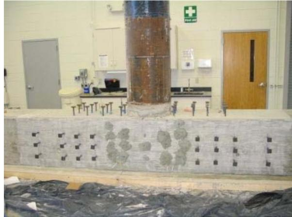
**Figure 0-8. Installed Headed Reinforcement**
