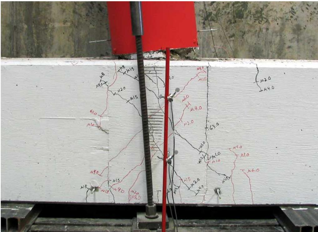
**Figure 0-16. Joint Cracking at 8.0  $\mu\Delta$**
