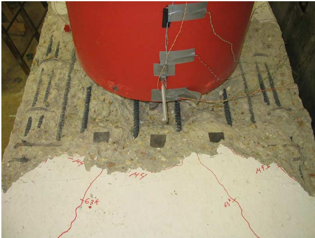
**Figure 0-21. Bent Cap Ultimate Damage**
