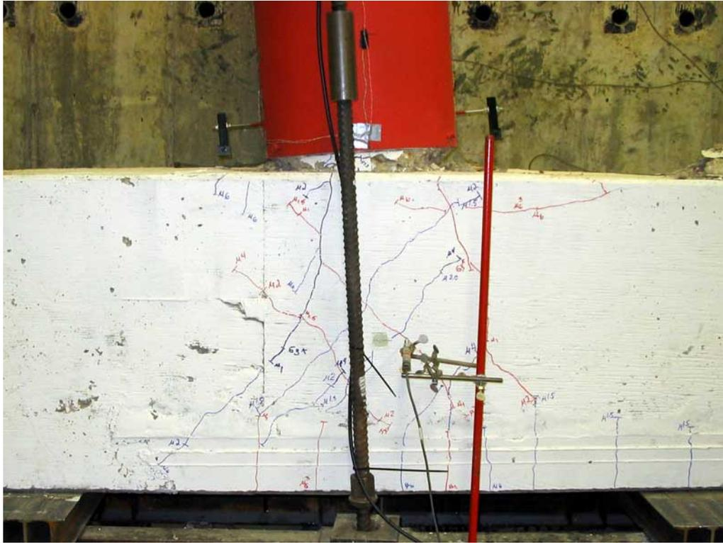
**Figure 0-13. Joint Cracking at 6.0  $\mu\Delta$**
