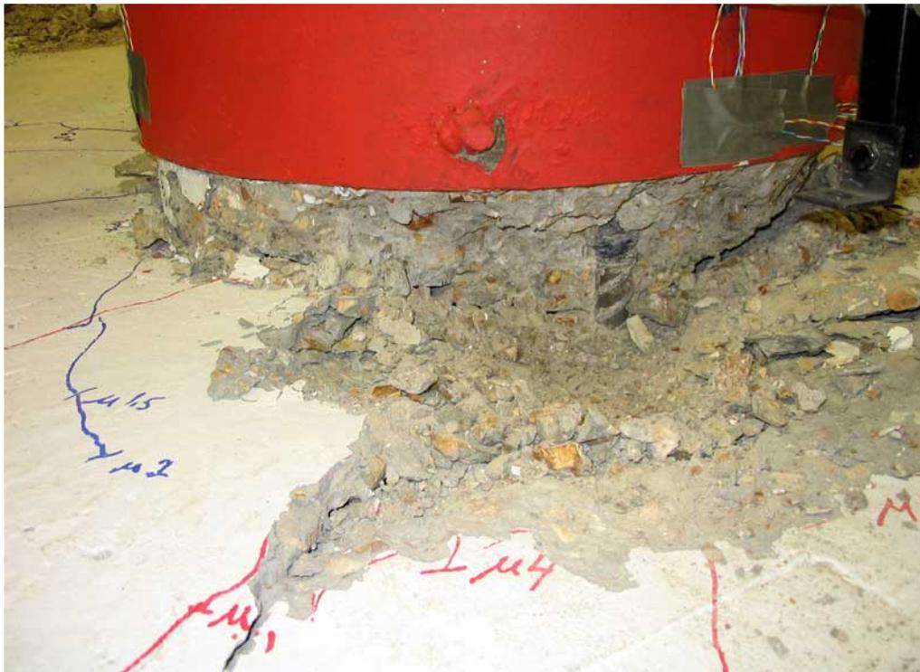
**Figure 0-14. Column Concrete Crushing at 6.0  $\mu\Delta$**
