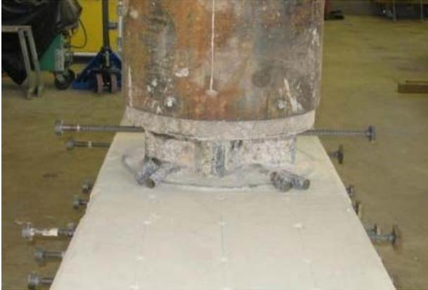
**Figure 0-3. Detail at Bent Cap Interface**
