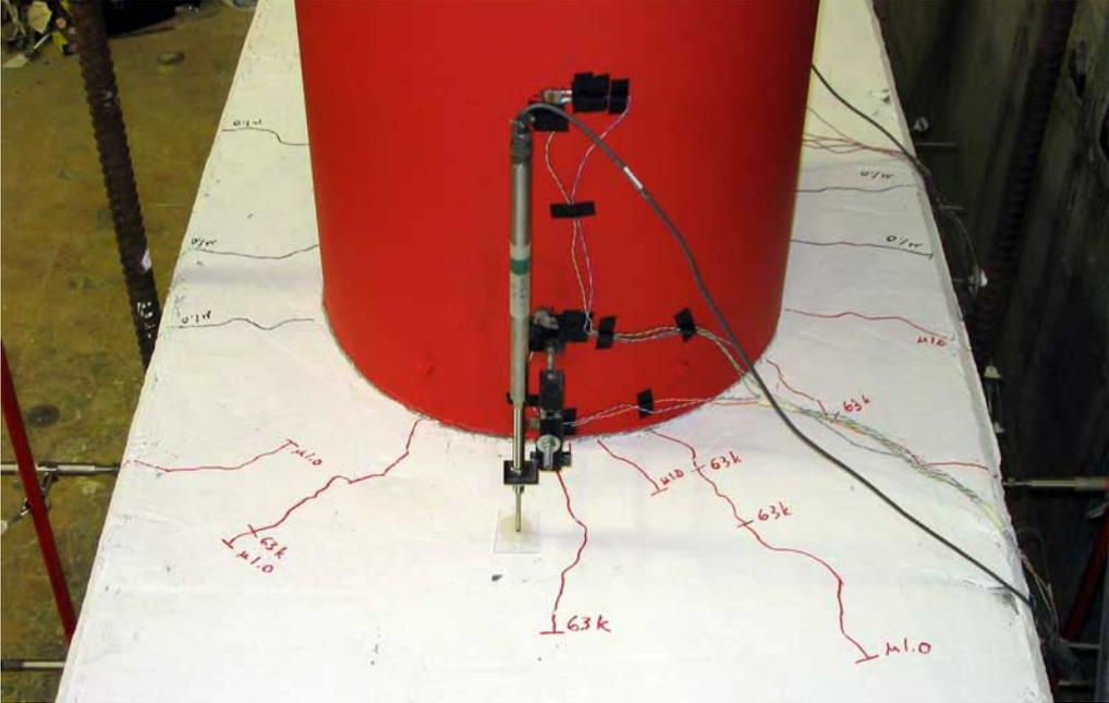
**Figure 0-3. Bent Cap Cracking at 1.0  $\mu\Delta$**
