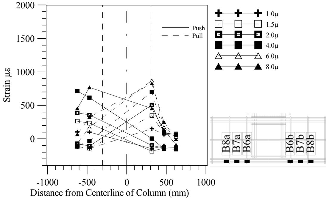
Figure 0-31. As-Built Bent Strain Gauge Profile
