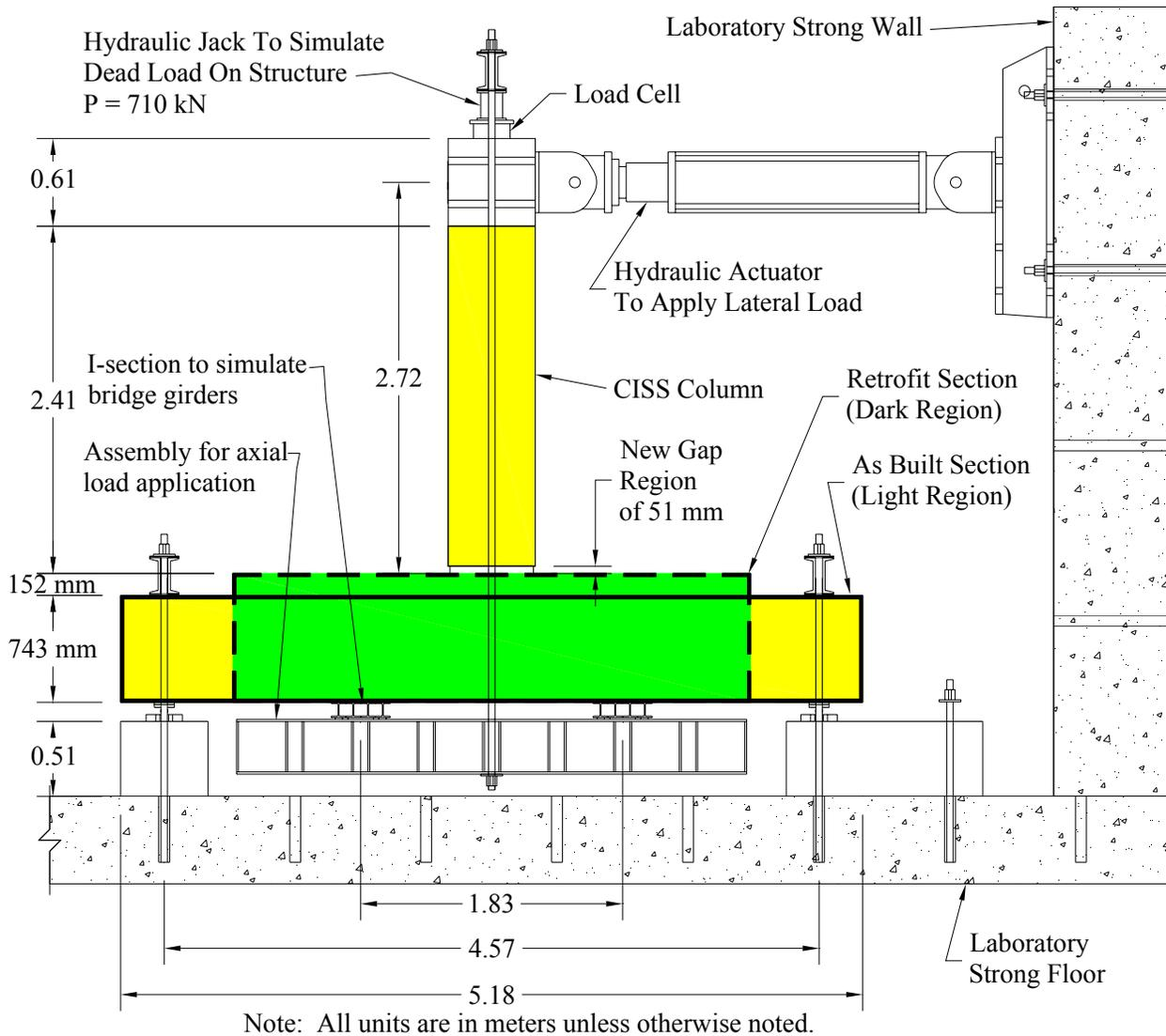
**Figure 0-1. Test Setup**
