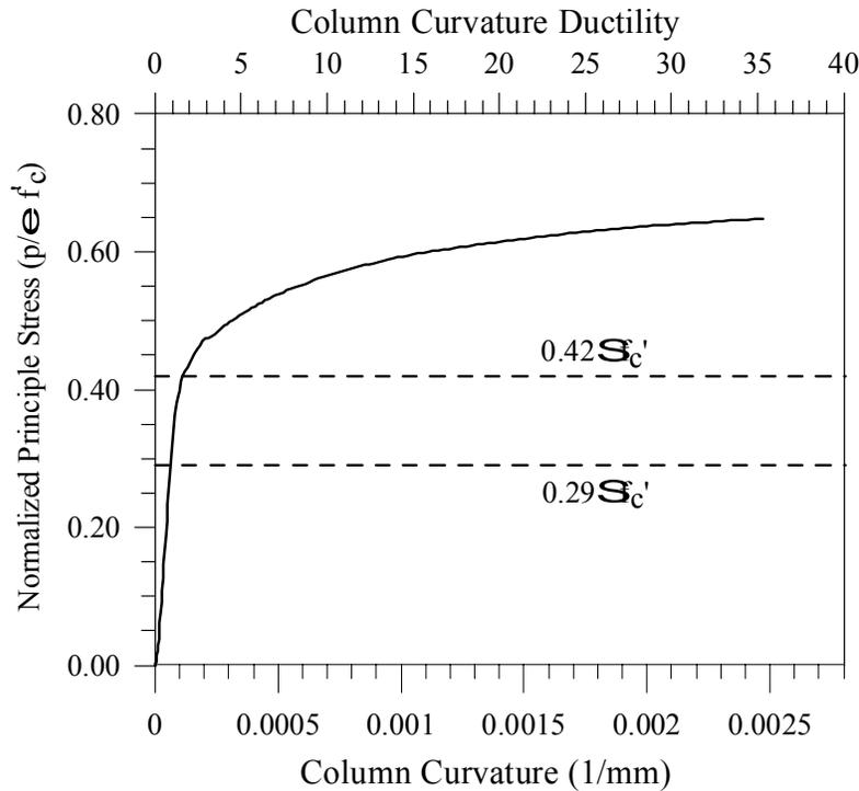
**Figure 0-7. Joint Principle Tensile Stresses - Retrofitted Column**
