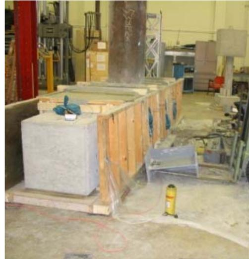
**Figure 0-25. Forming Retrofit Section**
