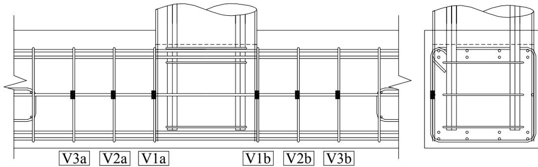
Figure 0-3. As-Built Bent Cap Shear Strain Gauges
