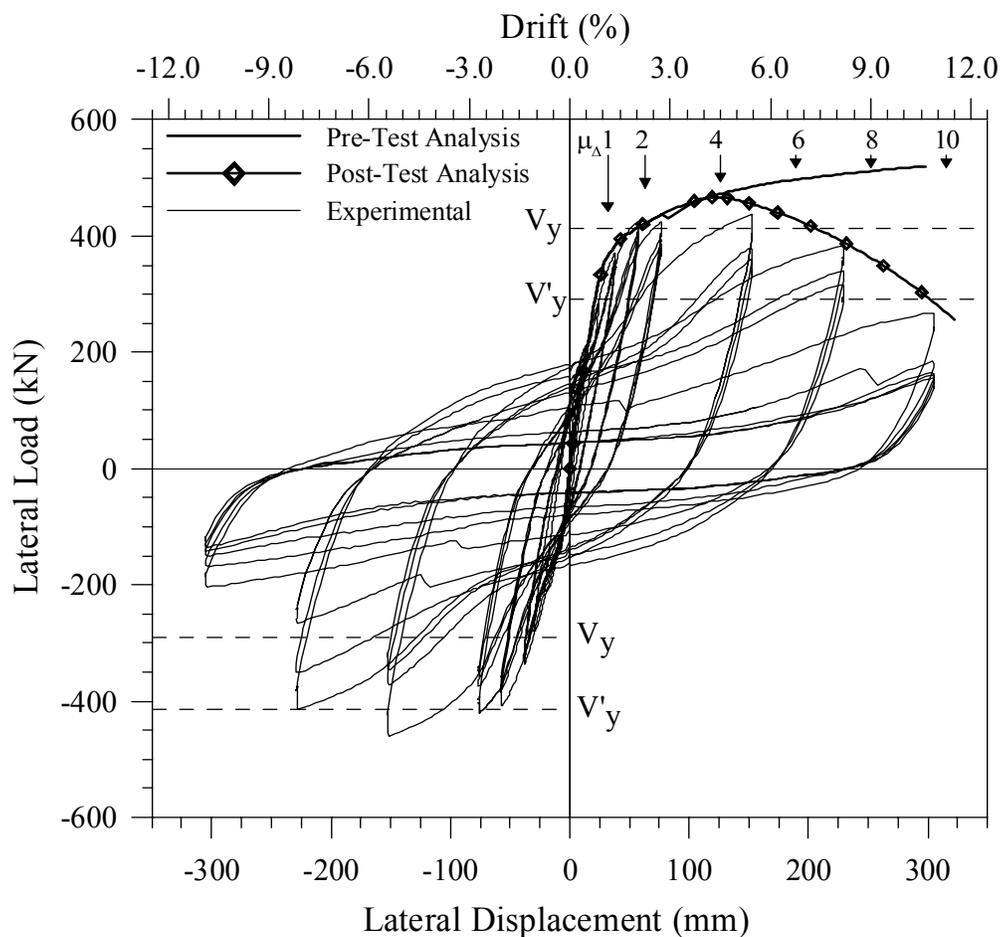
**Figure 0-21. Unit 2 – Load Displacement Response**
