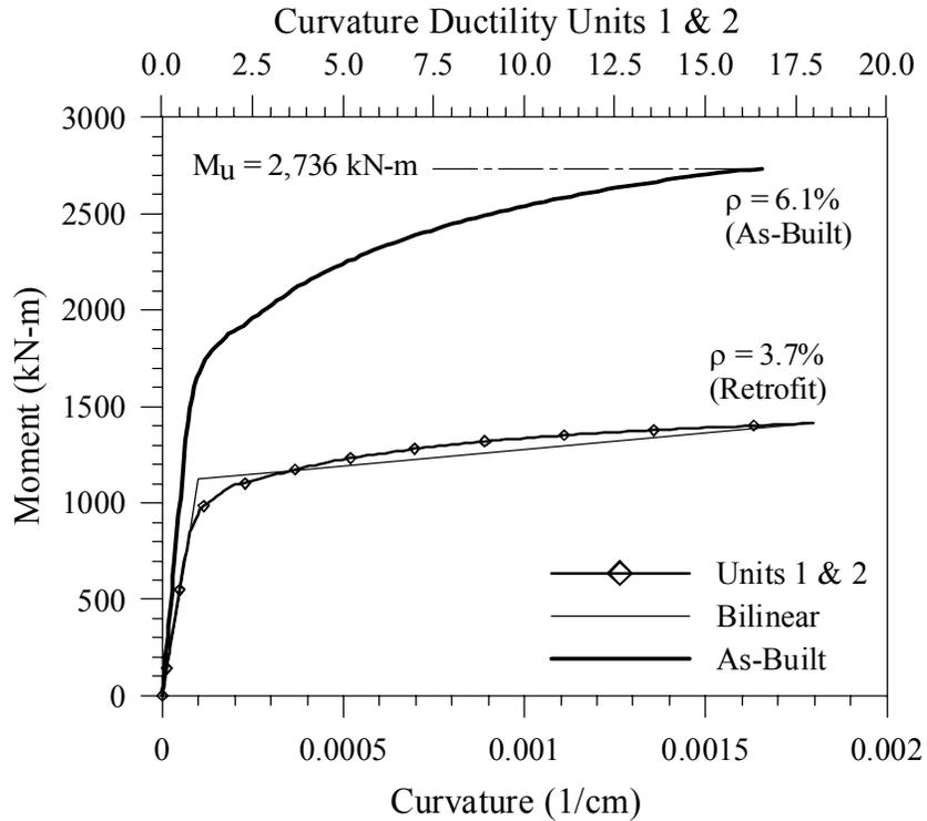
**Figure 0-3. Column Moment Curvature**
