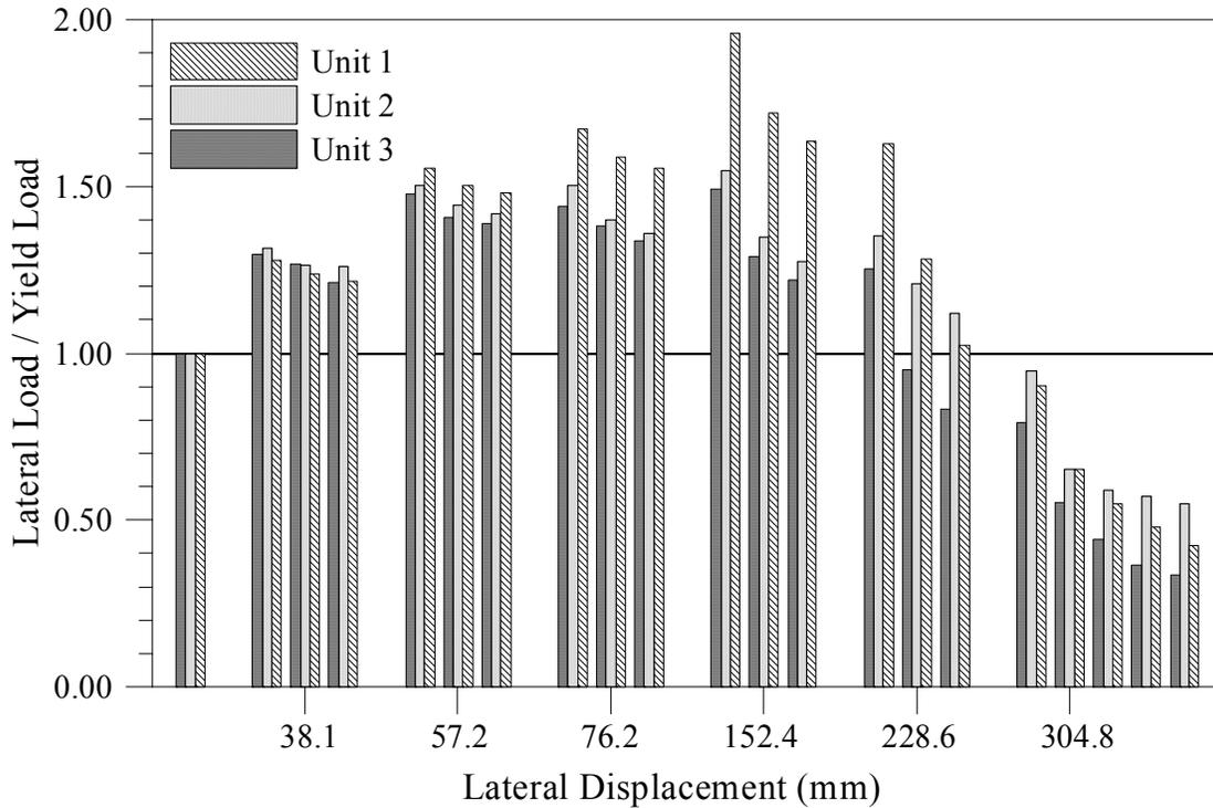
**Figure 0-2. Strength Degradation under Reversed cyclic loading**
