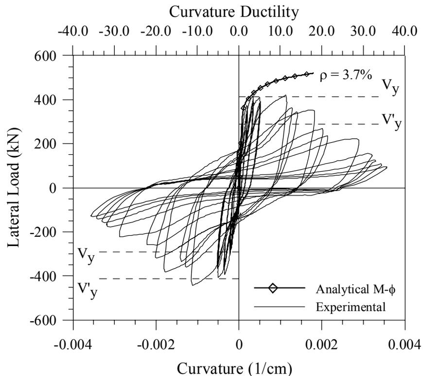
Figure 0-23. Unit 1 – Load versus Curvature Response
