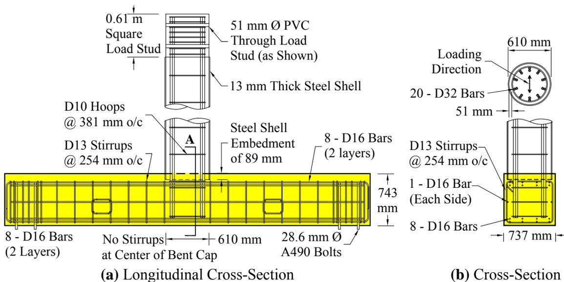
**Figure 0-2. As-Built Reinforcement Layout**
