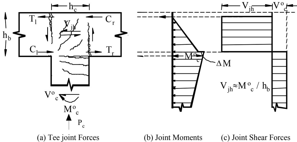
**Figure 0-6. Joint Shear Forces in Bridge Tee Joints**
