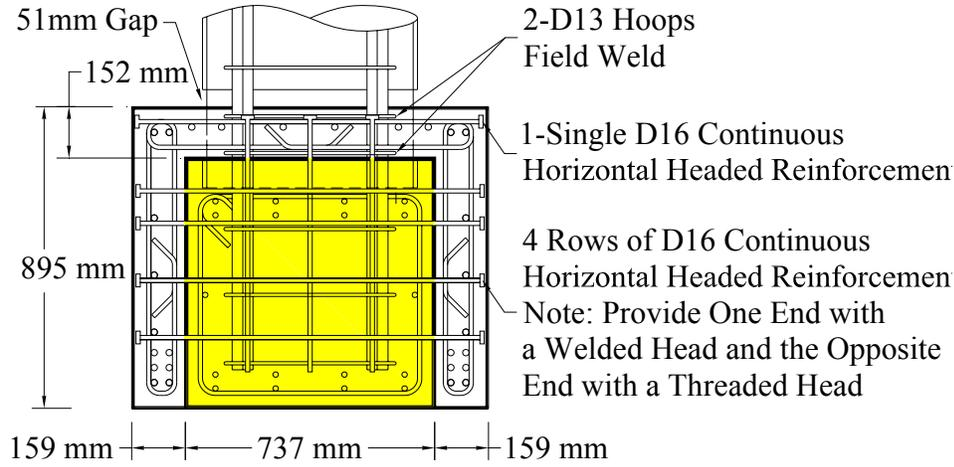
**Figure 0-1. Unit 2 Retrofit Cross-Section**
