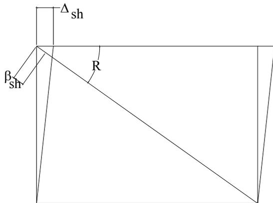
(e) Shear Deformation
