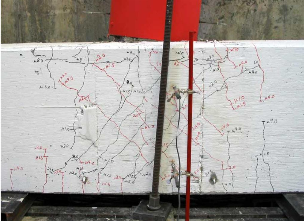
Figure 0-12. Joint Cracking at 8.0  $\mu\Delta$
