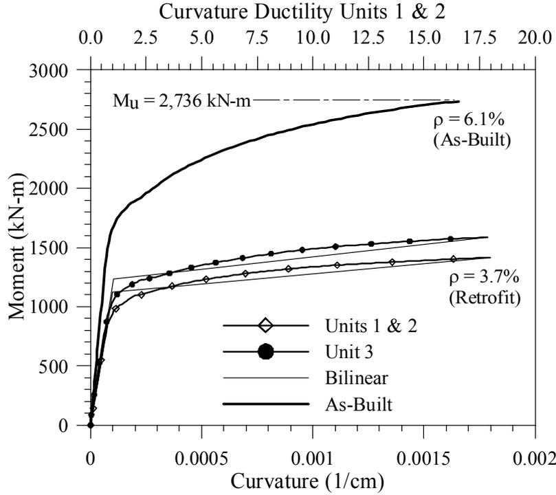
**Figure 0-4. Unit 3 Moment-Curvature**
