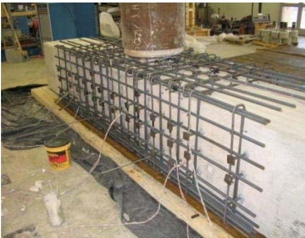
**Figure 0-5. Bent Cap Retrofit Section**
