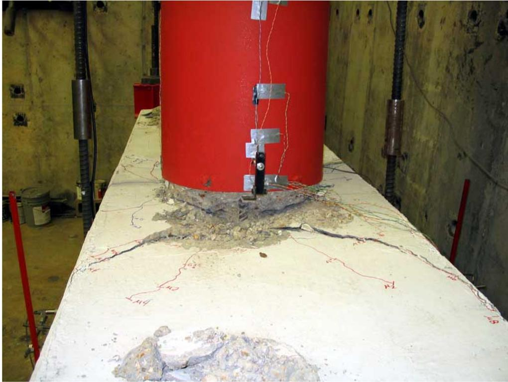
**Figure 0-17. Bent Cap Cracking at  $8.0 \mu\Delta$**
