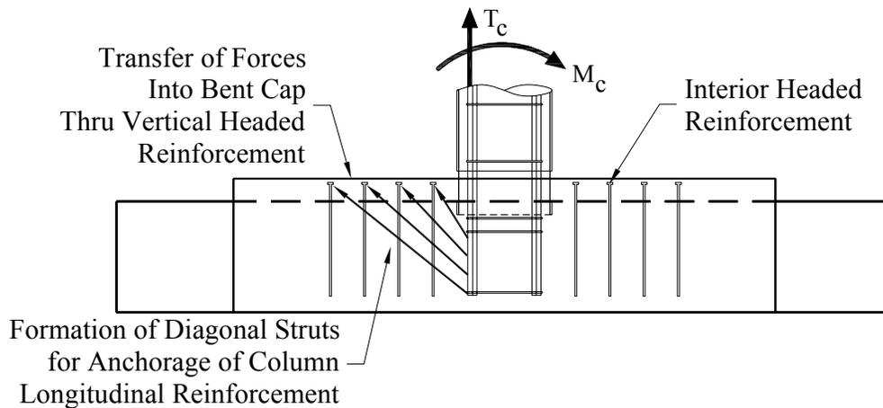
**Figure 0-11. Column Strut Forces**
