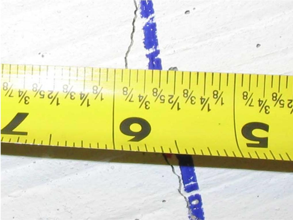
**Figure 0-11. Joint Crack Width at  $4.0 \mu\Delta$**
