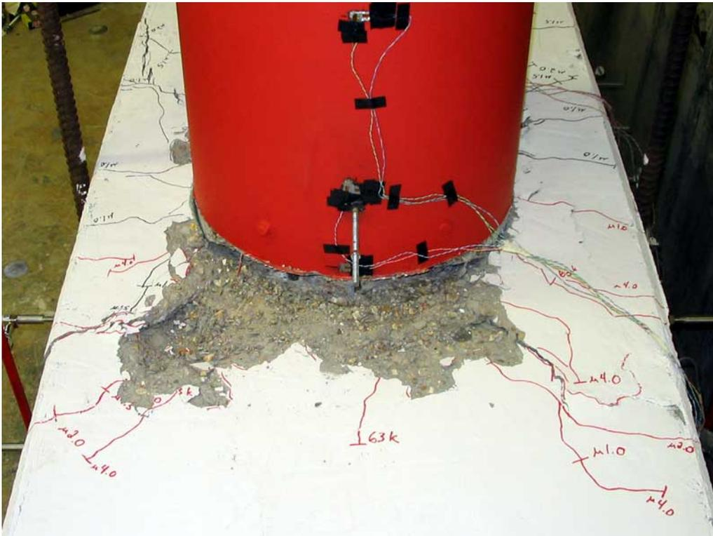
Figure 0-13. Bent Cap Cracking – Side “A” at 8.0  $\mu\Delta$
