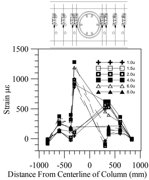
**Figure 0-36. Unit 2 Top Transverse Reinforcement Strain Profile**
