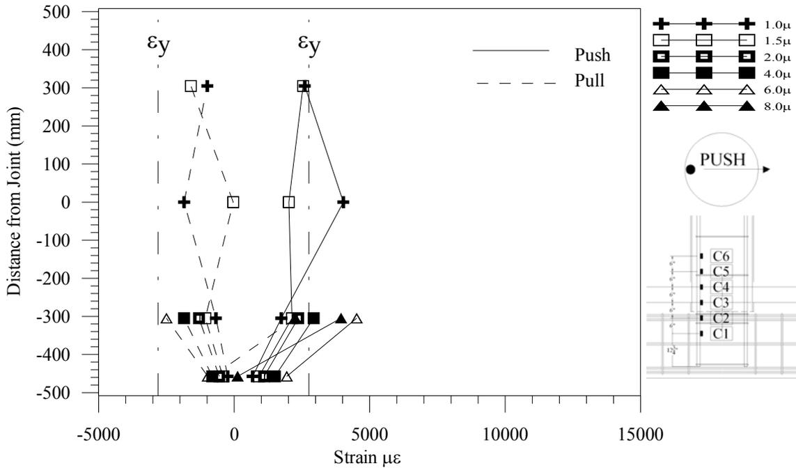
**Figure 0-28. Strain Gauge Profile – Side “B”**
