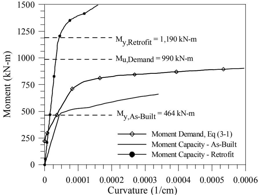
**Figure 0-5. Bent Cap Moment Curvature**
