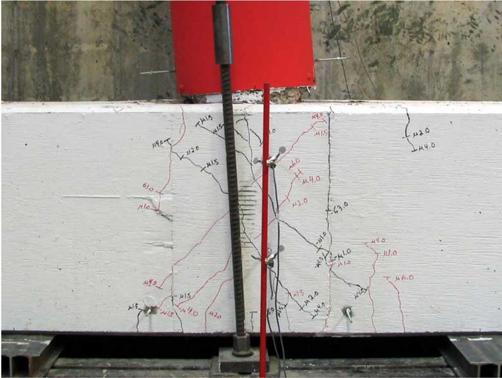
**Figure 0-13. Joint Cracking at 6.0  $\mu\Delta$**
