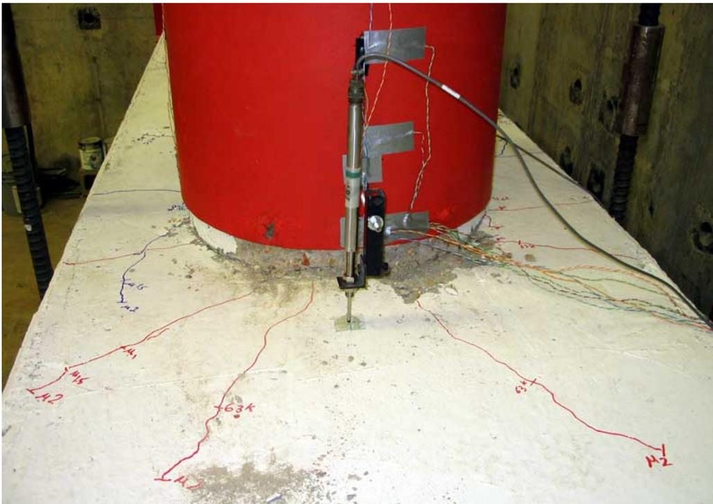
**Figure 0-8. Bent Cap Cracking at 2.0  $\mu\Delta$**
