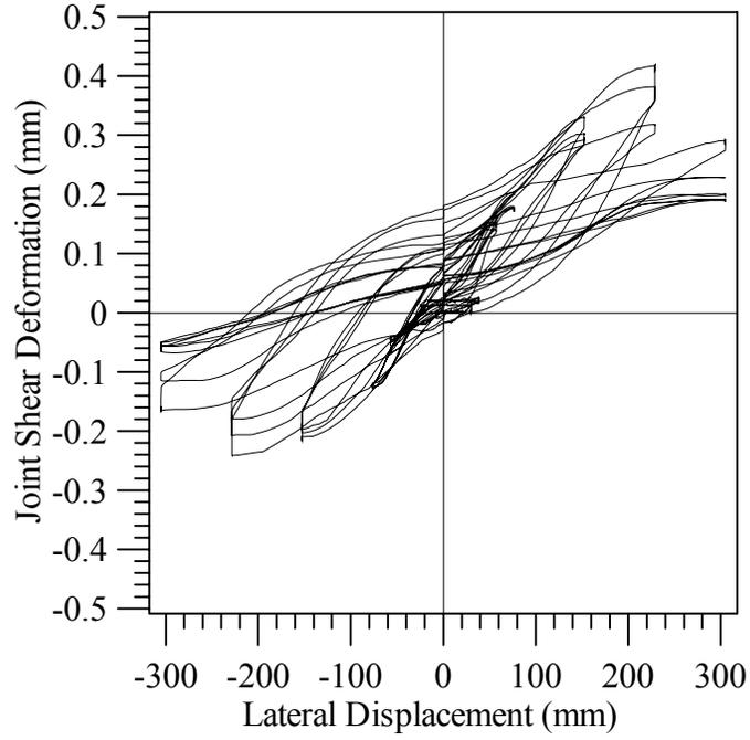
**Figure 0-33. Specimen #2 Joint Shear Deformation**
