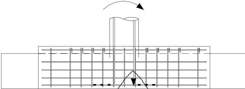
**Figure 0-32. Confinement of Column Anchorage Failure**
