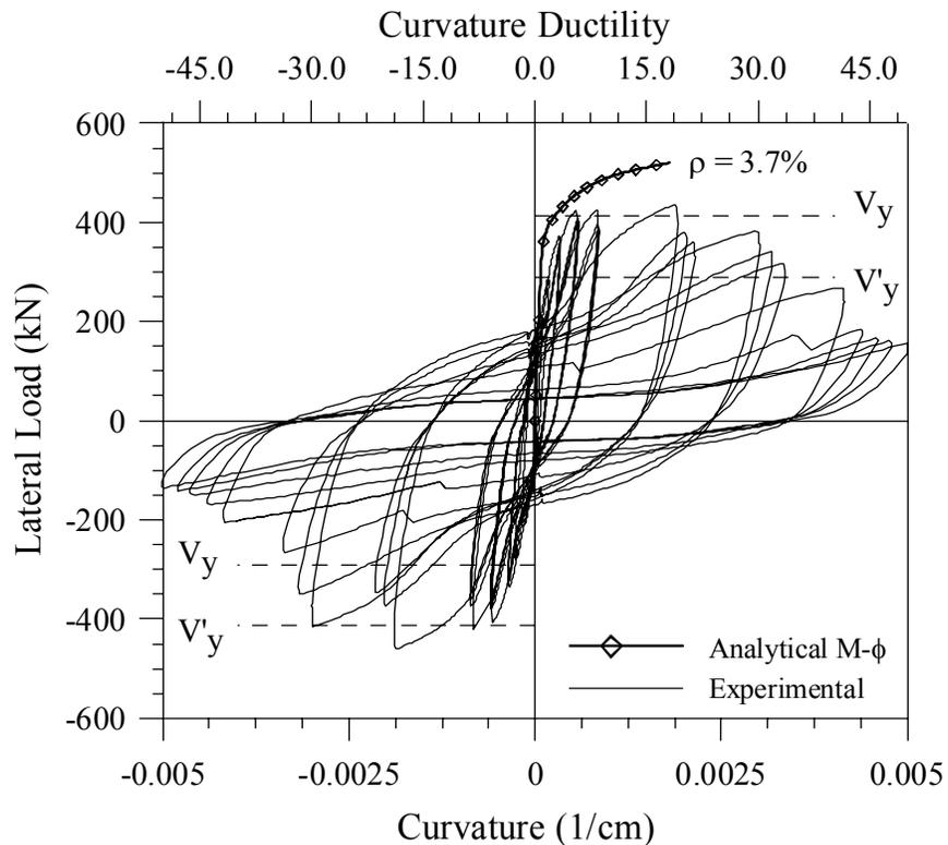
**Figure 0-24. Unit 2 – Load versus Curvature Response**
