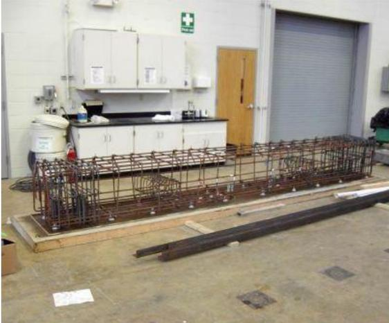
**Figure 0-13. Bent Cap Reinforcing Cage**
