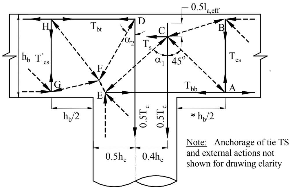
**Figure 0-8. Joint Force Transfer Model (Sritharan, 1999)**
