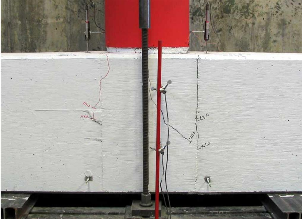
**Figure 0-5. Joint Cracking at 1.0  $\mu\Delta$**
