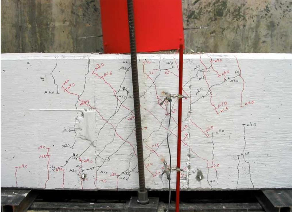
Figure 0-10. Joint Cracking at  $6.0 \mu\Delta$
