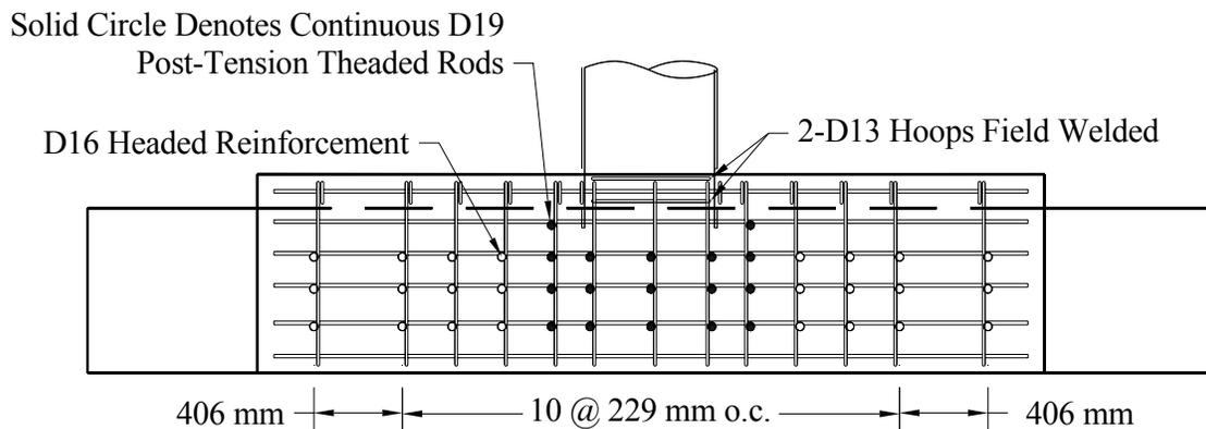
**Figure 0-2. Unit 3 Retrofit Reinforcement Layout**
