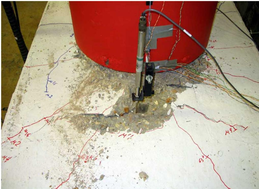
**Figure 0-10. Bent Cap Cracking at 4.0  $\mu\Delta$**
