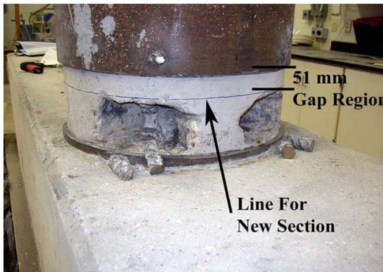
**Figure 0-2. Cut Longitudinal Reinforcement**
