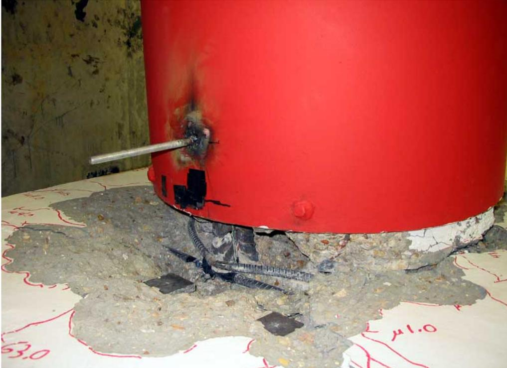
**Figure 0-19. Hoop Buckling Side “A”**
