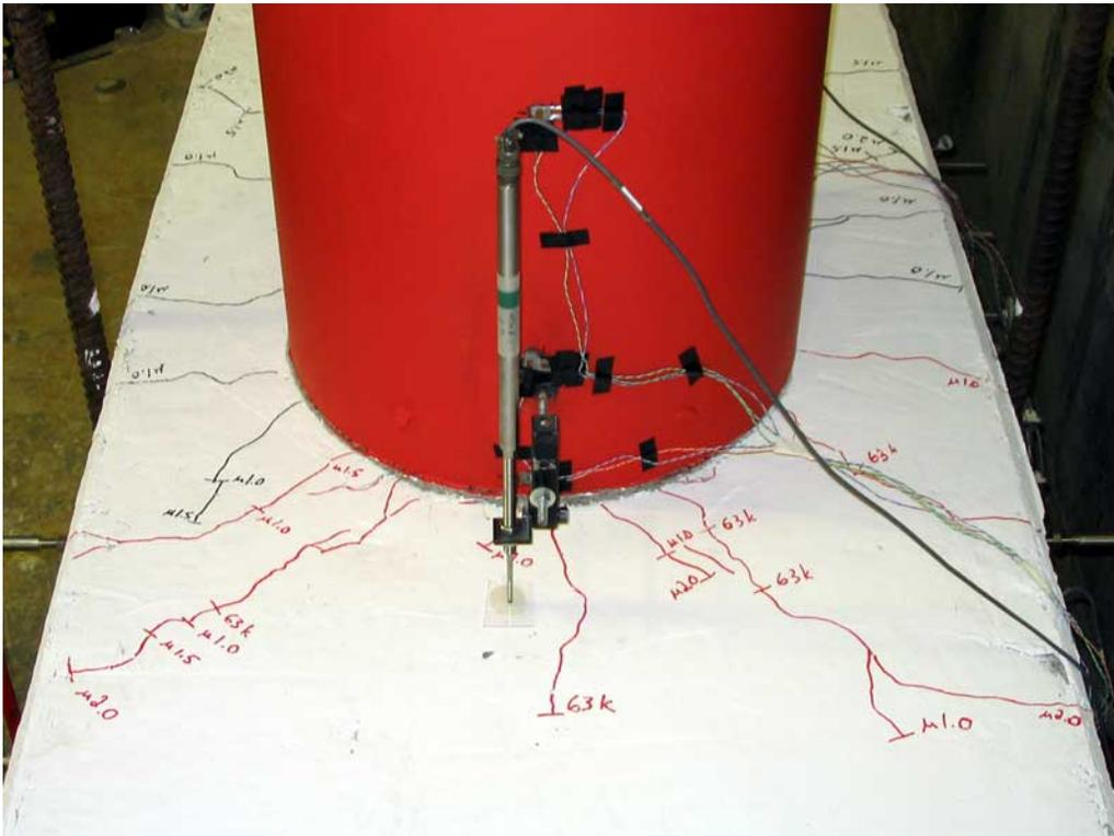
**Figure 0-7. Bent Cap Cracking at  $2.0 \mu\Delta$**
