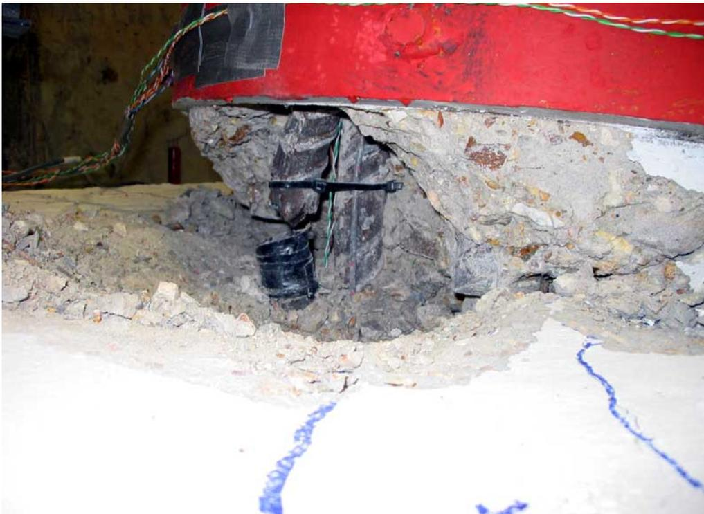
**Figure 0-18. Column Longitudinal Bar Fracture at  $8.0 \mu\Delta$**
