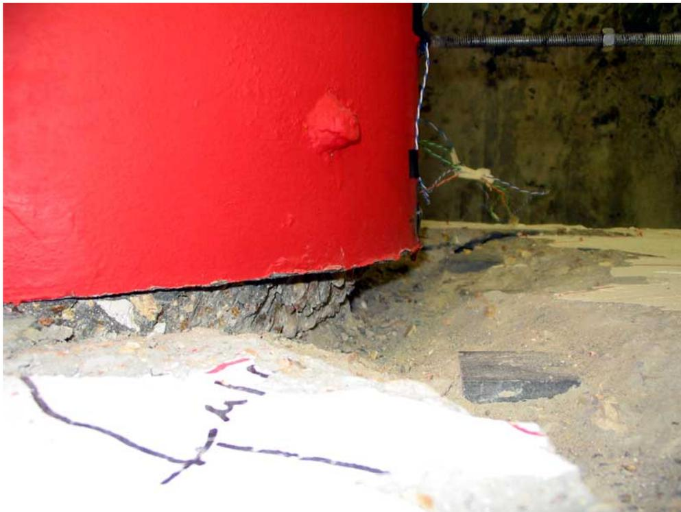
**Figure 0-17. Column Crushing Ultimate Damage**
