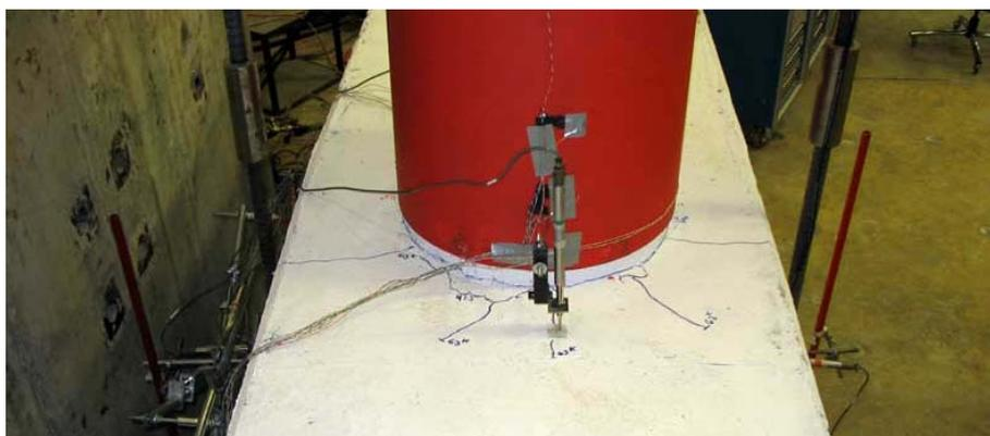
**Figure 0-1. Bent Cap Cracking at 1.00V<sub>y</sub>**
