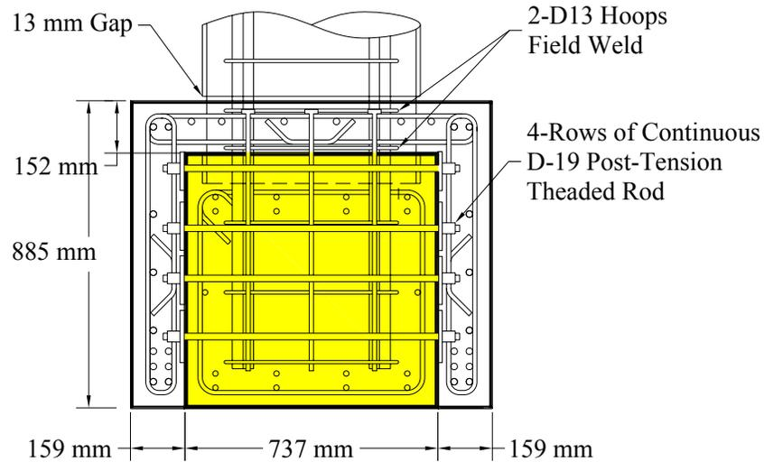
**Figure 0-1. Unit 3 Retrofit Cross-Section**
