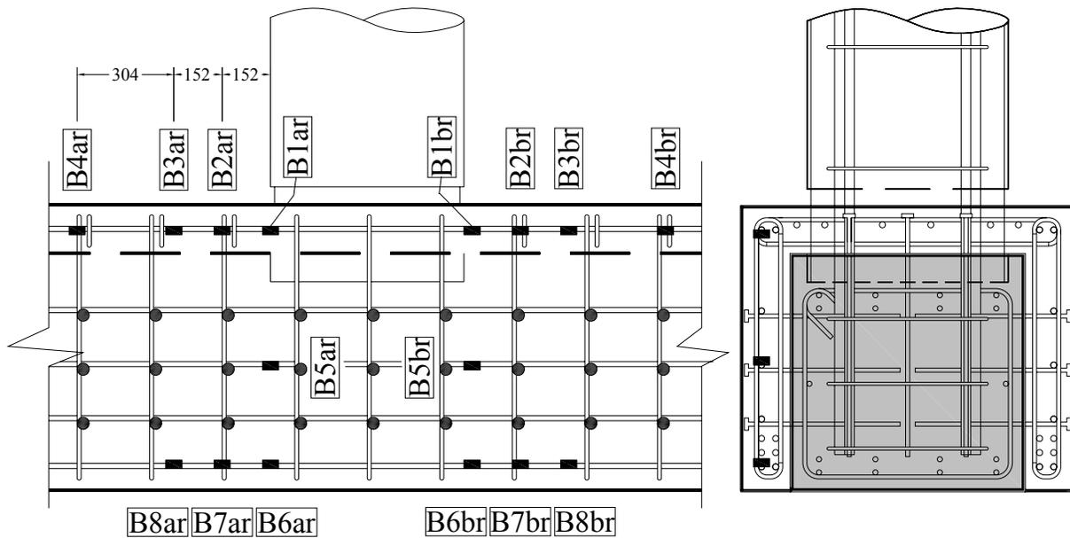
Figure 0-4. Retrofit Bent Cap Strain Gauges
