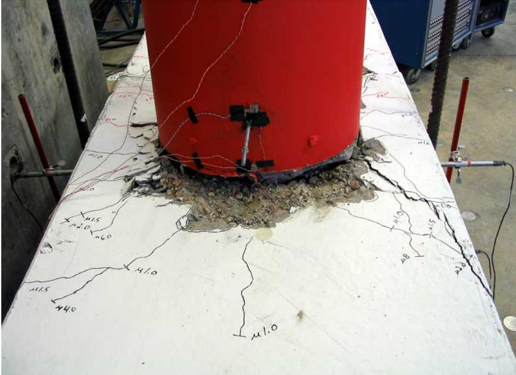
**Figure 0-14. Bent Cap Cracking – Side “B” at 8.0  $\mu\Delta$**
