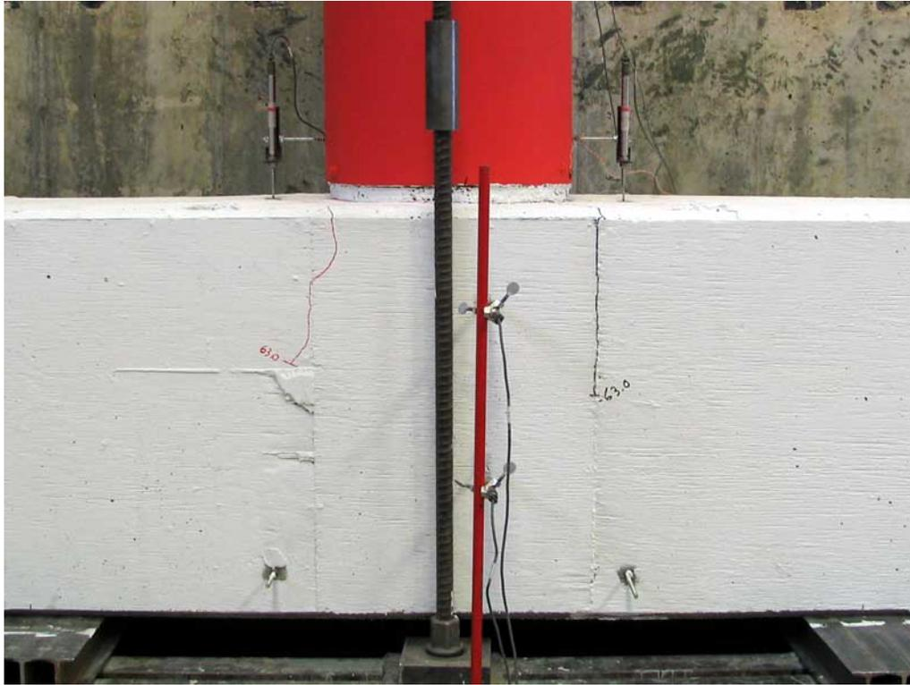
**Figure 0-4. Joint Cracking at 1.00V<sub>y</sub>**
