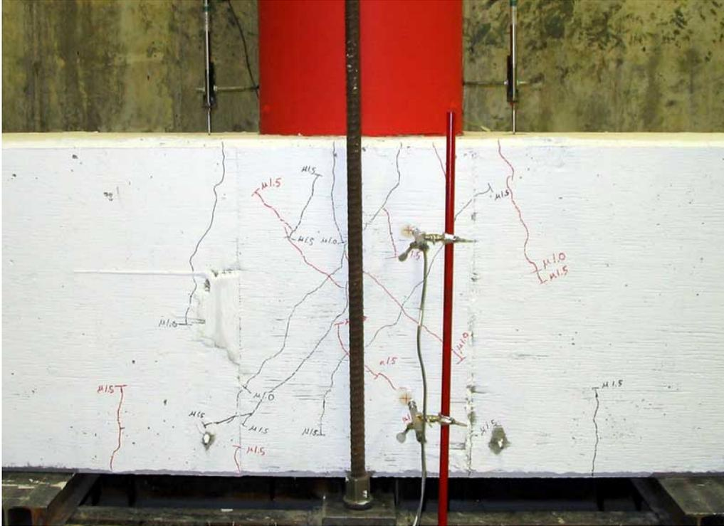
Figure 0-4. Joint Cracking at  $1.5 \mu\Delta$
