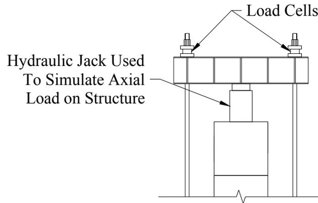
**Figure 0-8. Load Cells for Axial Load**
