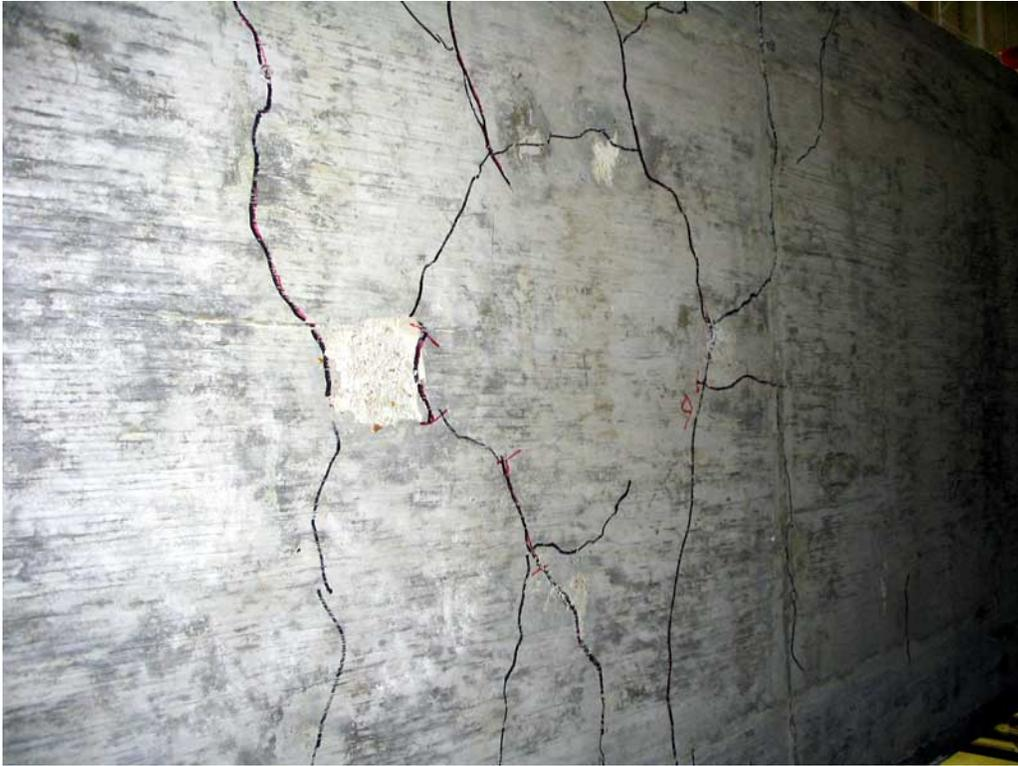
**Figure 0-15. Bottom Cracking at 8.0  $\mu\Delta$**
