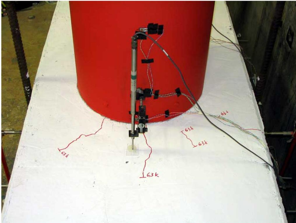
**Figure 0-1. Bent Cap Cracking at  $1.00V_y$**
