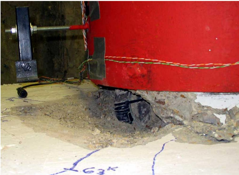
**Figure 0-16. Column Longitudinal Bar Buckling at 6.0  $\mu\Delta$**
