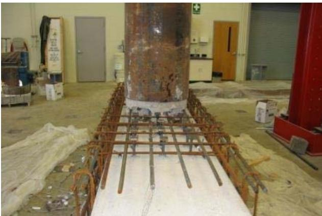
**Figure 0-22. Retrofit Section Reinforcing Cage**
