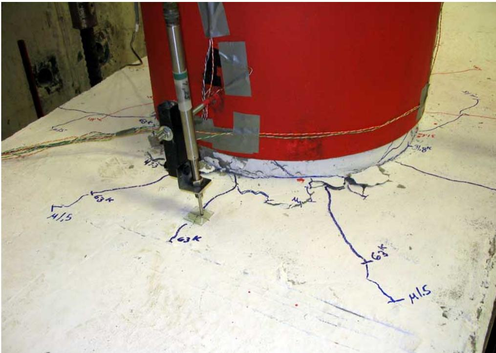
Figure 0-6. Bent Cap Cracking at  $1.5 \mu\Delta$
