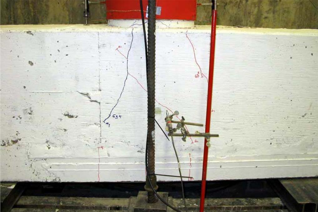
**Figure 0-3. Joint Cracking at 1.0  $\mu\Delta$**
