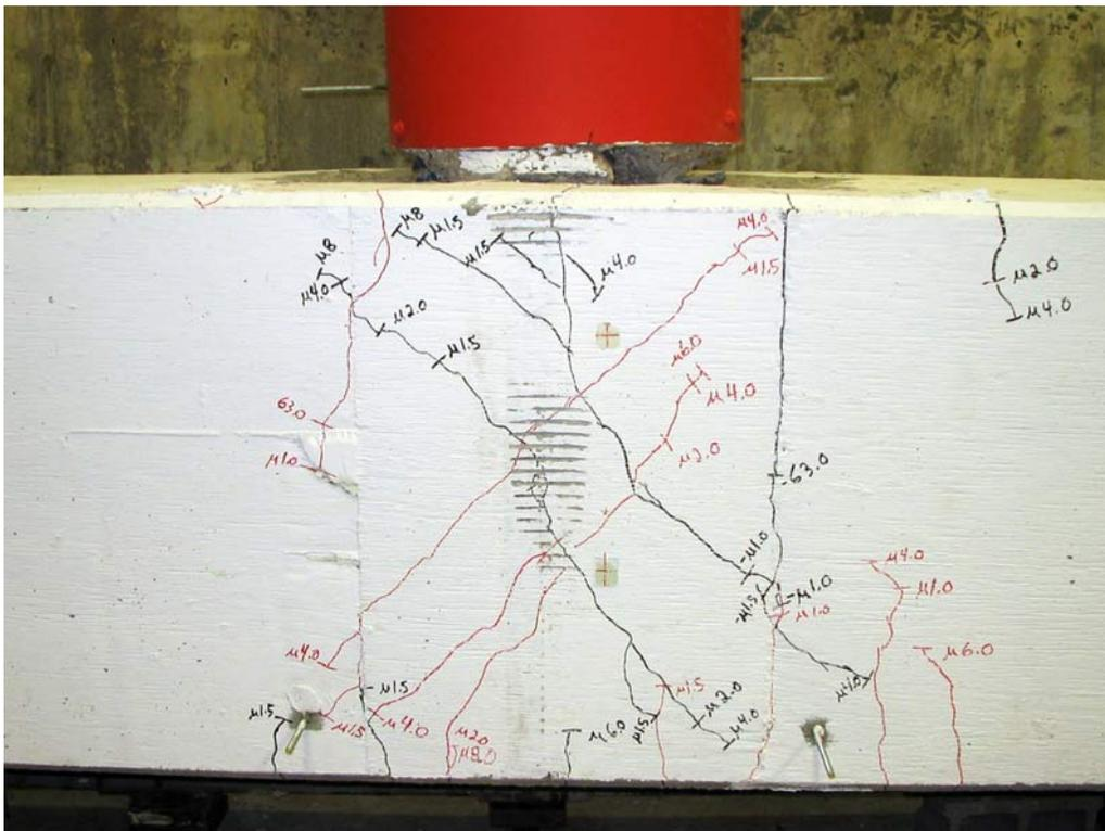
**Figure 0-22. Unit 2 Joint Shear Cracks**
