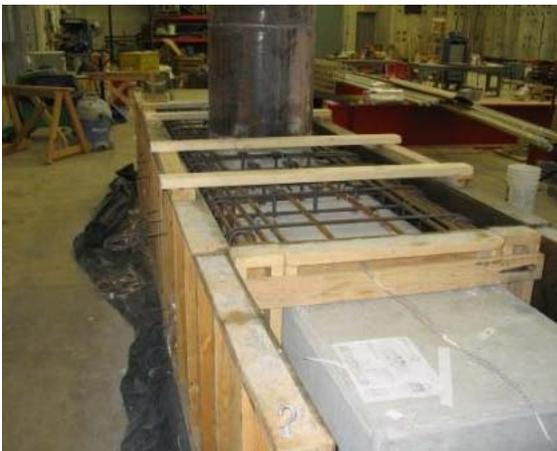
**Figure 0-9. Unit Before Casting of Upgrade Section**
