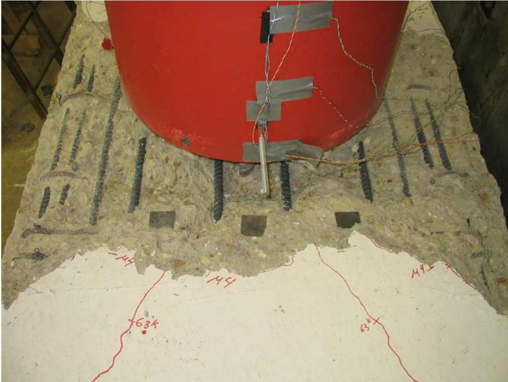
**Figure 0-21. Bent Cap Ultimate Damage**
