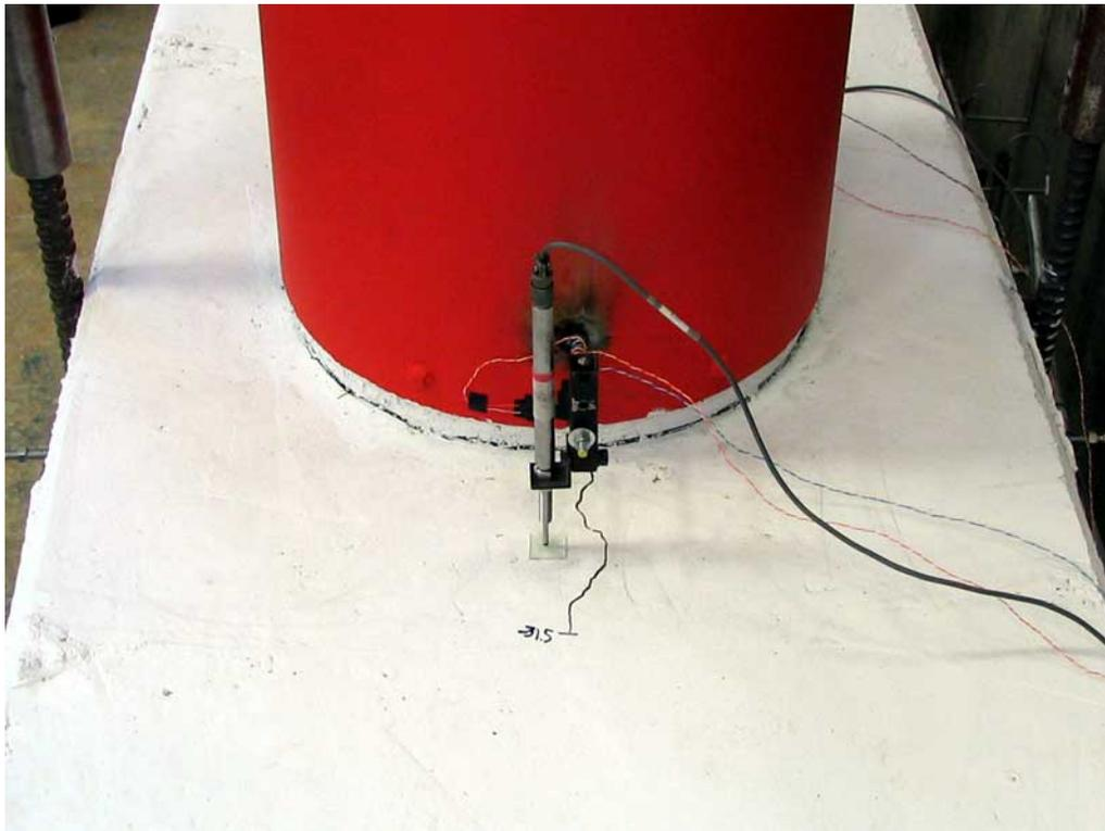
**Figure 0-1. Bent Cap Cracking at  $0.50V_y$**
