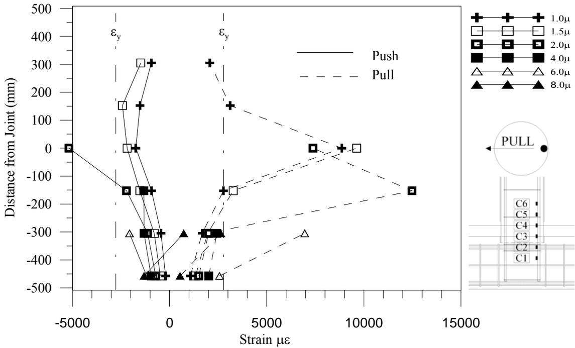
**Figure 0-27. Strain Gauge Profile – Side “A”**
