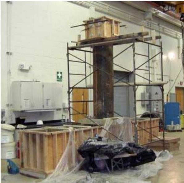
**Figure 0-18. Construction of the Load Stub**
