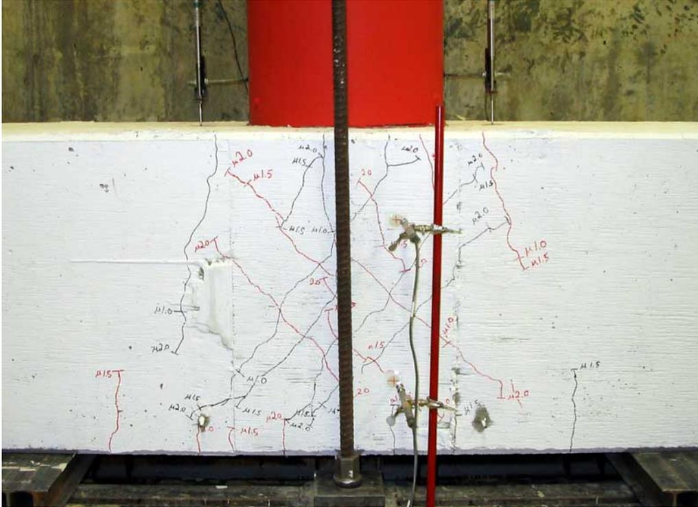
**Figure 0-6. Joint Cracking at  $2.0 \mu\Delta$**
