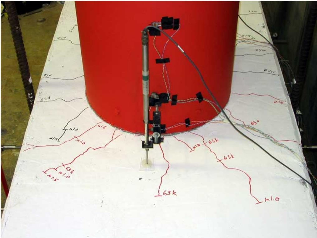
Figure 0-5. Bent Cap Cracking at  $1.5 \mu\Delta$
