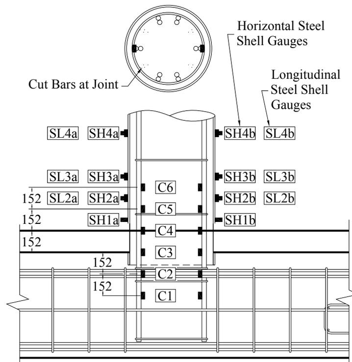
**Figure 0-1. Column Reinforcement and Steel Shell Strain Gauges**
