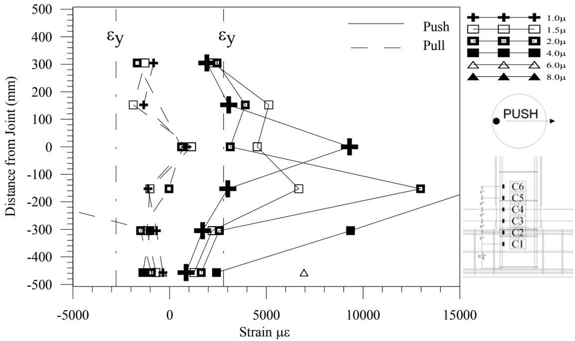
Figure 0-25. Strain Gauge Profile – Side “B”
