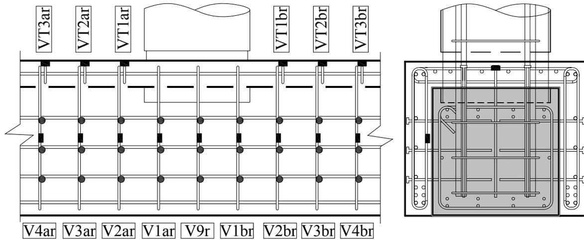
**Figure 0-5. Retrofit Bent Cap Shear Strain Gauges**
