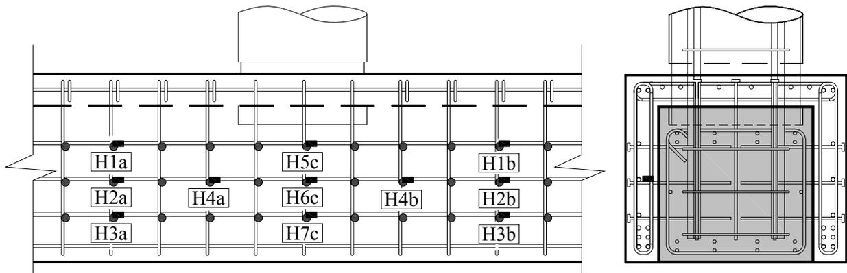
**Figure 0-6. Retrofit Transverse Headed Reinforcement Strain Gauges**
