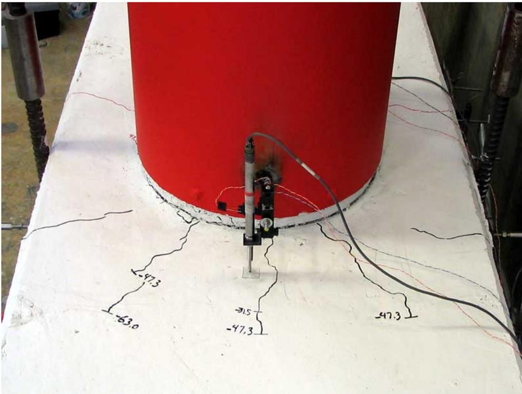
**Figure 0-3. Bent Cap Cracking at  $1.00V_y$**
