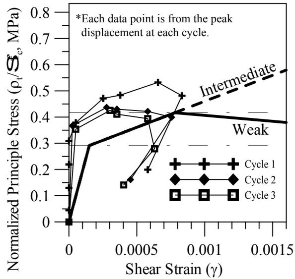
**Figure 0-34. Unit 2 Principle Tensile Stress vs. Joint Shear Strain**
