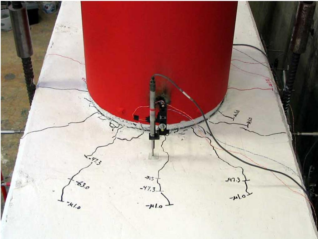
**Figure 0-6. Bent Cap Cracking at 1.0  $\mu\Delta$**
