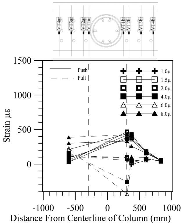
**Figure 0-32. Unit 3 Top Transverse Reinforcement Strain Profile**
