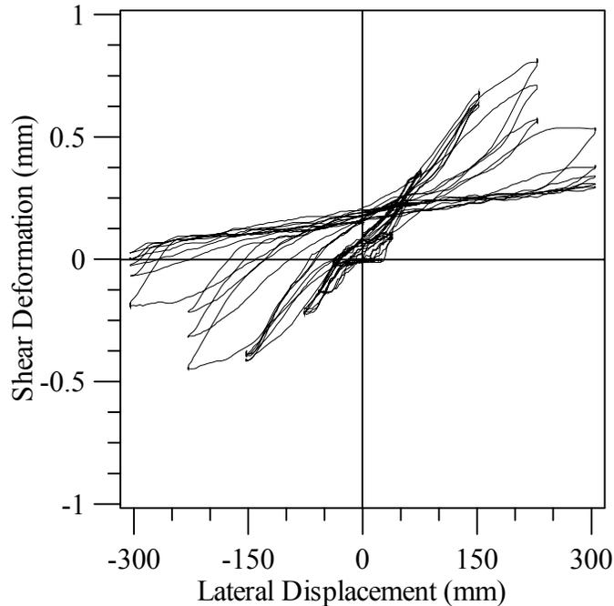
**Figure 0-30. Unit 3 Joint Shear Deformation**
