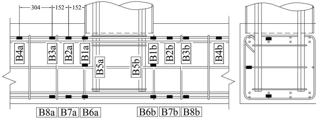
Figure 0-2. As-Built Bent Cap Strain Gauges
