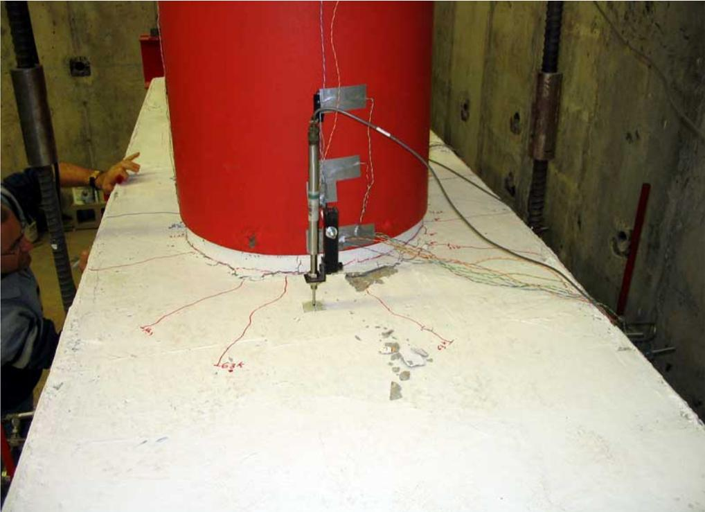
**Figure 0-4. Bent Cap Cracking at 1.0  $\mu\Delta$**
