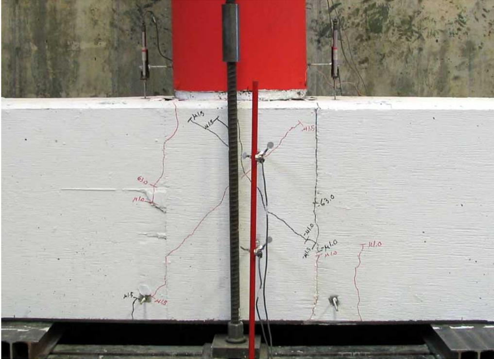
Figure 0-7. Joint Cracking at  $1.5 \mu\Delta$
