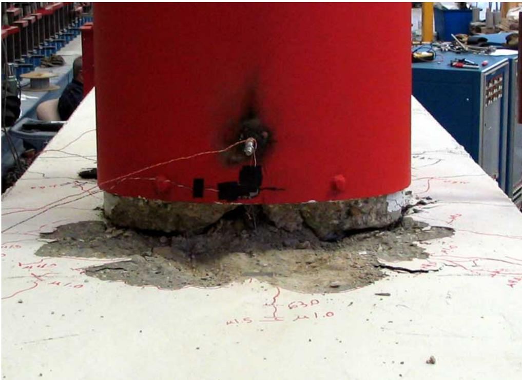
**Figure 0-14. Bent Cap Cracking at 6.0  $\mu\Delta$**
