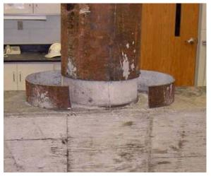
Figure 0-20. Cutting Steel Shell Casing
