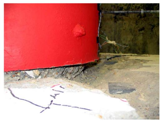
Figure 0-17. Column Crushing Ultimate Damage
