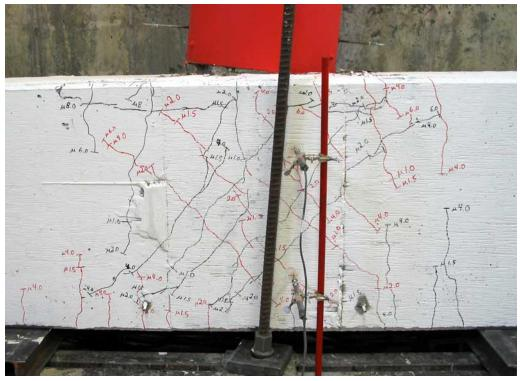
Figure 0-12. Joint Cracking at 8.0  $\mu_{\Delta}$
