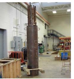
Figure 0-15. Colum Reinforcing Cage
