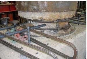
Figure 0-4. Detail at Bent Cap Interface
