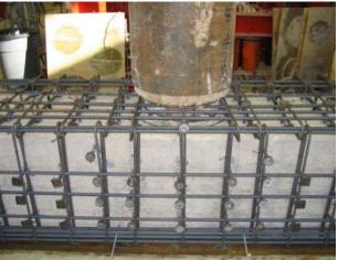
Figure 0-6. Bent Cap Retrofit Section
