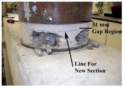
Figure 0-2. Cut Longitudinal Reinforcement
