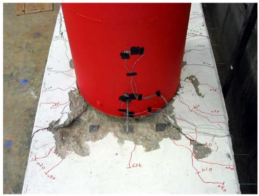
Figure 0-16. Bent Cap Cracking Ultimate Damage
