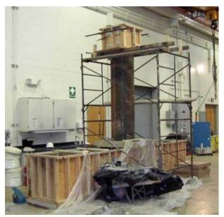
Figure 0-18. Construction of the Load Stub
