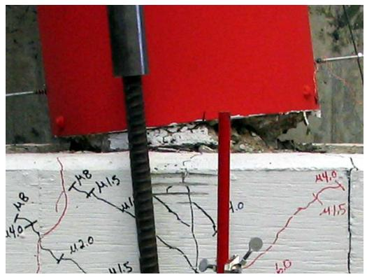
Figure 0-17. Column Crushing at 8.0  $\mu_{\Delta}$
