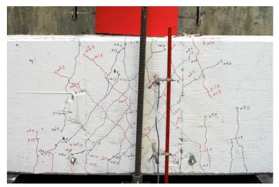
Figure 0-20. Unit 3 Joint Shear Cracks
