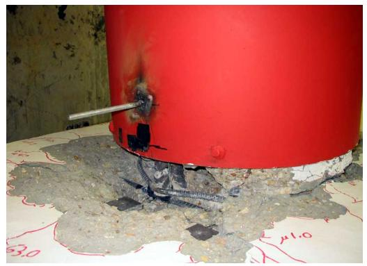
Figure 0-19. Hoop Buckling Side "A"
