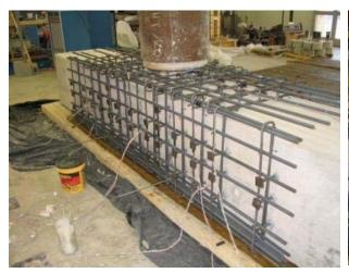
Figure 0-5. Bent Cap Retrofit Section
