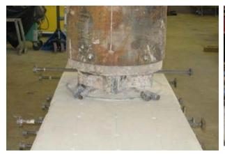
Figure 0-3. Detail at Bent Cap Interface
