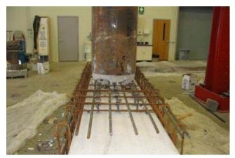
Figure 0-22. Retrofit Section Reinforcing Cage
