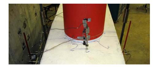
Figure 0-1. Bent Cap Cracking at 1.00Vy
