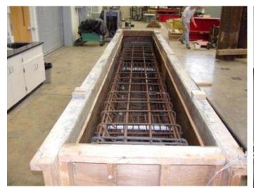
Figure 0-14. Bent Cap Inside Form Work
