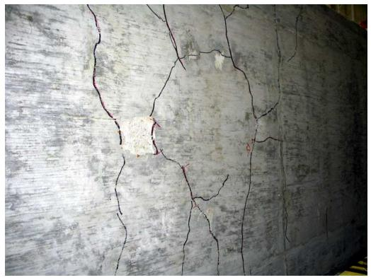
Figure 0-15. Bottom Cracking at 8.0  $\mu_{\Delta}$
