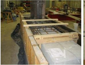
Figure 0-9. Unit Before Casting of Upgrade Section
