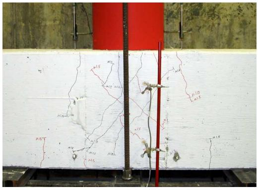
Figure 0-4. Joint Cracking at 1.5  $\mu_{\Delta}$
