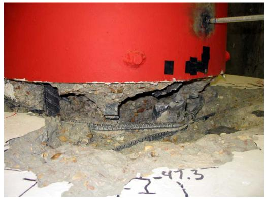
Figure 0-20. Hoop Buckling Side "B"
