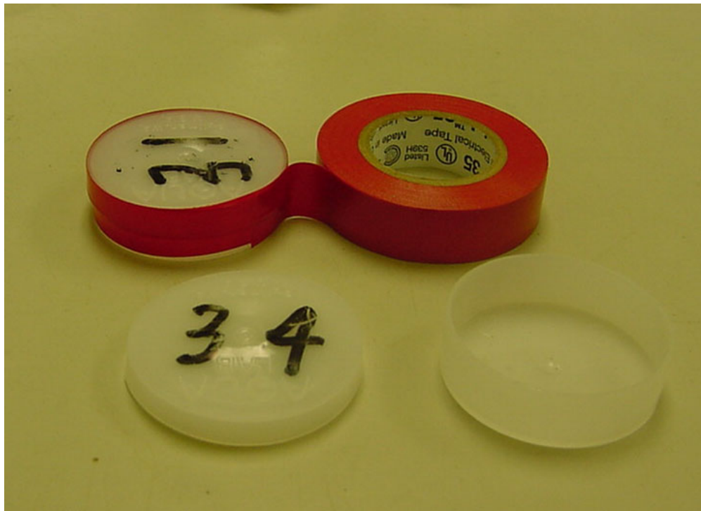
Figure 14. WP4 Cup and Lid and Sealing of Cup for Equilibration
