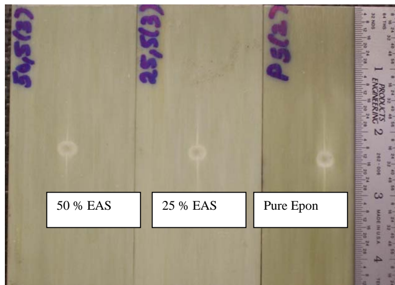
Figure 2. Front surface of composite samples impacted at 5 Joules
