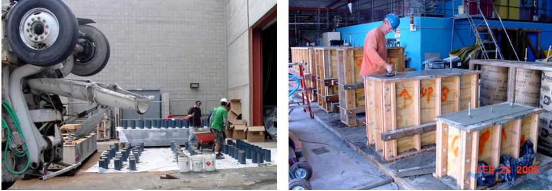
Figure 6-10 Casting of Columns and Cylinders at UCSD
