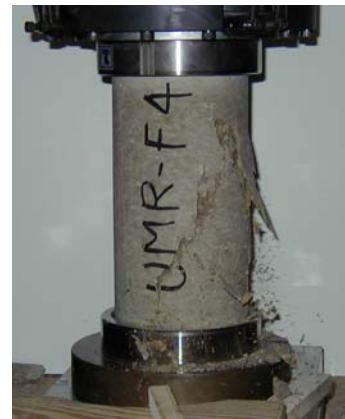
(b) Compression Test
