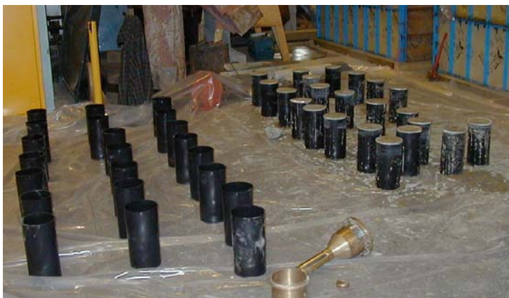
(a) Casting of Standard Concrete Cylinders
