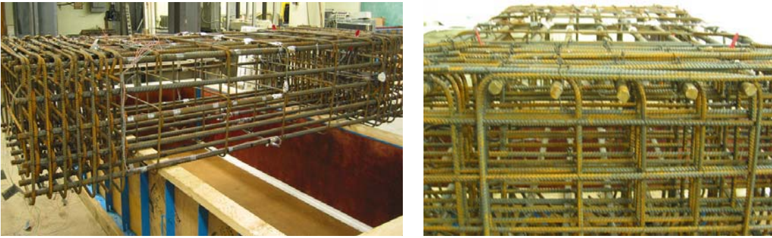
Figure 6-11 Layout of Steel Reinforcement; NIST Specimens
