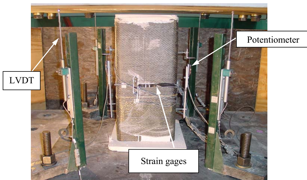
Figure 6-19 - Specimen E2 Setup at UCSD
