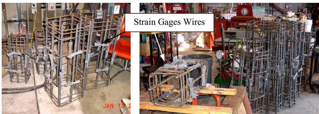
Figure 6-9 Steel Reinforcement for UCSD Specimens
