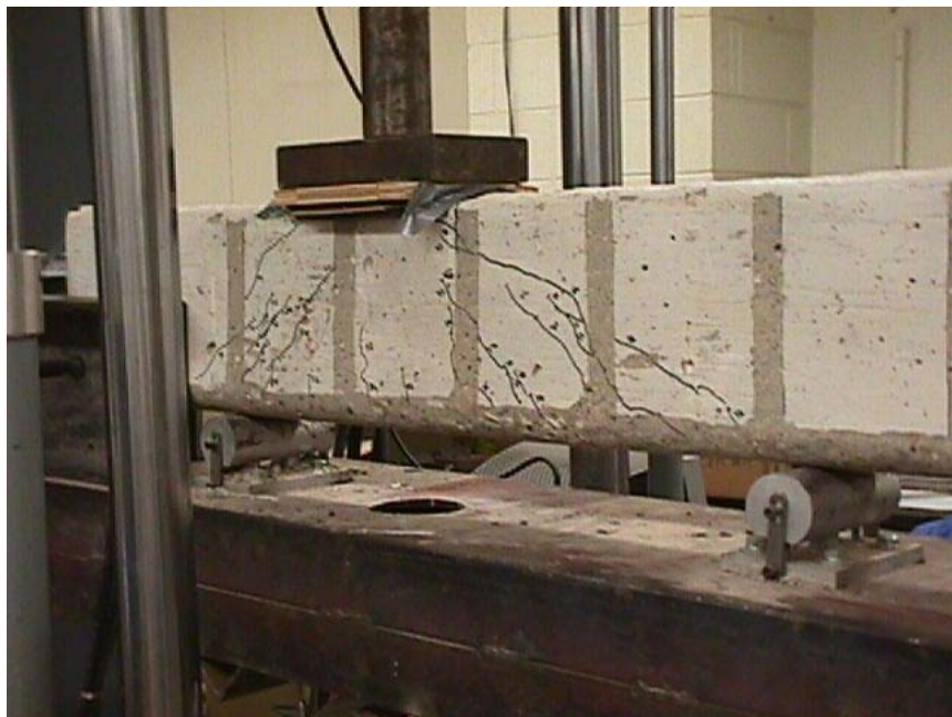
Fig. 4 – Crack patterns in Beam 1
