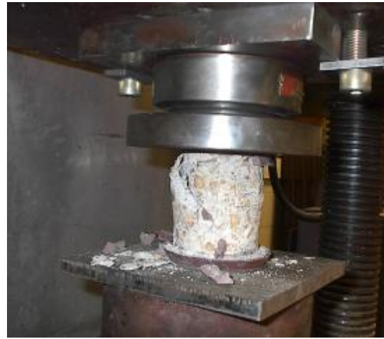
b) Compression Tests
