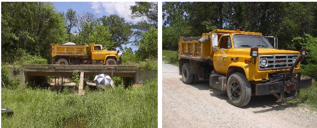
Figure 5.1. Load Tests after Strengthening on Bridge No. 3855006
