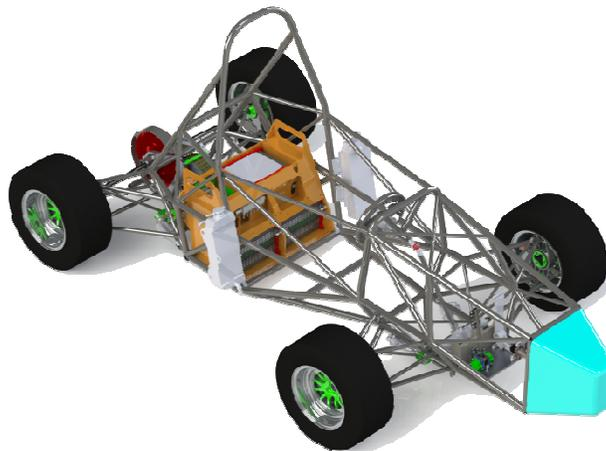
**Figure 1 - Solid Model Rendering of Vehicle**
